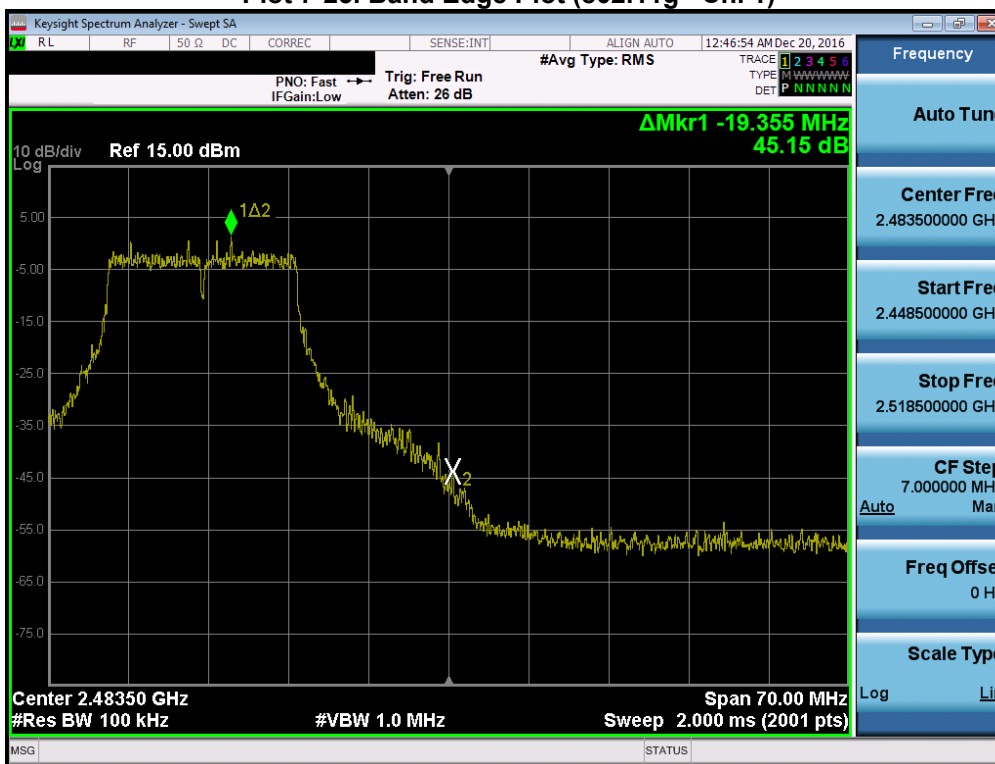
Plot 7-24. Band Edge Plot (802.11g – Ch. 11)
