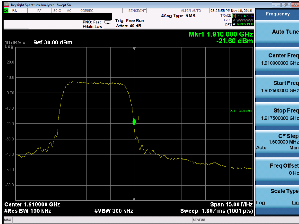
Plot 7-53. Band Edge Plot (PCS WCDMA Mode – Ch. 9538, Antenna A)
