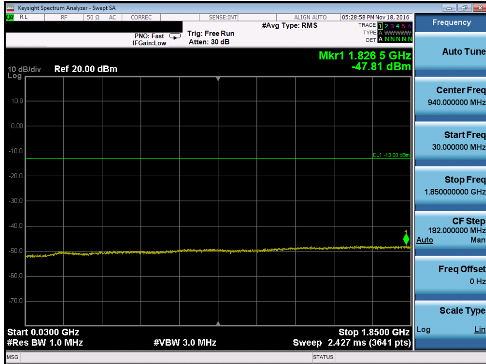
Plot 7-37. Conducted Spurious Plot (PCS WCDMA Mode – Ch. 9400, Antenna A)
