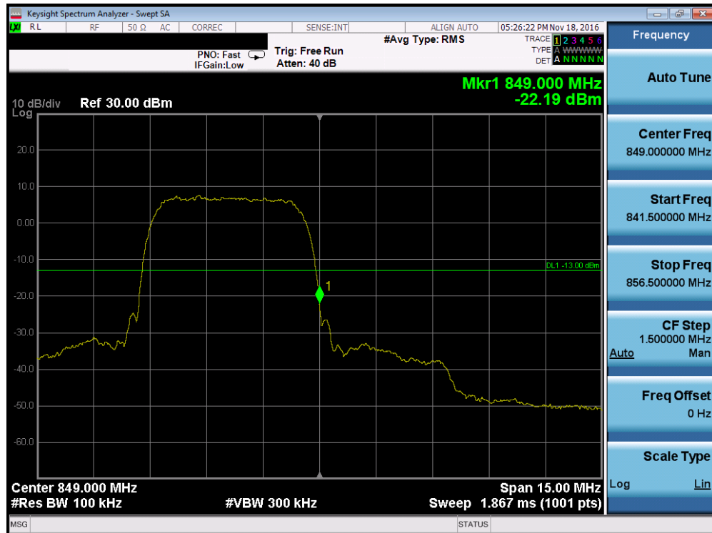
Plot 7-50. Band Edge Plot (Cellular WCDMA Mode – Ch. 4233, Antenna B)
