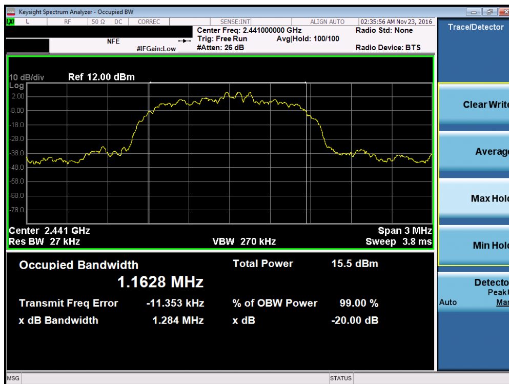
Plot 7-5. 20dB Bandwidth Plot (Bluetooth, 2Mbps – Ch. 39)
