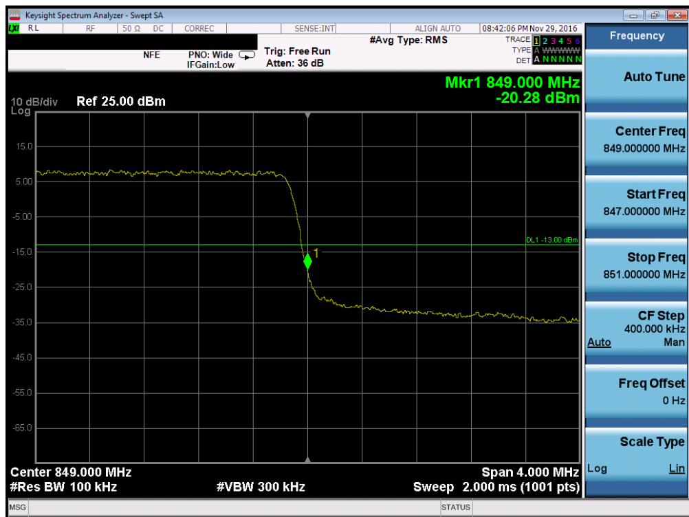
Plot 7-46. Upper Band Edge Plot (Band 5 - 3.0MHz QPSK - RB Size 15, Antenna C)
