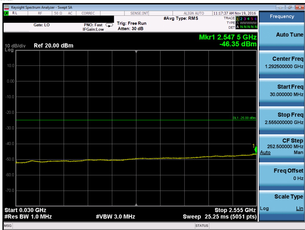
Plot 7-37. Conducted Spurious Plot (Band 41 – 5.0MHz QPSK – RB Size 1, RB Offset 0 – Mid Channel, Antenna A)
