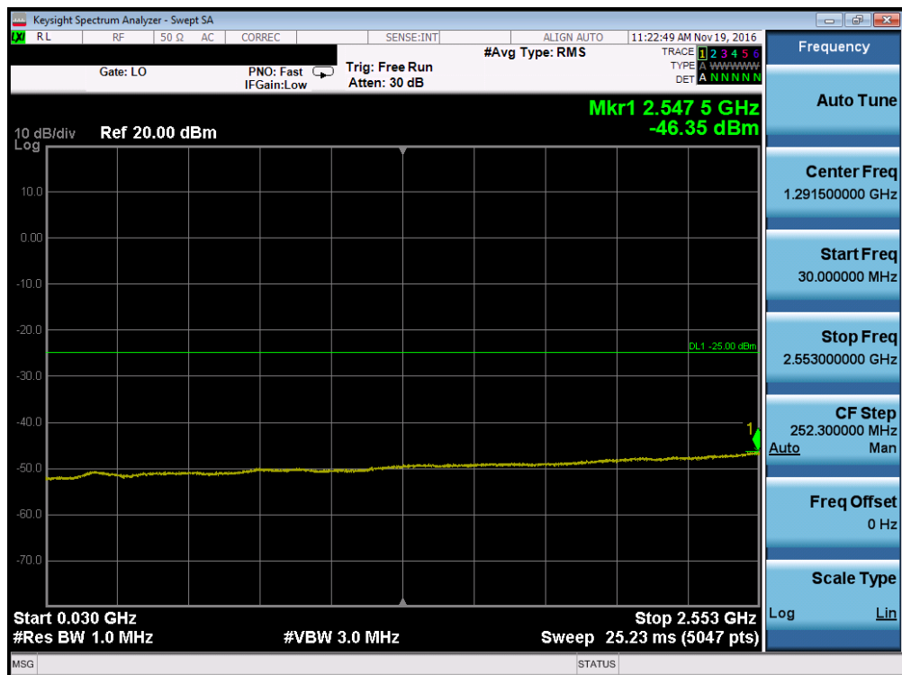
Plot 7-34. Conducted Spurious Plot (Band 41 – 5.0MHz QPSK – RB Size 1, RB Offset 0 – Low Channel, Antenna A)
