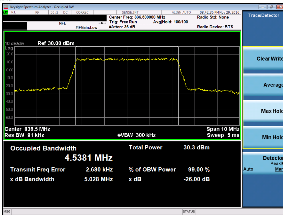
Plot 7-7. Occupied Bandwidth Plot (Band 5 – 5.0MHz QPSK – RB Size 25, Antenna C)
