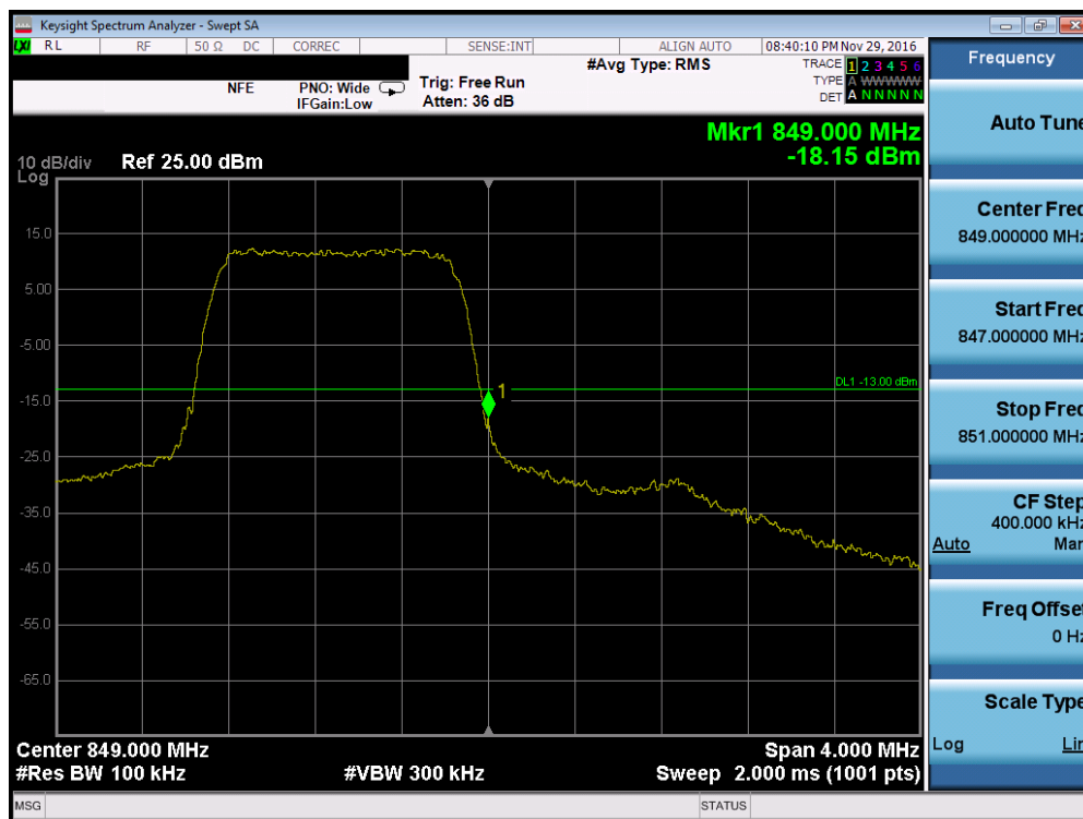
Plot 7-44. Upper Band Edge Plot (Band 5 – 1.4MHz QPSK – RB Size 6, Antenna C)
