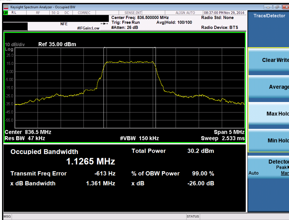
Plot 7-1. Occupied Bandwidth Plot (Band 5 – 1.4MHz QPSK – RB Size 6, Antenna C)
