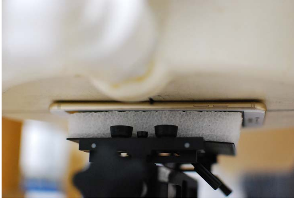
SAR Test Setup Photo 11 – Back at 0.0 cm
