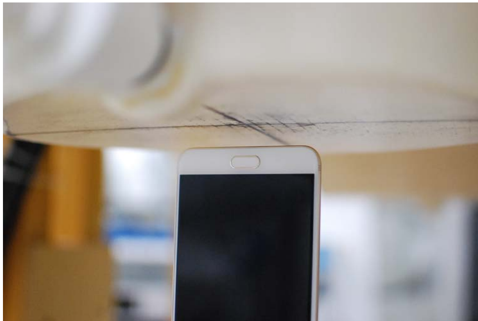
SAR Test Setup Photo 8 – Bottom at 1.0 cm
