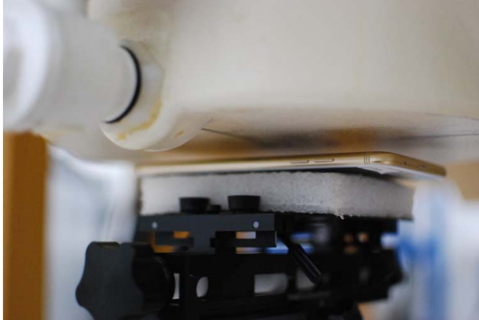
SAR Test Setup Photo 5 – Back at 1.0 cm
