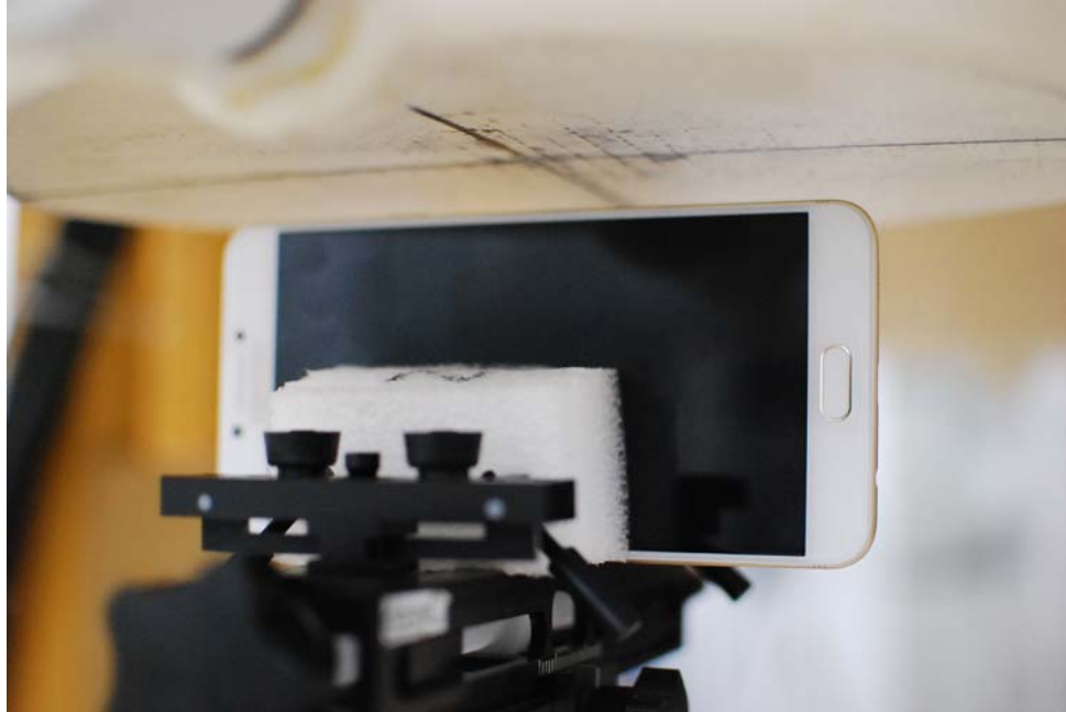
SAR Test Setup Photo 9 – Right at 1.0 cm
