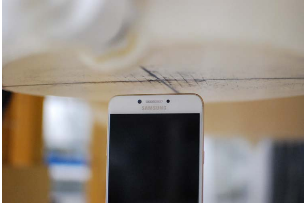
SAR Test Setup Photo 7 – Top at 1.0 cm
