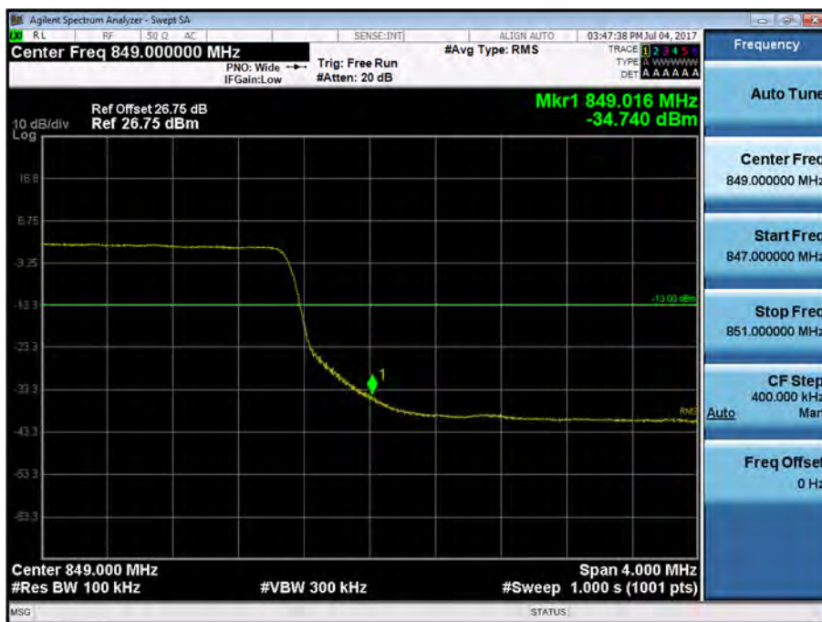
BAND 5. Upper Band Edge Plot (10M BW Ch.20600 QPSK_RB50_Offset 0)
