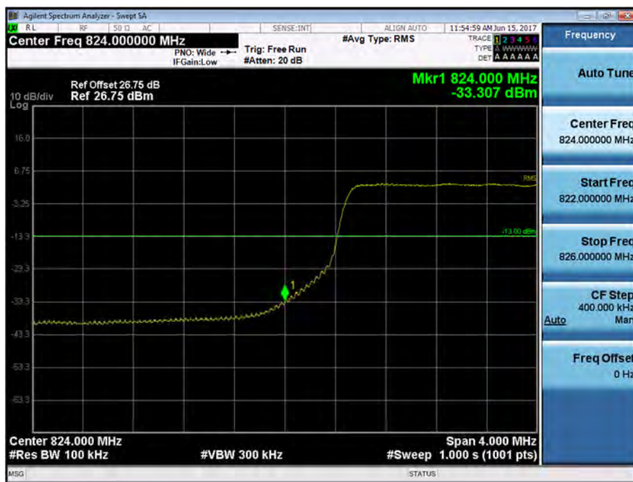
BAND 5. Lower Band Edge Plot (10M BW Ch.20450 QPSK_RB50_Offset 0)
