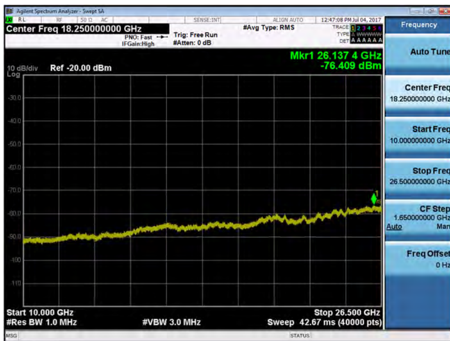
BAND7. Conducted Spurious Plot 2 (10MHz Ch.20800 QPSK RB 1, Offset 0)
