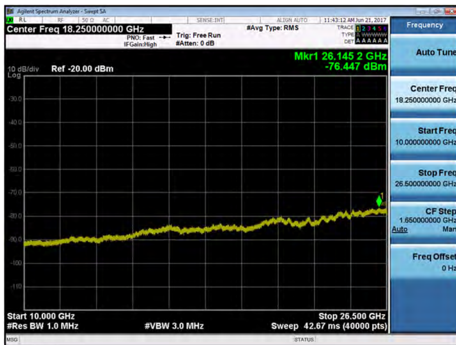
BAND7. Conducted Spurious Plot 2 (15MHz Ch.21375 QPSK RB 1, Offset 0)
