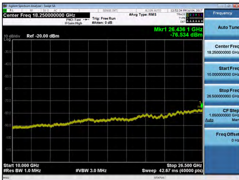
BAND7. Conducted Spurious Plot 2 (15MHz Ch.20825 QPSK RB 1, Offset 0)
