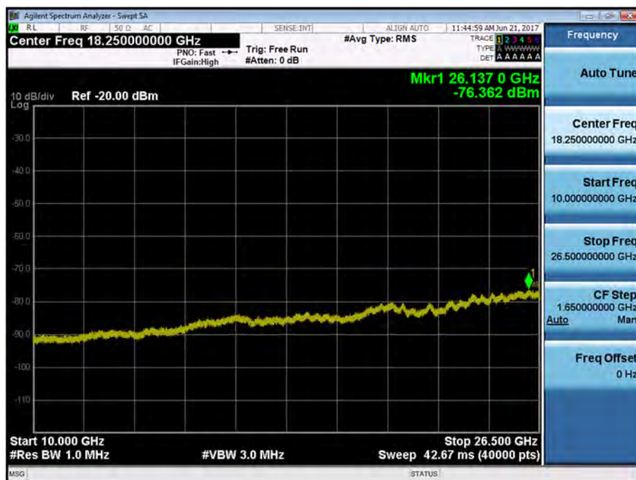
BAND7. Conducted Spurious Plot 2 (20MHz Ch.20850 QPSK RB 1, Offset 0)
