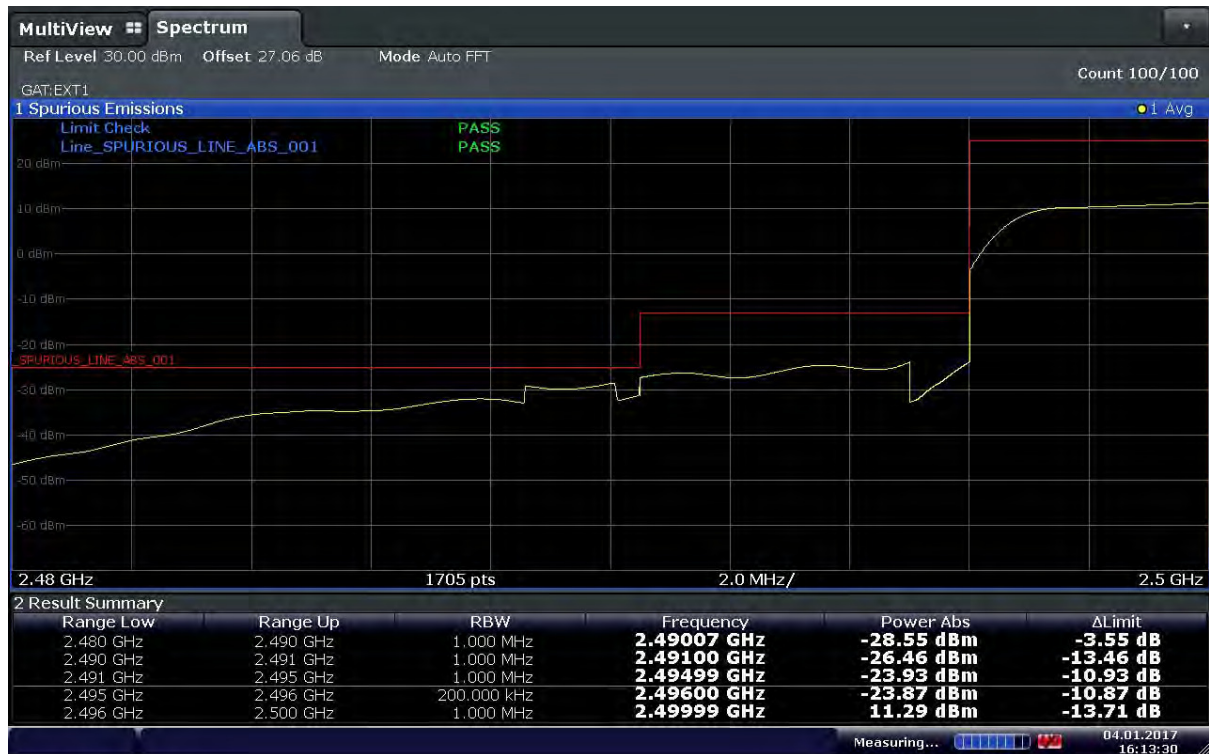
Plot 6-49. Lower Band Edge Plot (Band41 – 15MHz – QPSK – RB Size 75 – Ch.39725)
