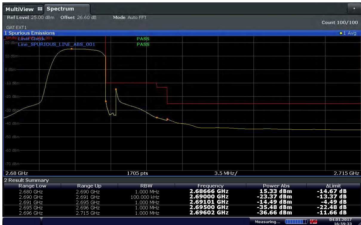
Plot 6-46. Upper Band Edge Plot (Band41 – 5MHz – QPSK – RB Size 25 – Ch.41565)
