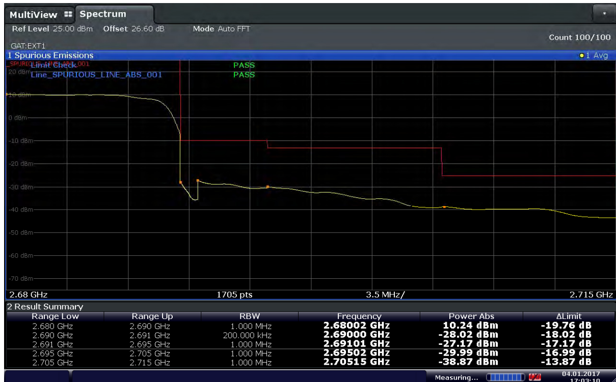
Plot 6-50. Upper Band Edge Plot (Band41 – 15MHz – QPSK – RB Size 75 – Ch.41515)
