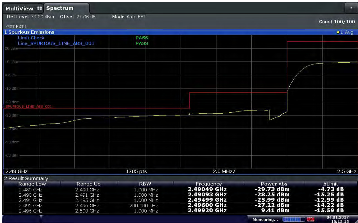
Plot 6-51. Lower Band Edge Plot (Band41 – 20MHz – QPSK – RB Size 100 – Ch.39750)
