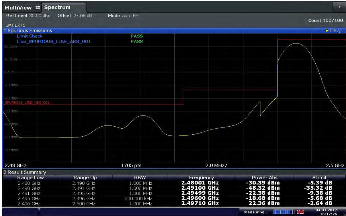
Plot 6-53. Lower Band Edge Plot (Band41 – 20MHz – QPSK – RB Size 1 – RB Offset 0 – Ch.39750)
