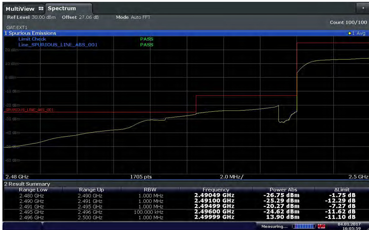
Plot 6-47. Lower Band Edge Plot (Band41 – 10MHz – QPSK – RB Size 50 – Ch.39700)
