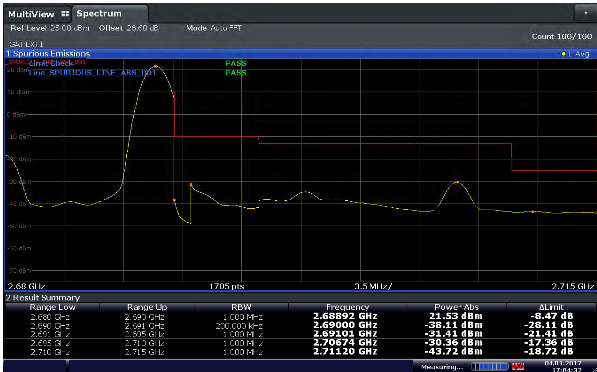
Plot 6-54. Upper Band Edge Plot (Band41 – 20MHz – QPSK – RB Size 1 – RB Offset 99 – Ch.41490)
