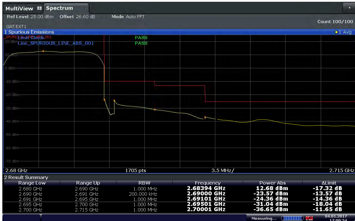
Plot 6-48. Upper Band Edge Plot (Band41 – 10MHz – QPSK – RB Size 50 – Ch.41540)
