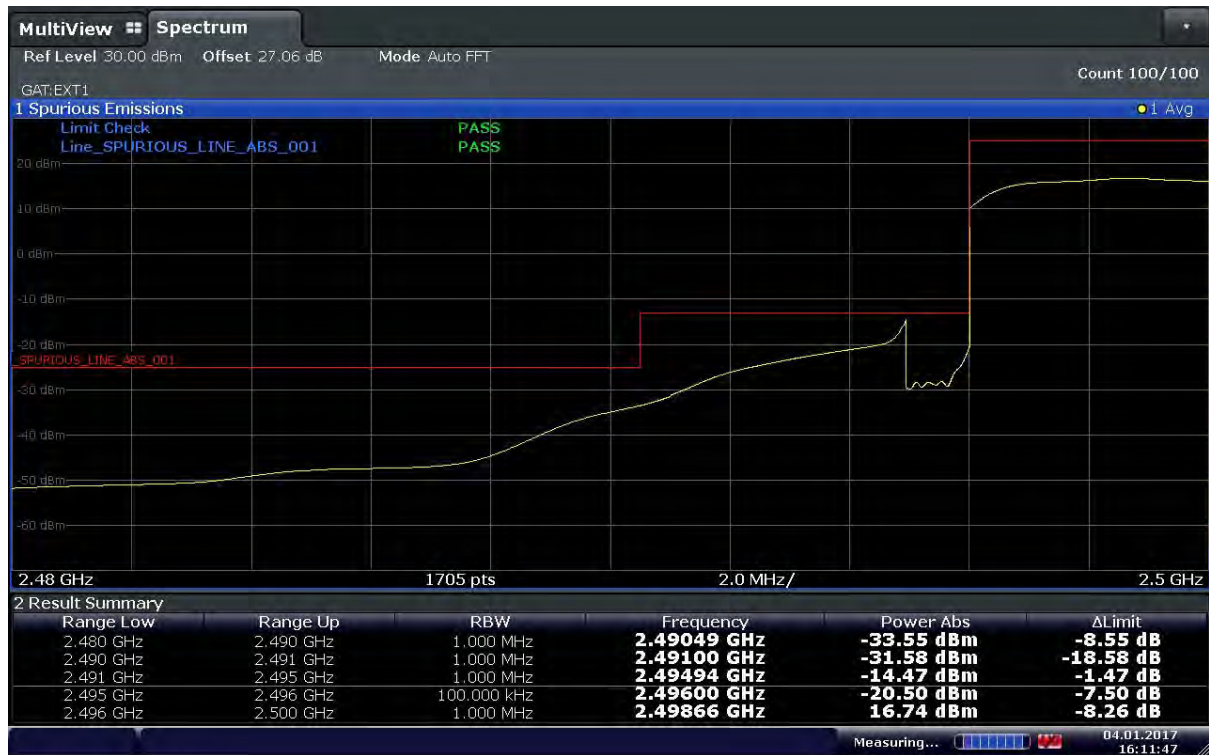
Plot 6-45. Lower Band Edge Plot (Band41 – 5MHz – QPSK – RB Size 25 – Ch.39675)
