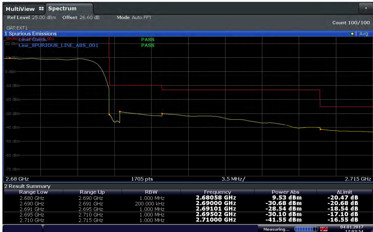
Plot 6-52. Upper Band Edge Plot (Band41 – 20MHz – QPSK – RB Size 100 – Ch.41490)
