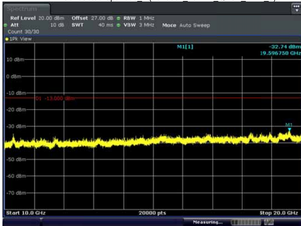
BAND 2. Conducted Spurious_2 (19100ch_20MHz_QPSK_RB 1_0)
