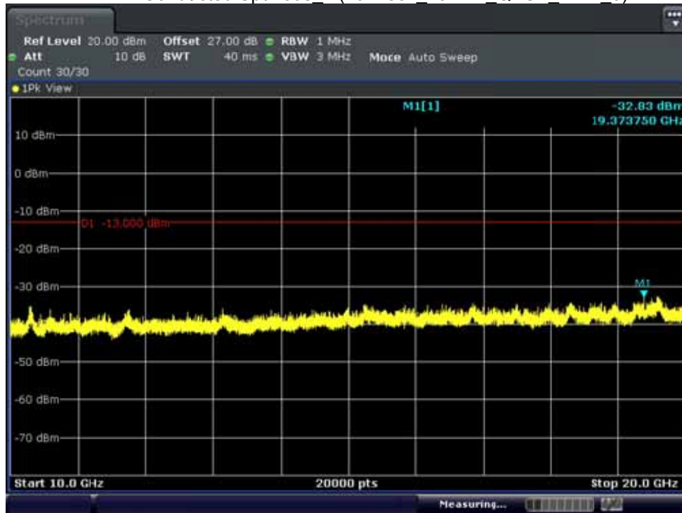
BAND 2. Conducted Spurious_2 (19125ch_15MHz_QPSK_RB 1_0)
