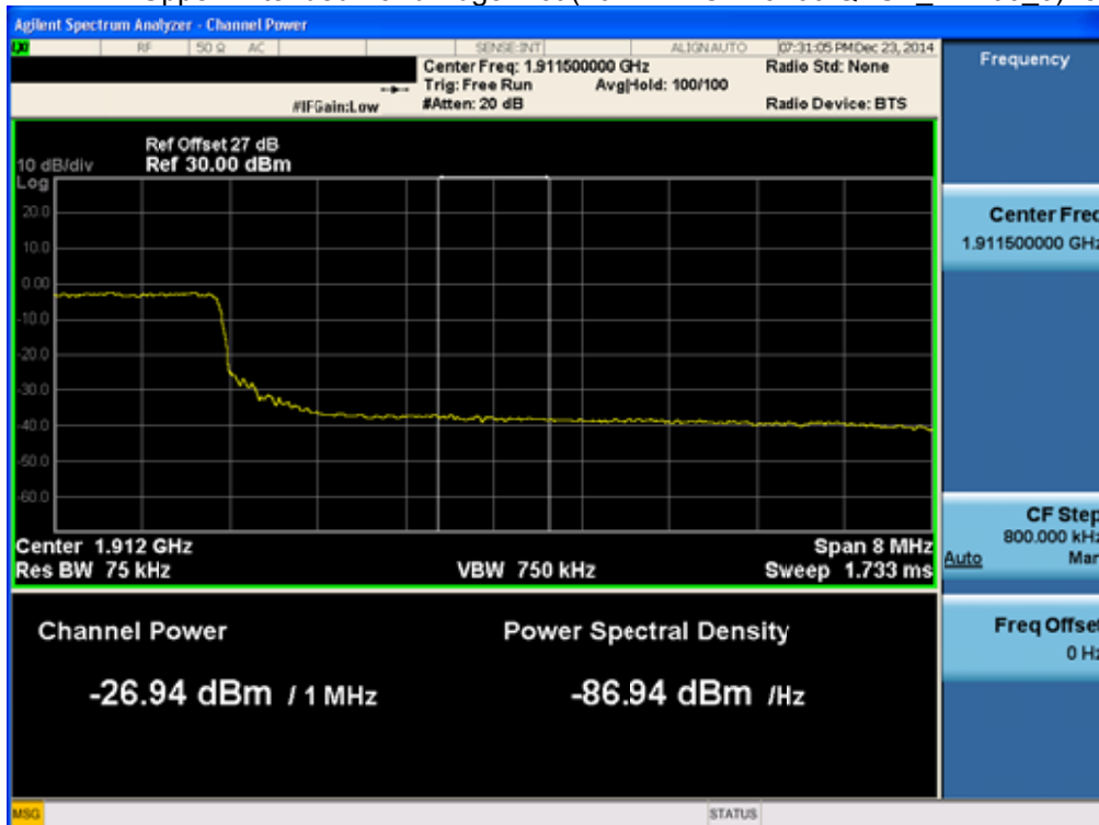
BAND 2. Upper Extended Band Edge Plot (20M BW Ch.19100 QPSK_RB100_0) -3
