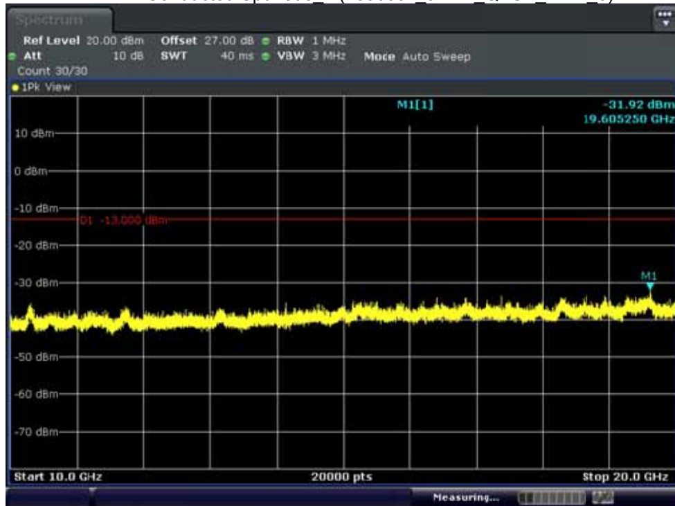
BAND 2. Conducted Spurious_2 (18900ch_5MHz_QPSK_RB 1_0)
