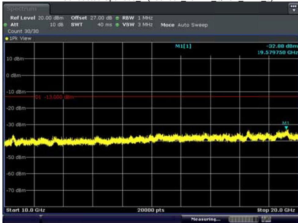
BAND 2. Conducted Spurious_2 (18675ch_15MHz_QPSK_RB 1_0)
