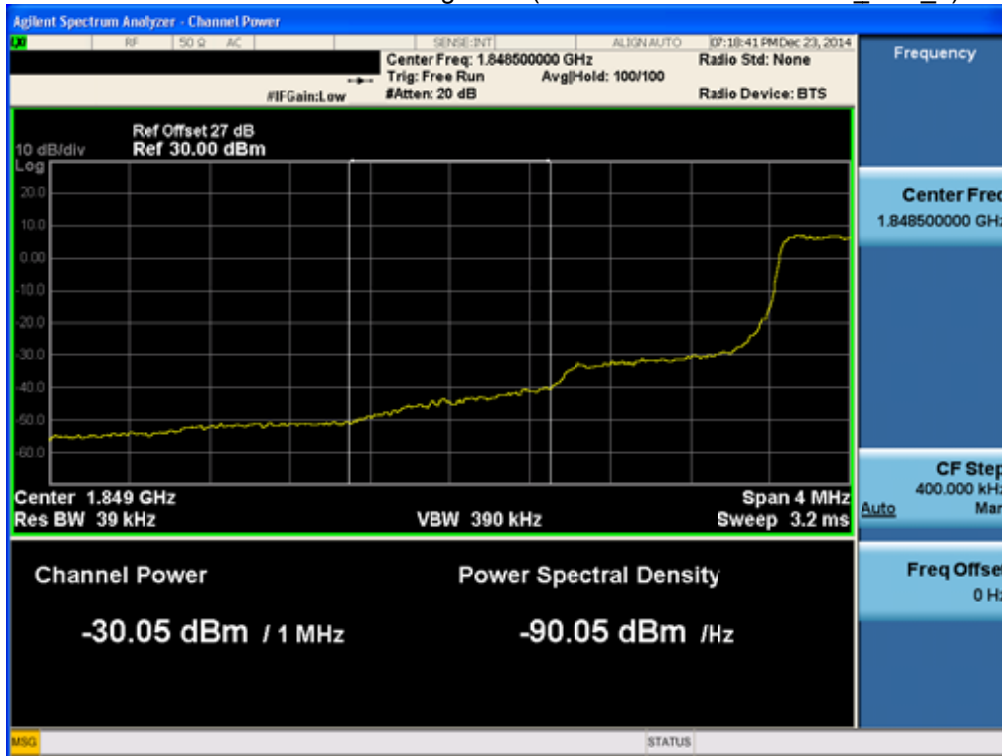
BAND 2. Lower Band Edge Plot (3M BW Ch.18615 QPSK_RB1_Offset 0) -1
