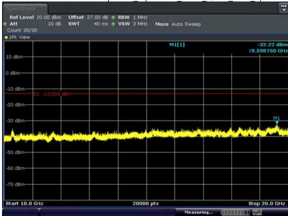
BAND 2. Conducted Spurious_2 (18900ch_3MHz_QPSK_RB 1_0)
