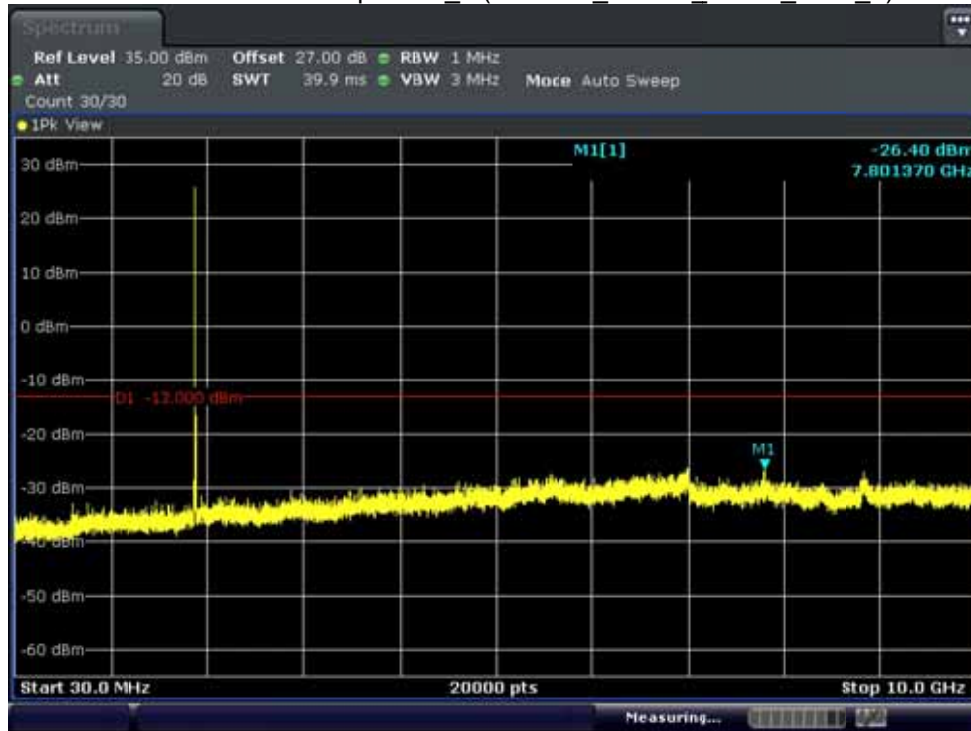
BAND 2. Conducted Spurious_1 (19125ch_15MHz_QPSK_RB 1_0)
