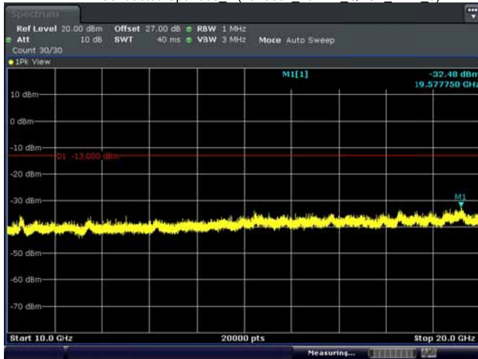
BAND 2. Conducted Spurious_2 (19150ch_10MHz_QPSK_RB 1_0)
