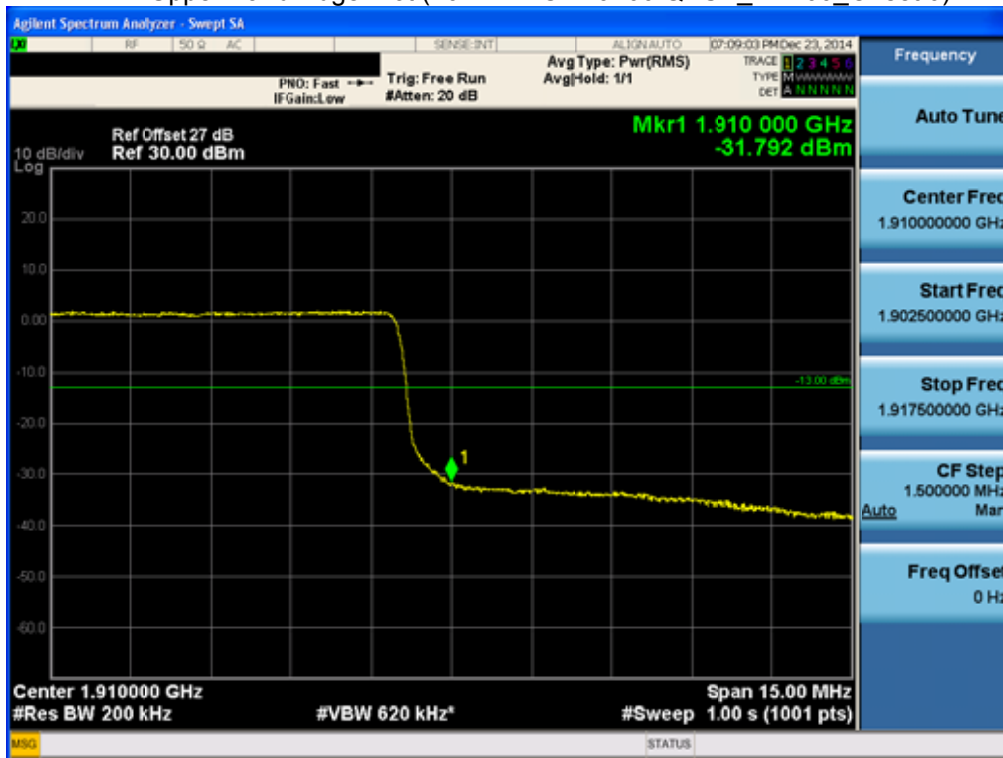
BAND 2. Upper Extended Band Edge Plot (20M BW Ch.19100 QPSK_RB100_0) -3
