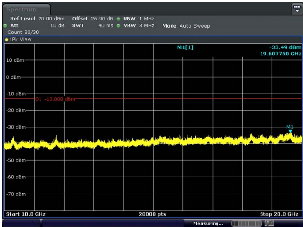
BAND 4. Conducted Spurious Plot_2 (20175ch_5MHz_QPSK_RB 1_0)
