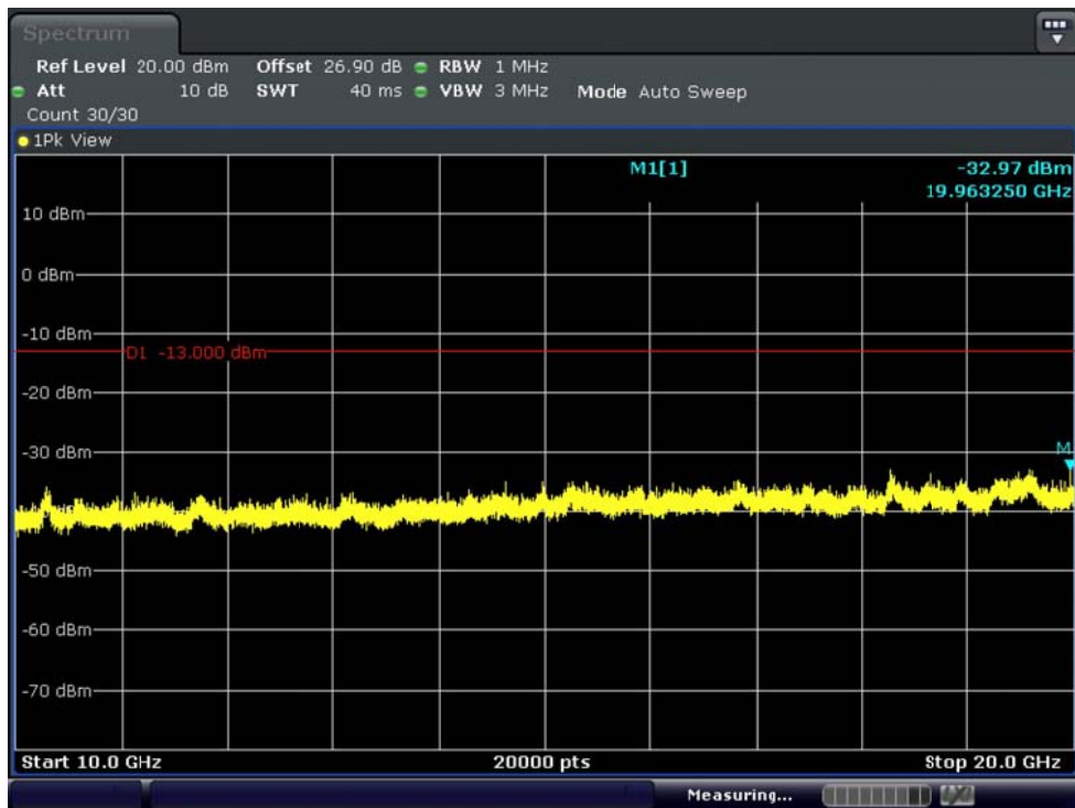
BAND 4. Conducted Spurious Plot_2 (19957ch_1.4MHz_QPSK_RB 1_0)
