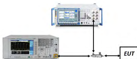
Figure 7-4. Test Instrument & Measurement Setup
