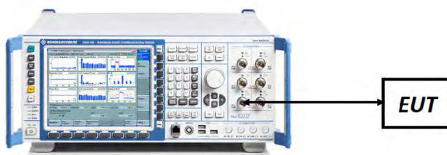
Figure 7-8. ERP/EIRP Measurement Setup
