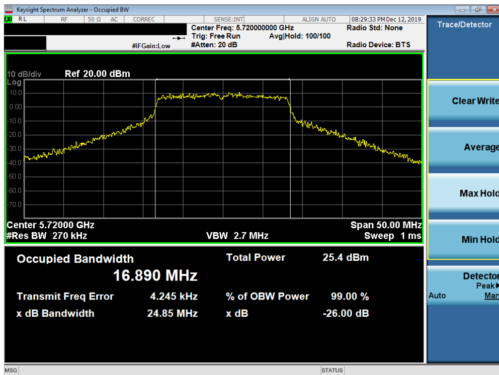
Plot 7-51. 26dB Bandwidth Plot SISO ANT2 (802.11a (UNII Band 2C) – Ch. 144)
