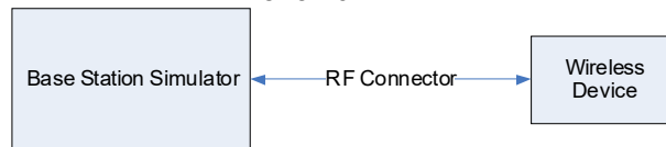
Figure 9-3 Power Measurement Setup
