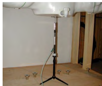
Figure 10-2 System Verification Setup Photo
