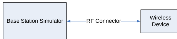
Figure 9-1 Power Measurement Setup
