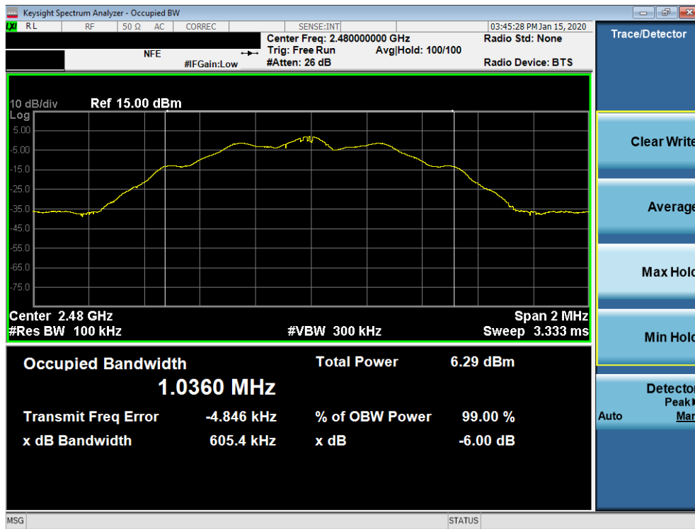
Plot 7-3. 6dB Bandwidth Plot (Bluetooth (LE), 125kbps – Ch. 39)
