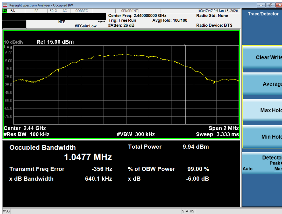
Plot 7-5. 6dB Bandwidth Plot (Bluetooth (LE), 500kbps – Ch. 19)
