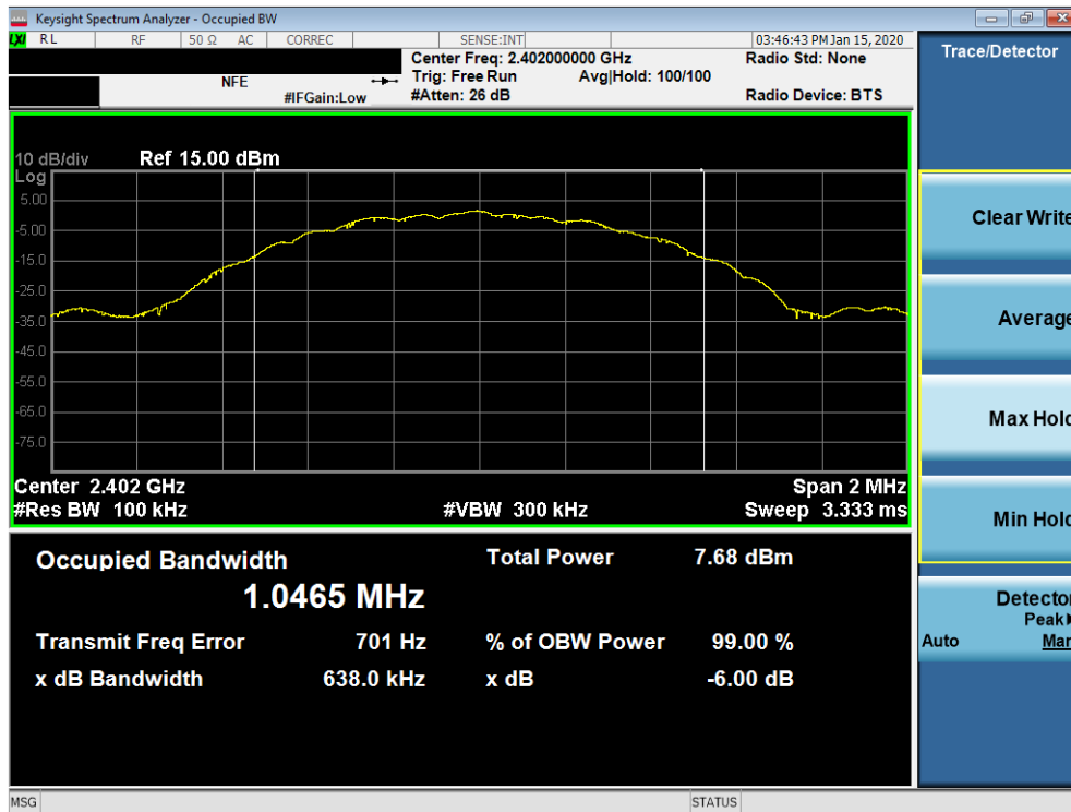
Plot 7-4. 6dB Bandwidth Plot (Bluetooth (LE), 500kbps – Ch. 0)
