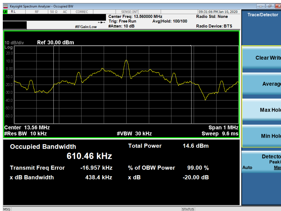
Figure 7-2. Occupied Bandwidth Plot
