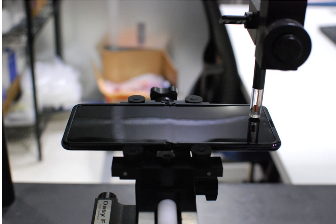
Figure 16-1 Test Setup for Wireless Device
