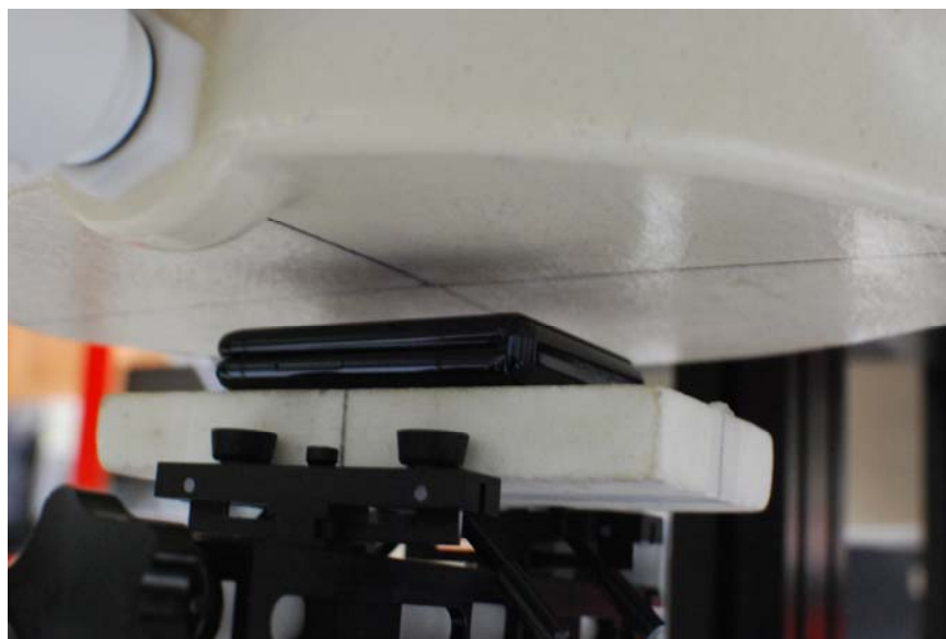
SAR Test Setup Photo 22 – Closed Back Side at 15 mm
