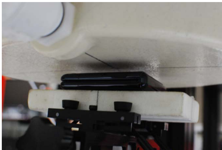
SAR Test Setup Photo 24 – Closed Front Side at 10 mm
