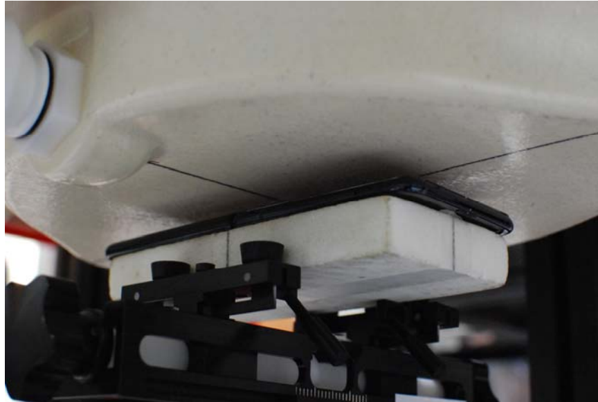
SAR Test Setup Photo 7 – Back Side at 9 mm
