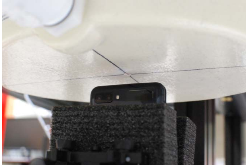
SAR Test Setup Photo 26 – Closed Bottom Edge at 10 mm
