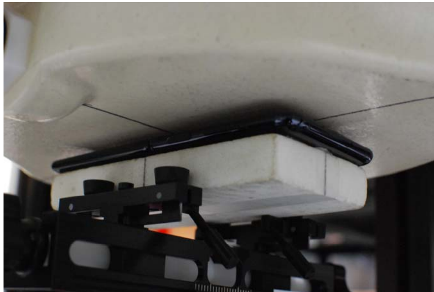
SAR Test Setup Photo 10 – Front Side at 7 mm
