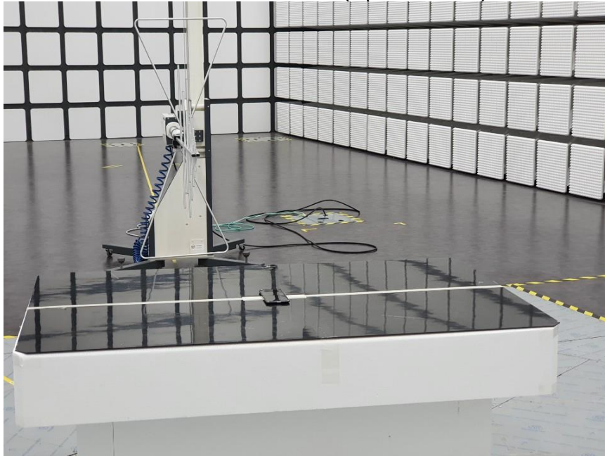
BELOW 1 GHz REAR TEST PHOTO(Open & X axis)
