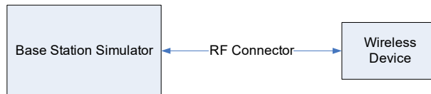
Figure 9-3 Power Measurement Setup
