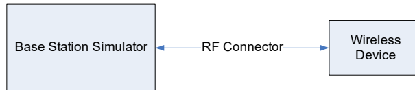
Figure 9-1 Power Measurement Setup
