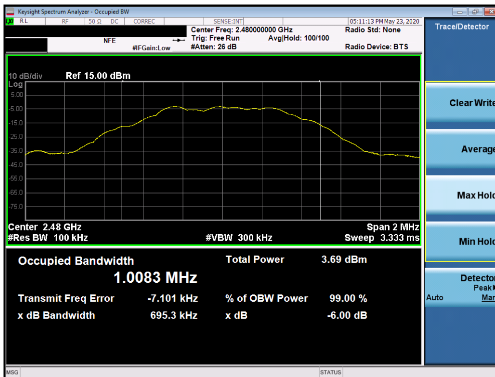
Plot 7-6. 6dB Bandwidth Plot (Bluetooth (LE), 500kbps – Ch. 39)
