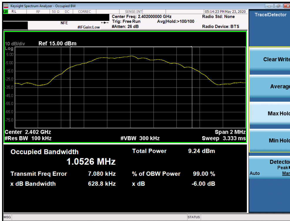
Plot 7-7. 6dB Bandwidth Plot (Bluetooth (LE), 1Mbps – Ch. 0)
