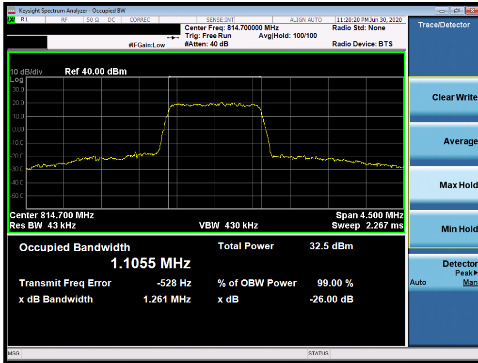
Plot 7-3. Occupied Bandwidth Plot (LTE Band 26 - 1.4MHz QPSK - Full RB Configuration)
