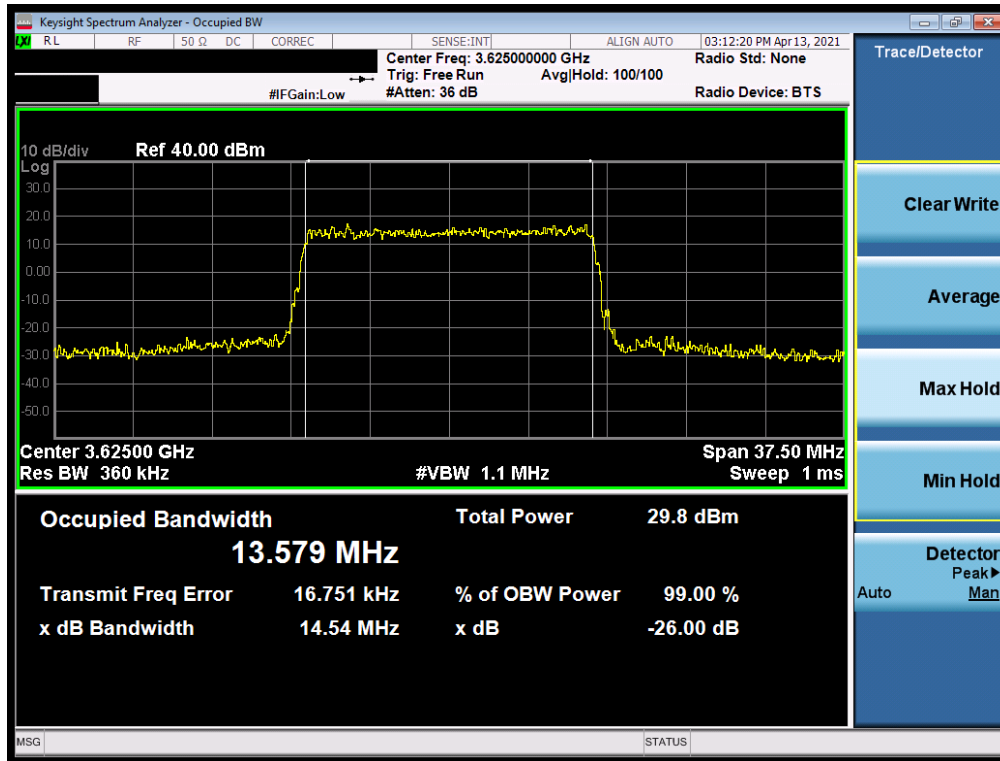
Plot 7-3. Occupied Bandwidth Plot (LTE Band 48 - 15MHz QPSK - Full RB Configuration)
