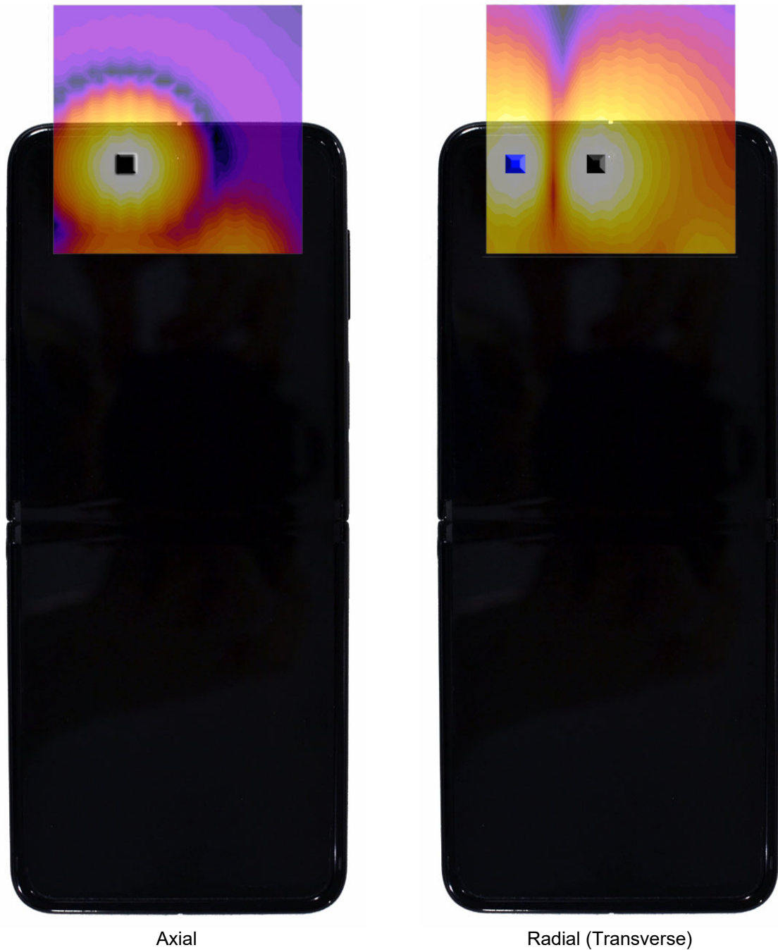
Figure 16-3 T-Coil Scan Overlay Magnetic Field Distributions
