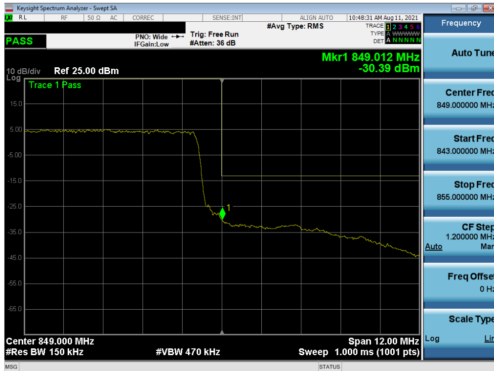
Plot 7-73. Upper Band Edge Plot (LTE Band 26 - 15MHz QPSK – Full RB)
