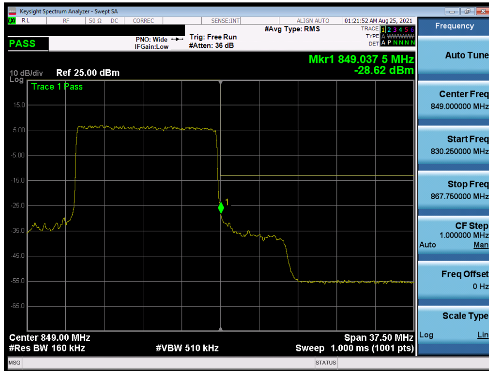
Plot 7-85. Upper Band Edge Plot (NR Band n5 – 15.0MHz - Full RB)
