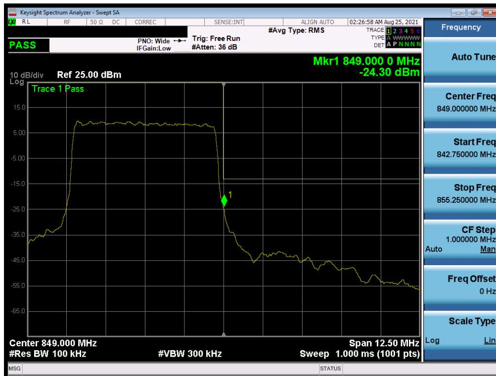
Plot 7-89. Upper Band Edge Plot (NR Band n5 – 5.0MHz - Full RB)
