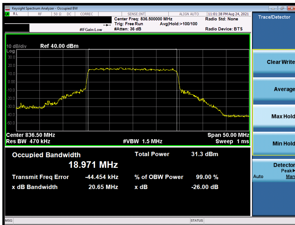
Plot 7-12. Occupied Bandwidth Plot (NR Band n5 - 20MHz QPSK - Full RB)
