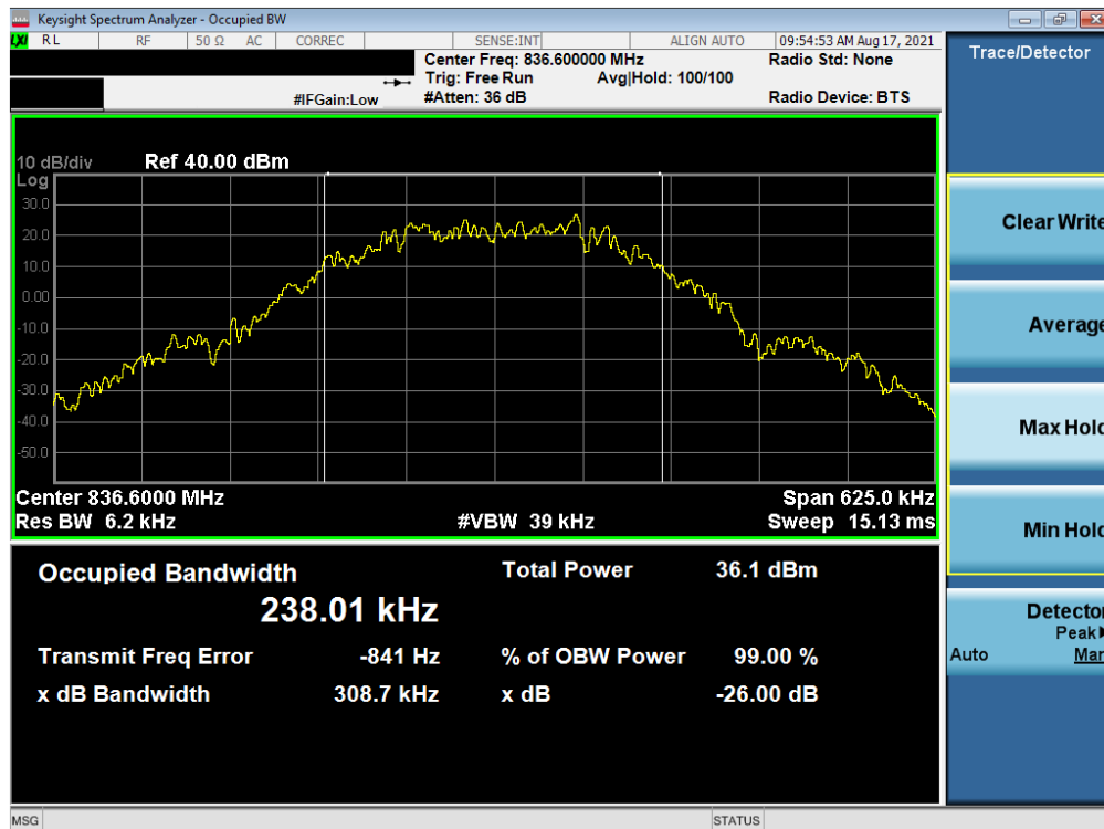
Plot 7-24. Occupied Bandwidth Plot (EDGE, Ch. 190)
