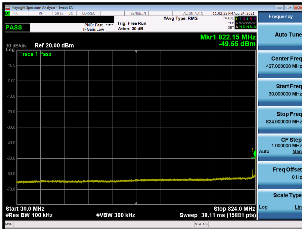
Plot 7-39. Conducted Spurious Plot (NR Band n5 - 20.0MHz - 1 RB - Mid Channel)
