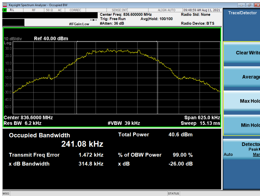
Plot 7-23. Occupied Bandwidth Plot (GPRS, Ch. 190)
