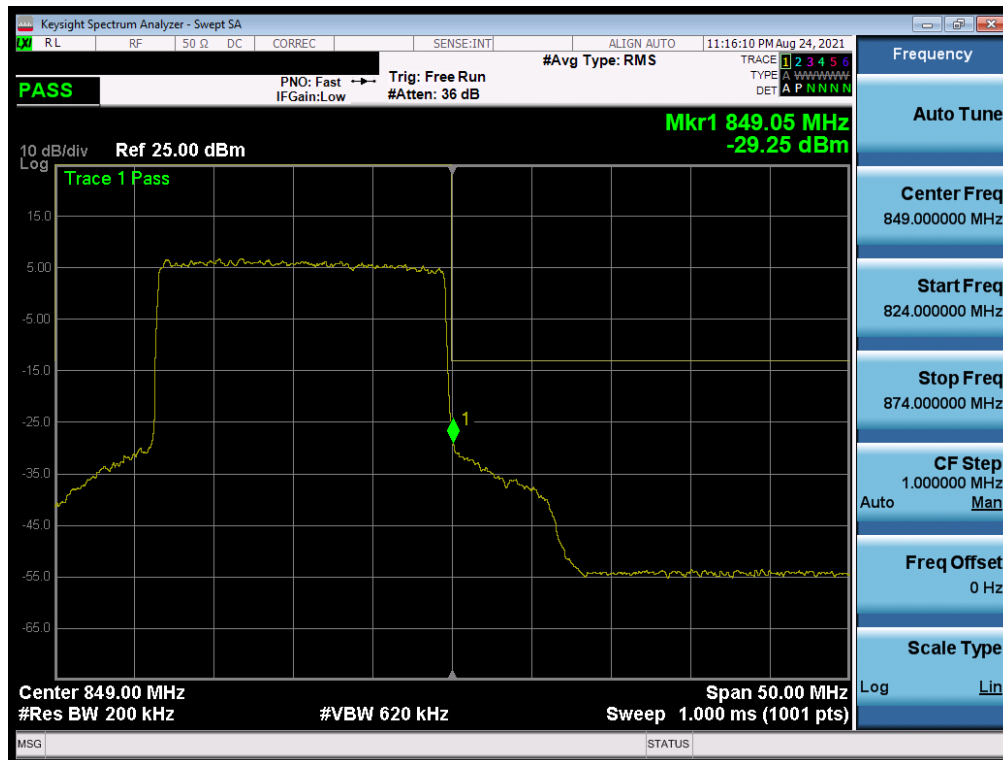
Plot 7-83. Upper Band Edge Plot (NR Band n5 – 20.0MHz - Full RB)
