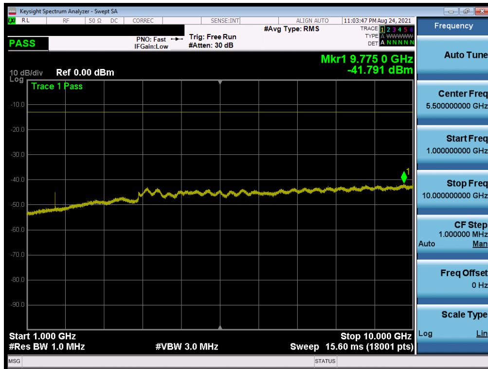
Plot 7-41. Conducted Spurious Plot (NR Band n5 - 20.0MHz - 1 RB - Mid Channel)
