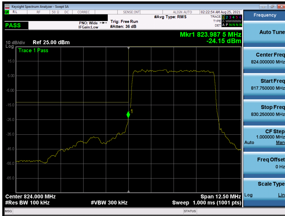
Plot 7-88. Lower Band Edge Plot (NR Band n5 – 5.0MHz - Full RB)
