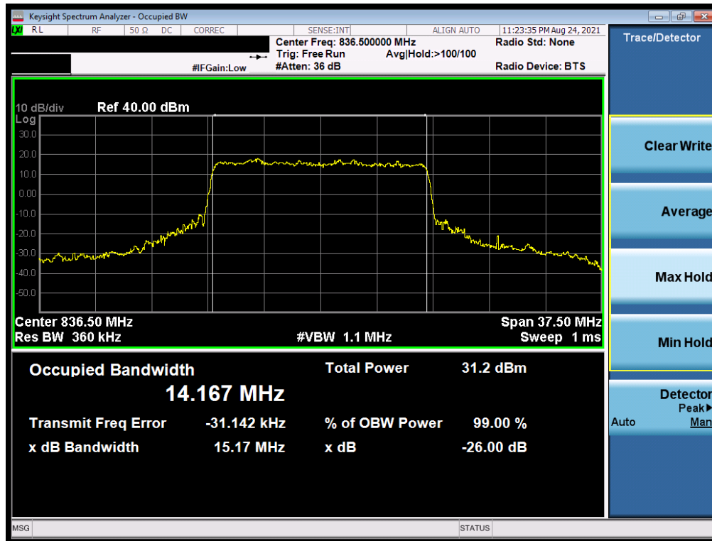
Plot 7-16. Occupied Bandwidth Plot (NR Band n5 - 15MHz 16-QAM - Full RB)
