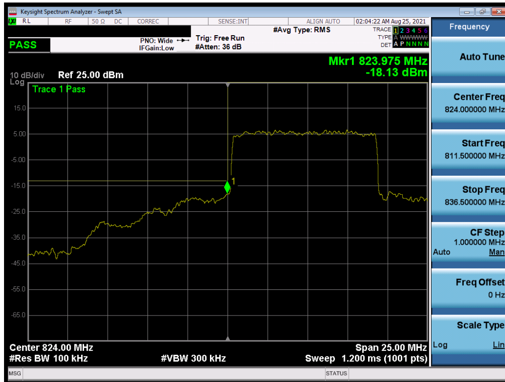
Plot 7-86. Lower Band Edge Plot (NR Band n5 – 10.0MHz - Full RB)
