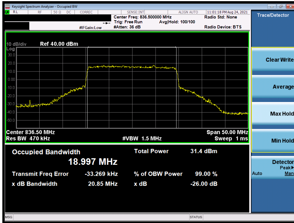
Plot 7-13. Occupied Bandwidth Plot (NR Band n5 - 20MHz 16-QAM - Full RB)
