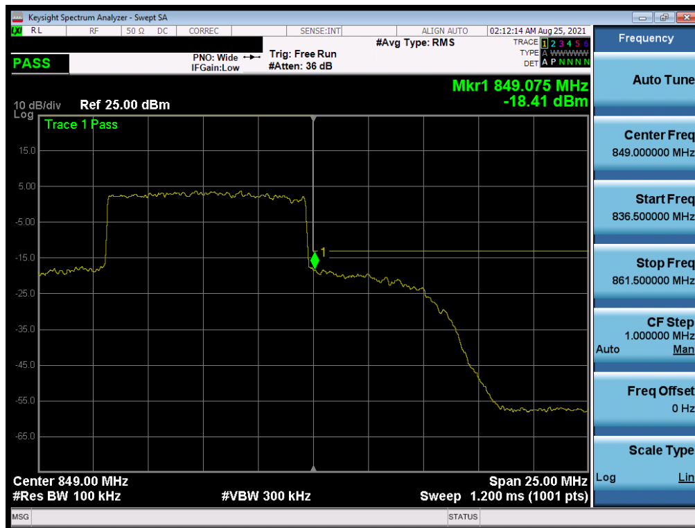
Plot 7-87. Upper Band Edge Plot (NR Band n5 – 10.0MHz - Full RB)
