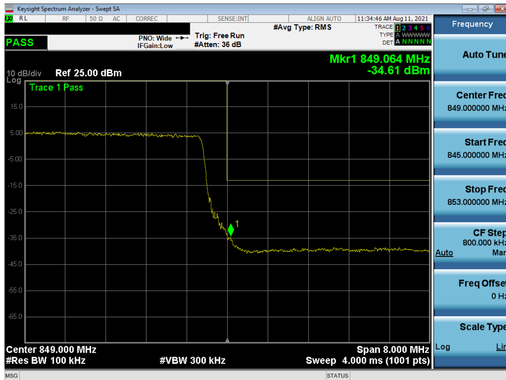
Plot 7-75. Upper Band Edge Plot (LTE Band 26/5 - 10MHz QPSK – Full RB)
