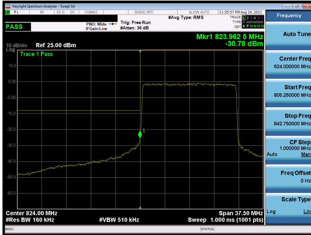
Plot 7-84. Lower Band Edge Plot (NR Band n5 – 15.0MHz - Full RB)
