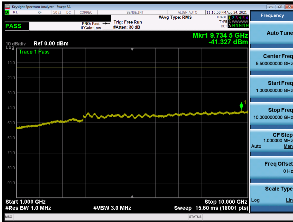
Plot 7-38. Conducted Spurious Plot (NR Band n5 - 20.0MHz - 1 RB - Low Channel)
