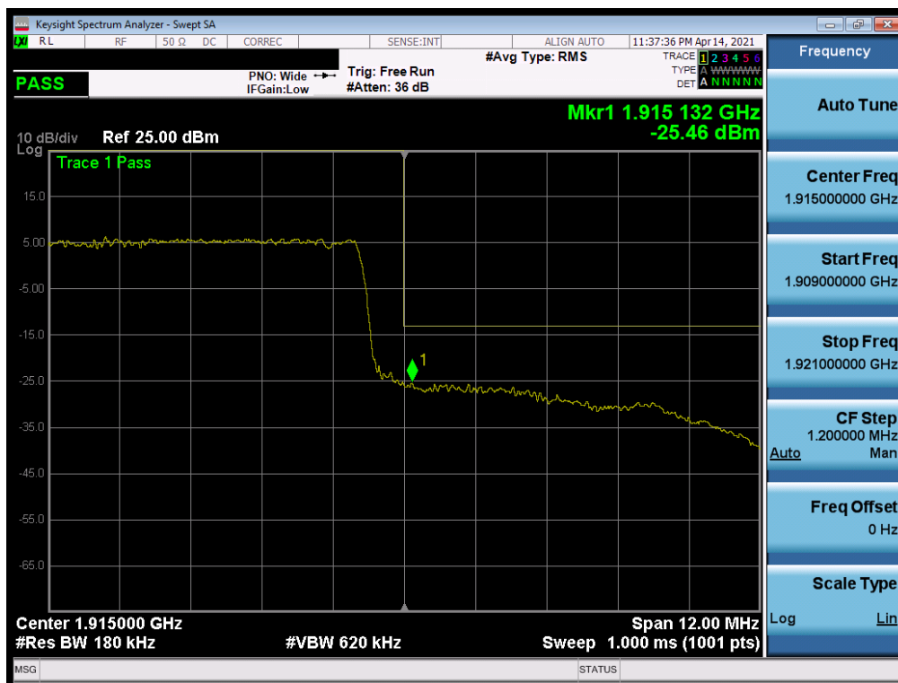
Plot 7-123. Upper Band Edge Plot (LTE Band 25 - 15MHz QPSK – Full RB)
