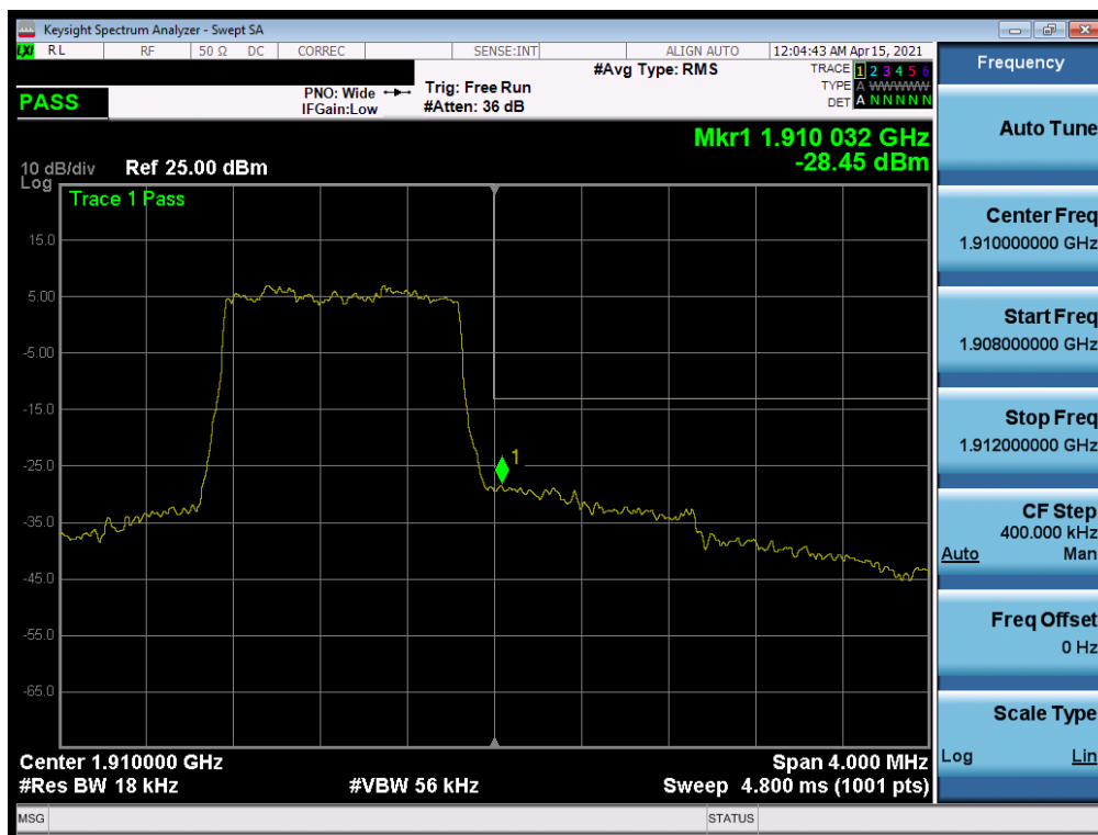
Plot 7-145. Upper Band Edge Plot (LTE Band 2 – 1.4MHz QPSK – Full RB)
