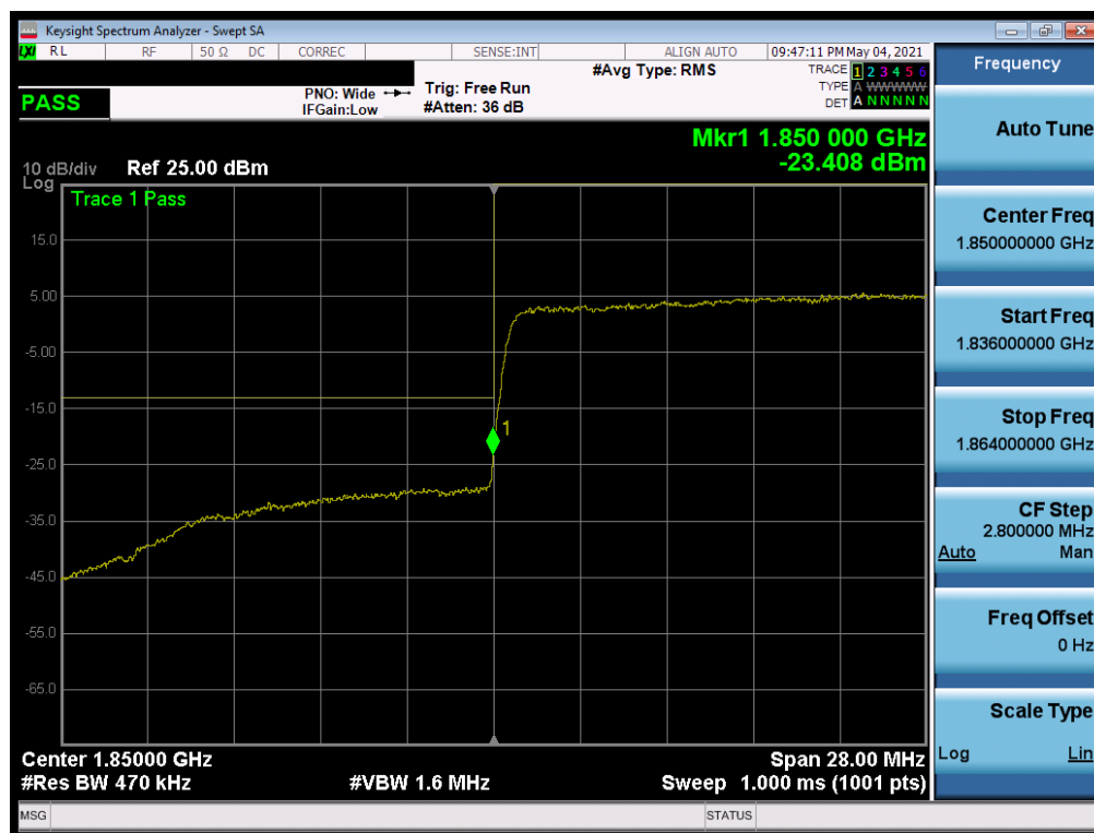
Plot 7-185. Lower Band Edge Plot (NR Band n25 – 40MHz QPSK – Full RB)
