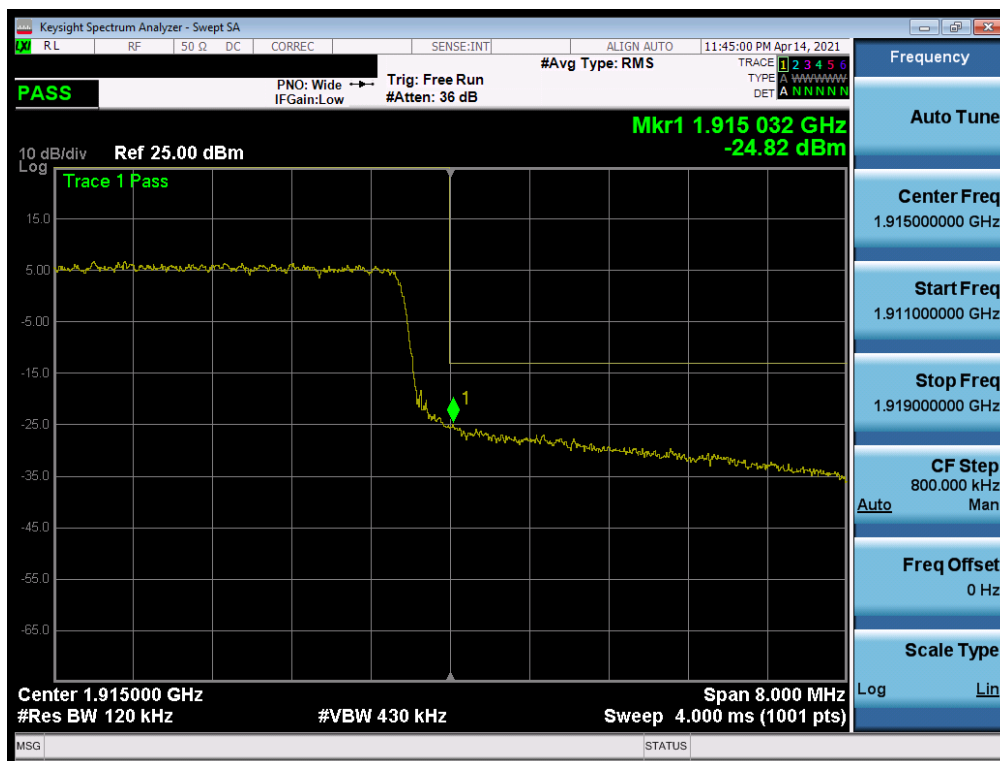
Plot 7-129. Upper Band Edge Plot (LTE Band 25 - 10MHz QPSK – Full RB)
