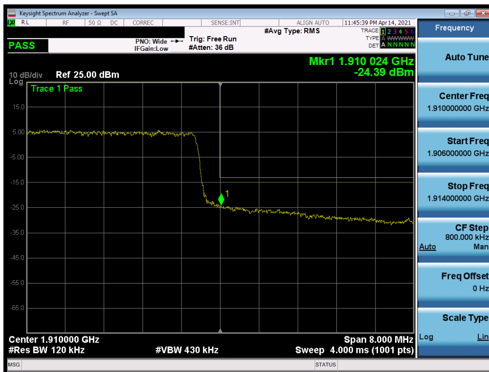
Plot 7-127. Upper Band Edge Plot (LTE Band 2 - 10MHz QPSK – Full RB)
