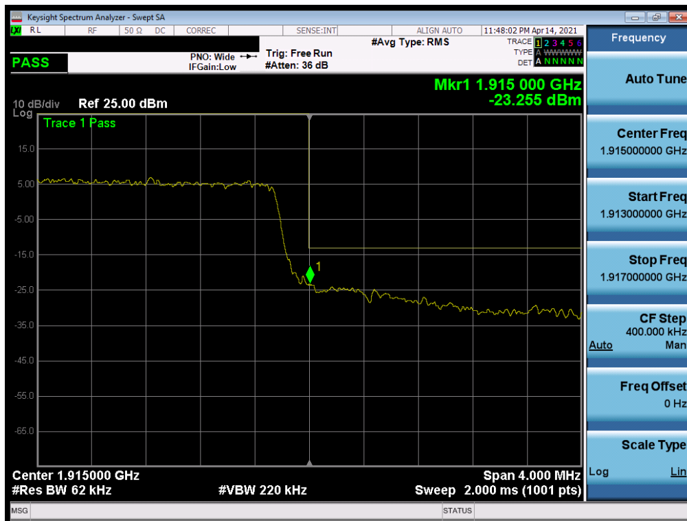
Plot 7-135. Upper Band Edge Plot (LTE Band 25 - 5MHz QPSK – Full RB)
