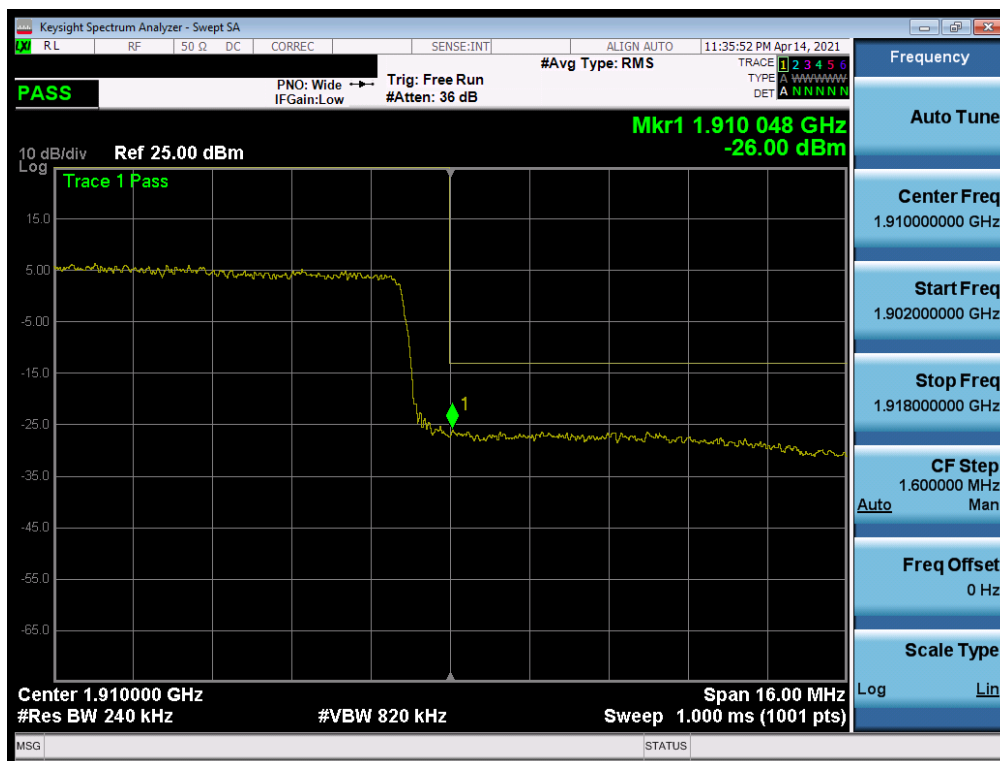
Plot 7-115. Upper Band Edge Plot (LTE Band 2 - 20MHz QPSK - Full RB)
