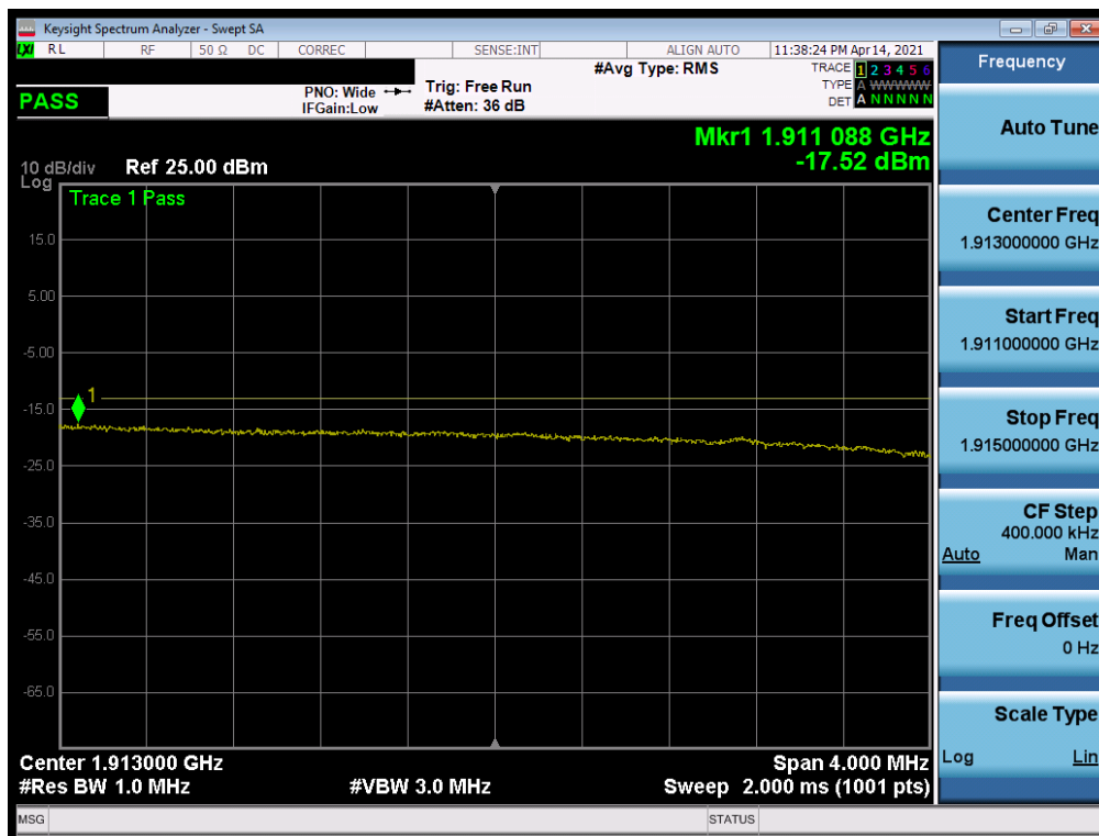
Plot 7-122. Extended Upper Band Edge Plot (LTE Band 2 - 15MHz QPSK - Full RB)
