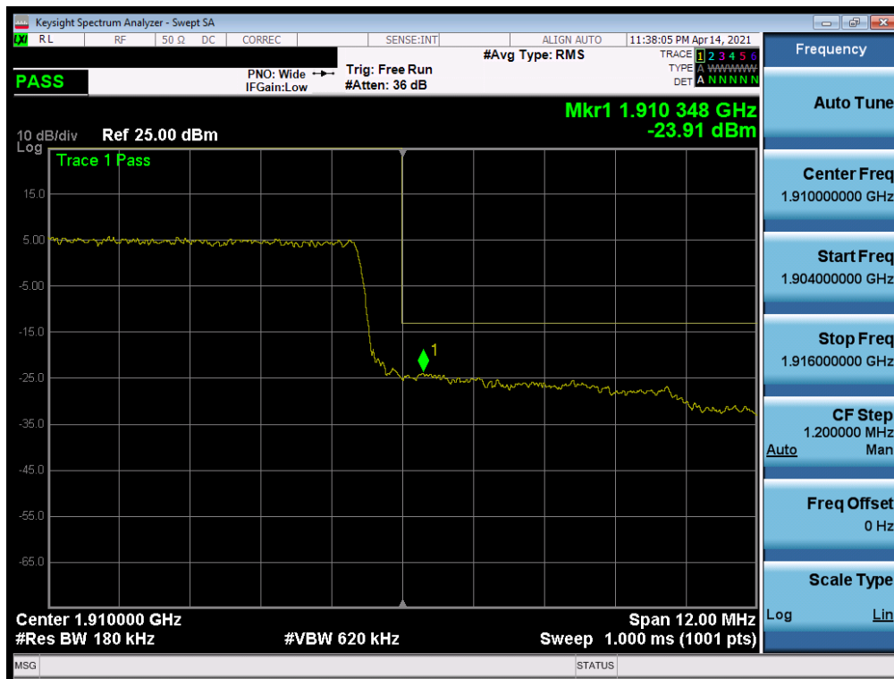
Plot 7-121. Upper Band Edge Plot (LTE Band 2 - 15MHz QPSK - Full RB)
