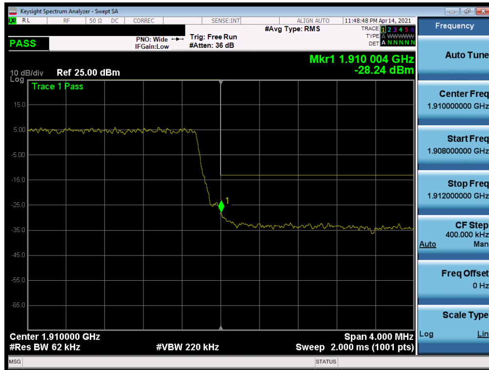
Plot 7-133. Upper Band Edge Plot (LTE Band 2 - 5MHz QPSK – Full RB)
