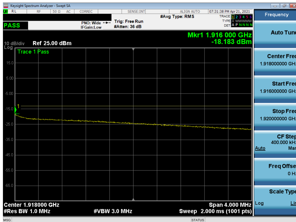
Plot 7-178. Extended Upper Band Edge Plot (NR Band n25 - 10MHz QPSK – Full RB)
