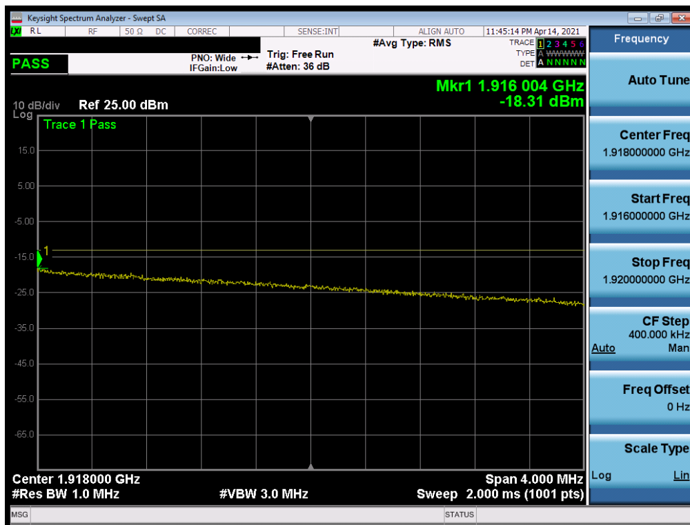
Plot 7-130. Extended Upper Band Edge Plot (LTE Band 25 - 10MHz QPSK – Full RB)
