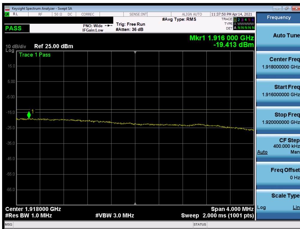
Plot 7-124. Extended Upper Band Edge Plot (LTE Band 25 - 15MHz QPSK – Full RB)
