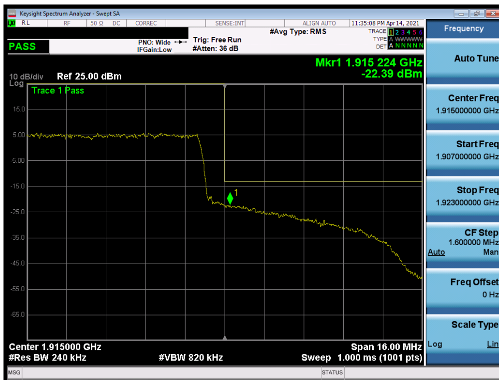
Plot 7-117. Upper Band Edge Plot (LTE Band 25 - 20MHz QPSK – Full RB)
