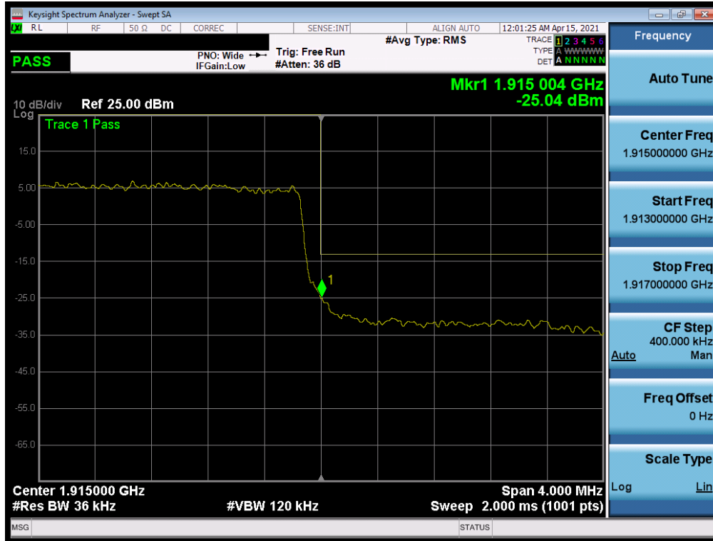
Plot 7-141. Upper Band Edge Plot (LTE Band 25 - 3MHz QPSK – Full RB)
