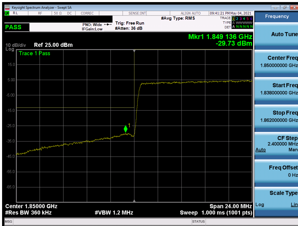
Plot 7-189. Lower Band Edge Plot (NR Band n25 - 30MHz QPSK - Full RB)
