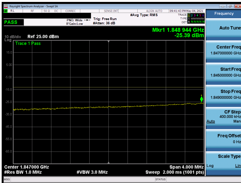
Plot 7-190. Extended Lower Band Edge Plot (NR Band n25 - 30MHz QPSK - Full RB)
