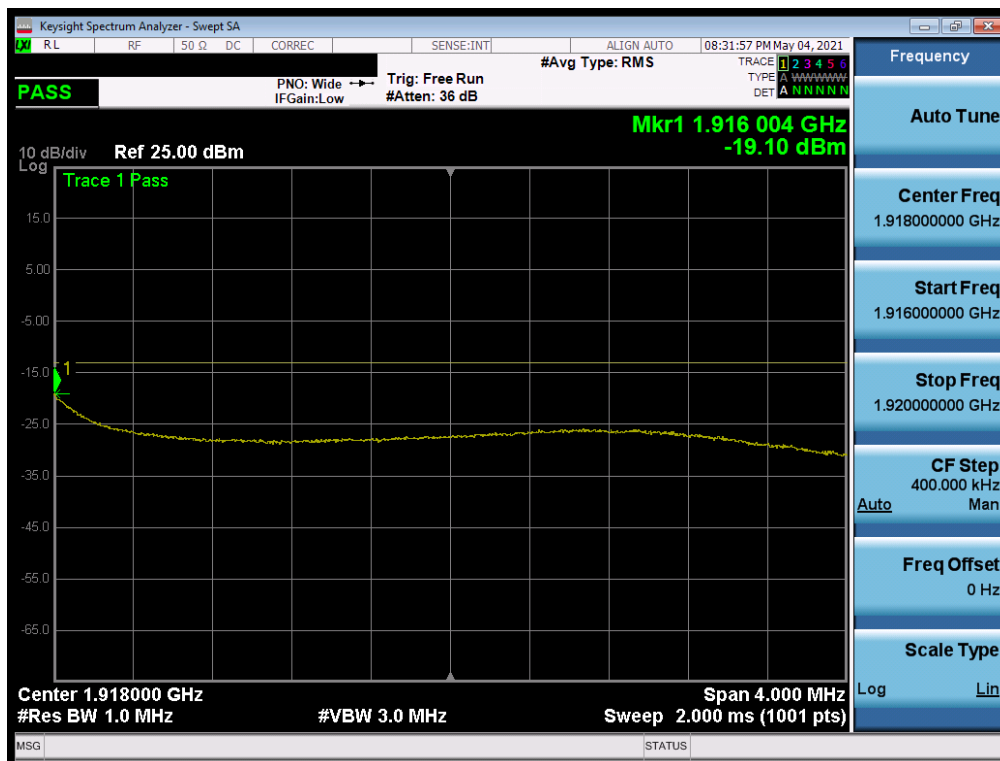
Plot 7-214. Extended Upper Band Edge Plot (NR Band n25 – 10MHz QPSK – Full RB)
