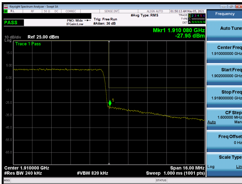
Plot 7-199. Upper Band Edge Plot (NR Band n2 – 20MHz QPSK – Full RB)
