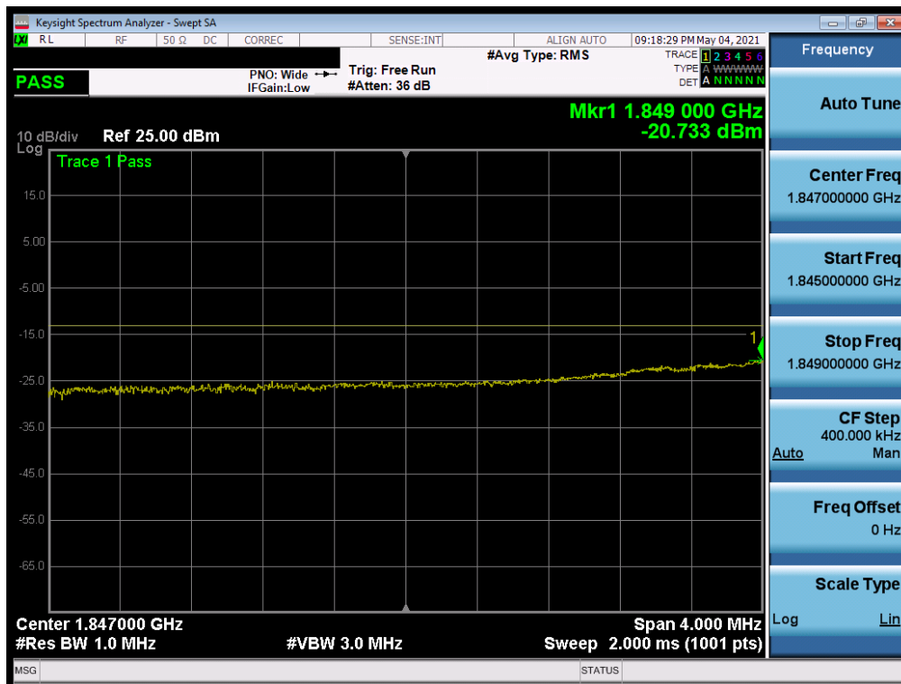
Plot 7-198. Extended Lower Band Edge Plot (NR Band n25/2 – 20MHz QPSK – Full RB)
