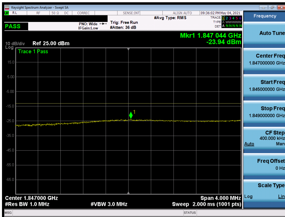
Plot 7-194. Extended Lower Band Edge Plot (NR Band n25 – 25MHz QPSK – Full RB)
