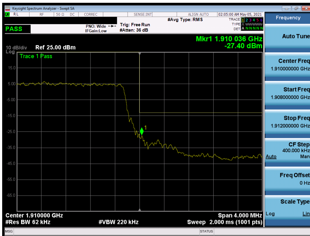
Plot 7-217. Upper Band Edge Plot (NR Band n2 – 5MHz QPSK – Full RB)
