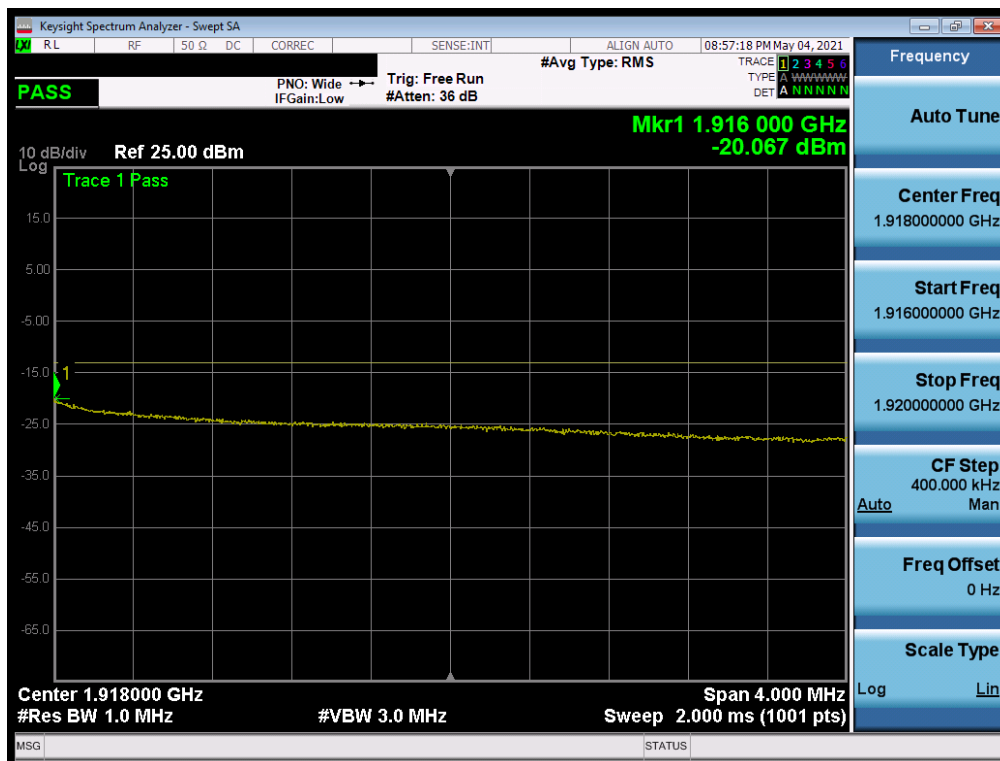
Plot 7-208. Extended Upper Band Edge Plot (NR Band n25 - 15MHz QPSK - Full RB)
