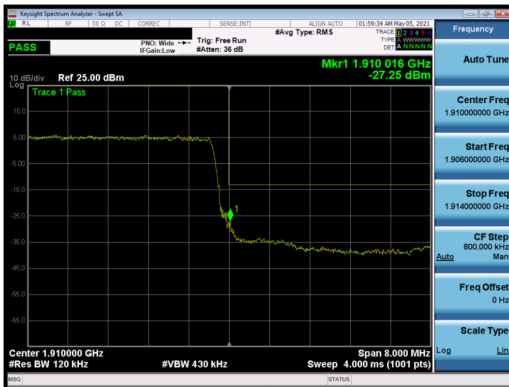
Plot 7-211. Upper Band Edge Plot (NR Band n2 - 10MHz QPSK - Full RB)
