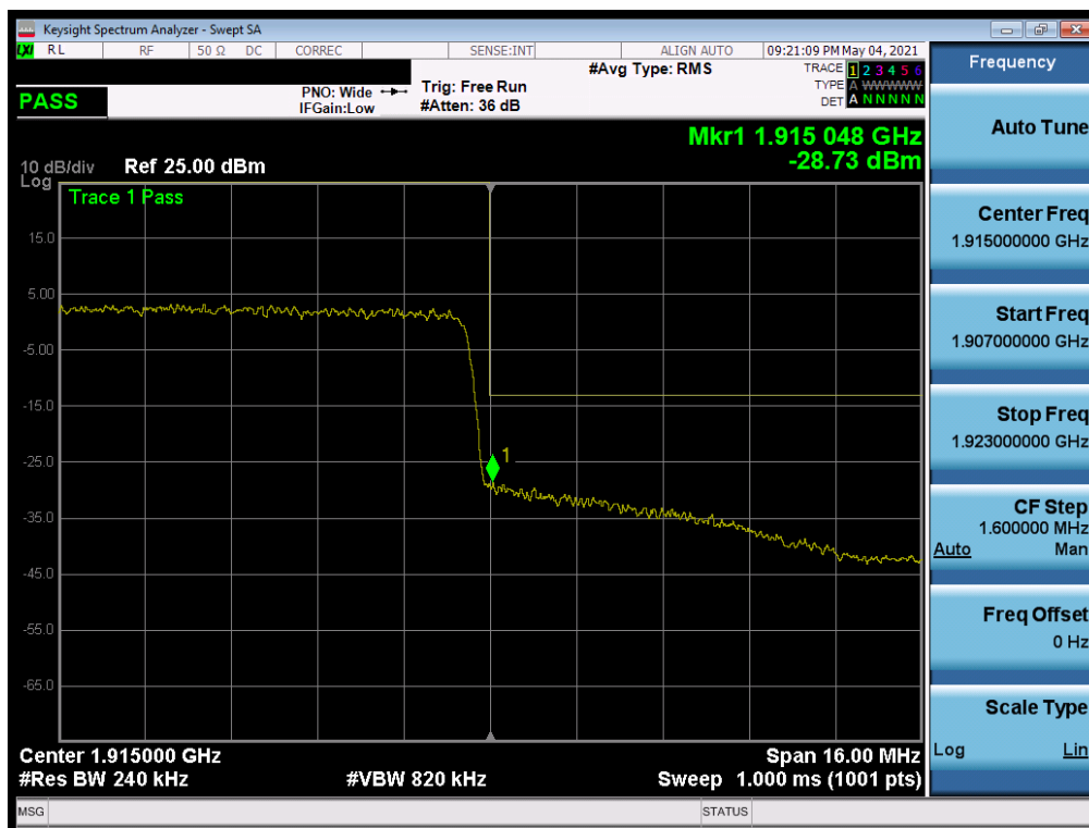
Plot 7-201. Upper Band Edge Plot (NR Band n25 – 20MHz QPSK – Full RB)
