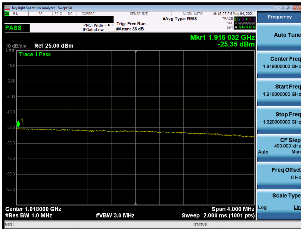
Plot 7-188. Extended Upper Band Edge Plot (NR Band n25 - 40MHz QPSK - Full RB)
