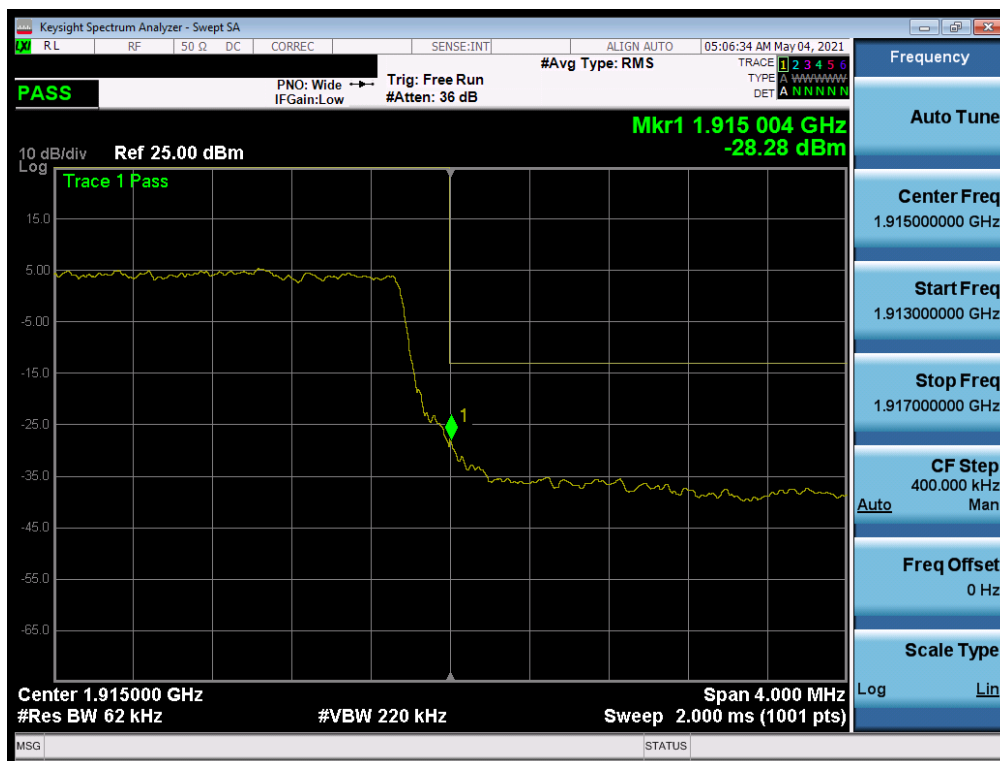
Plot 7-219. Upper Band Edge Plot (NR Band n25 – 5MHz QPSK – Full RB)
