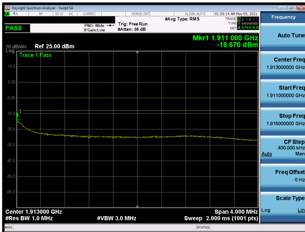
Plot 7-212. Extended Upper Band Edge Plot (NR Band n2 - 10MHz QPSK - Full RB 2)
