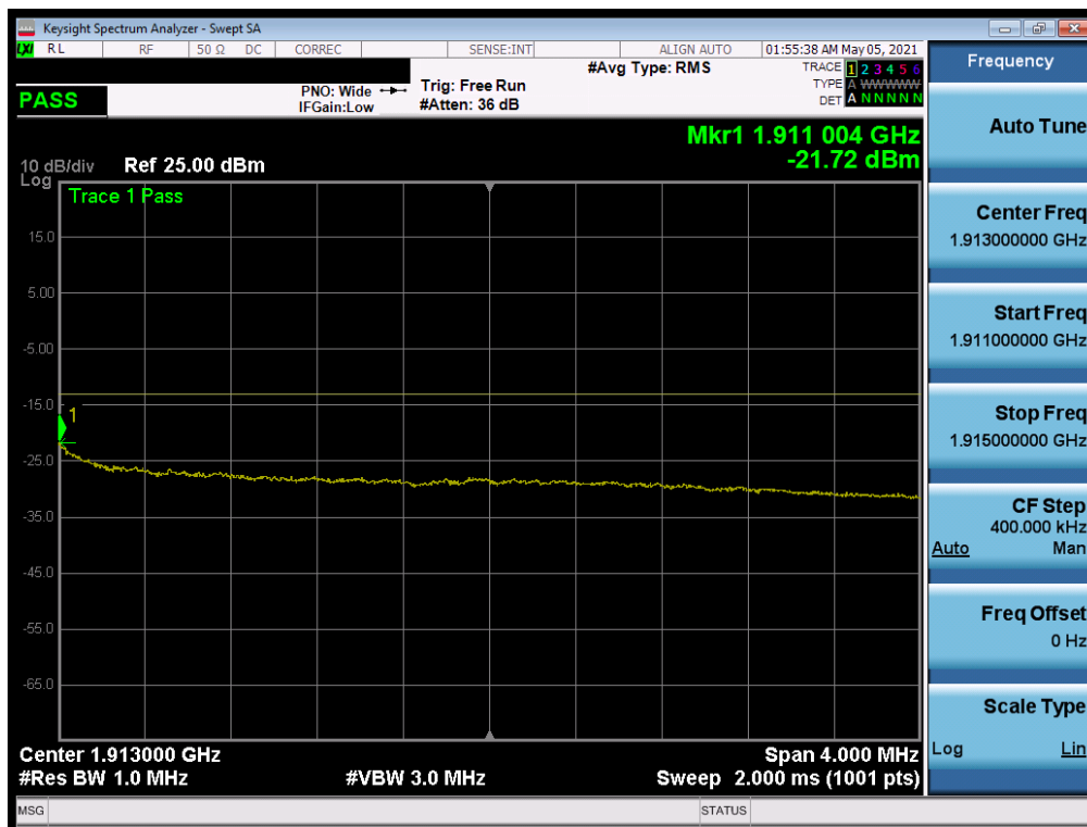
Plot 7-206. Extended Upper Band Edge Plot (NR Band n2 – 15MHz QPSK – Full RB)
