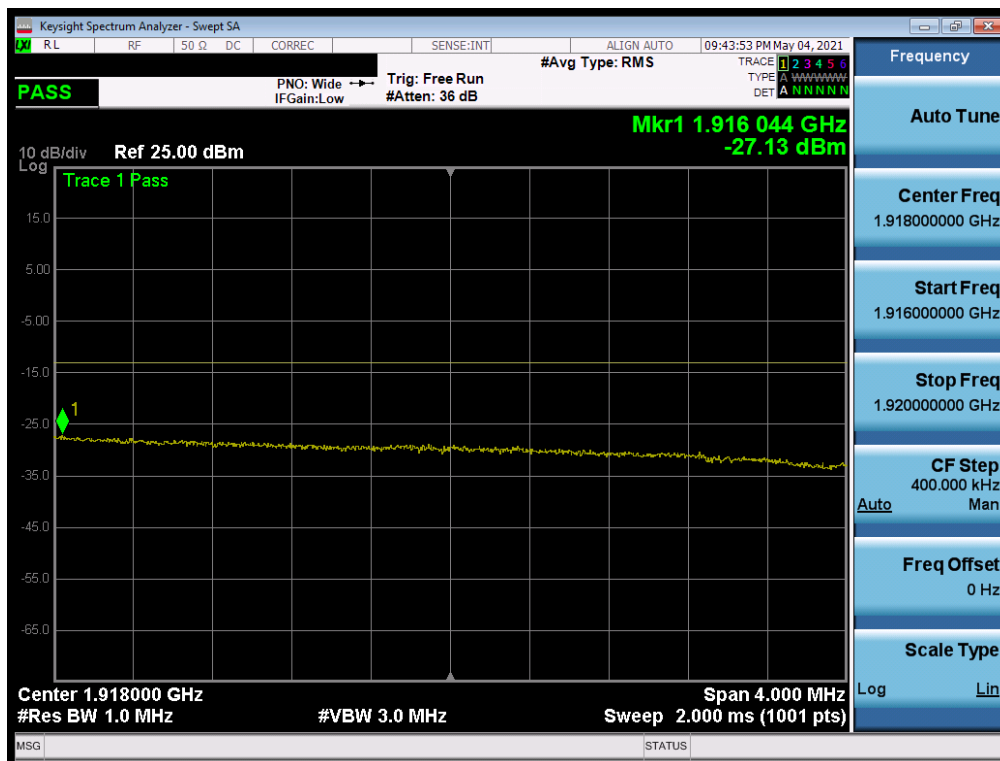
Plot 7-192. Extended Upper Band Edge Plot (NR Band n25 - 30MHz QPSK - Full RB)
