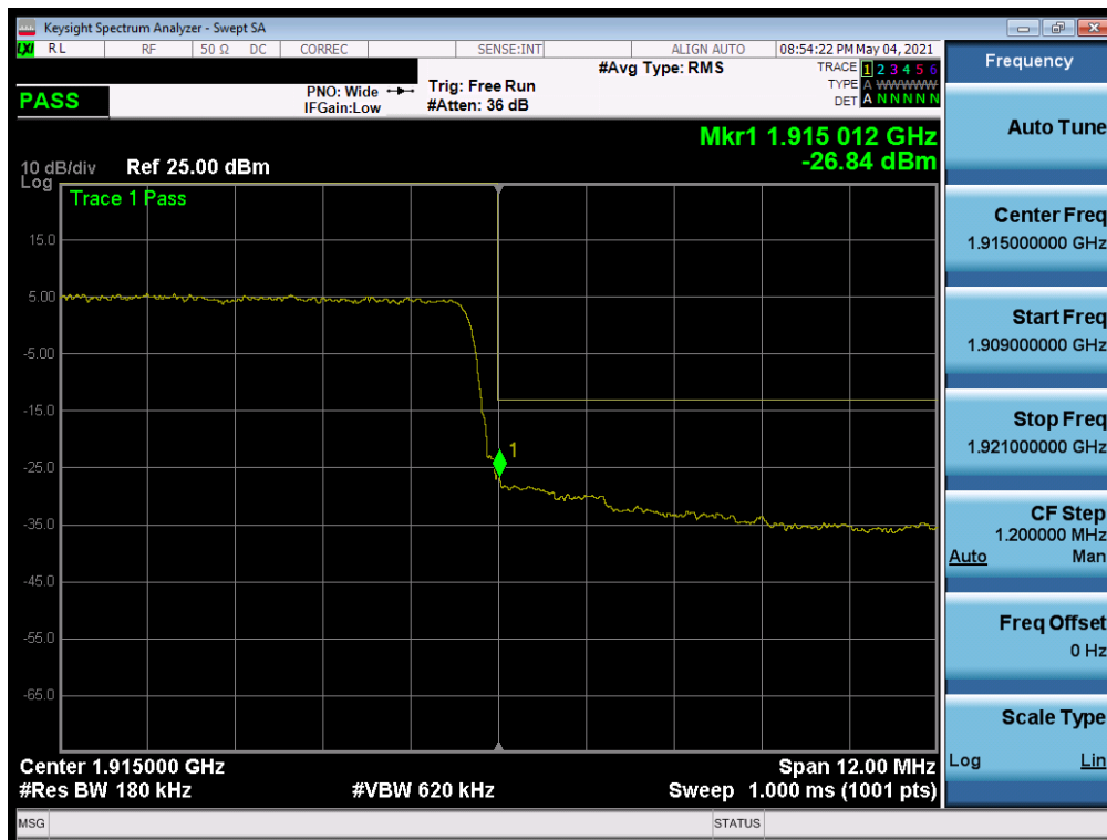
Plot 7-207. Upper Band Edge Plot (NR Band n25 - 15MHz QPSK - Full RB)
