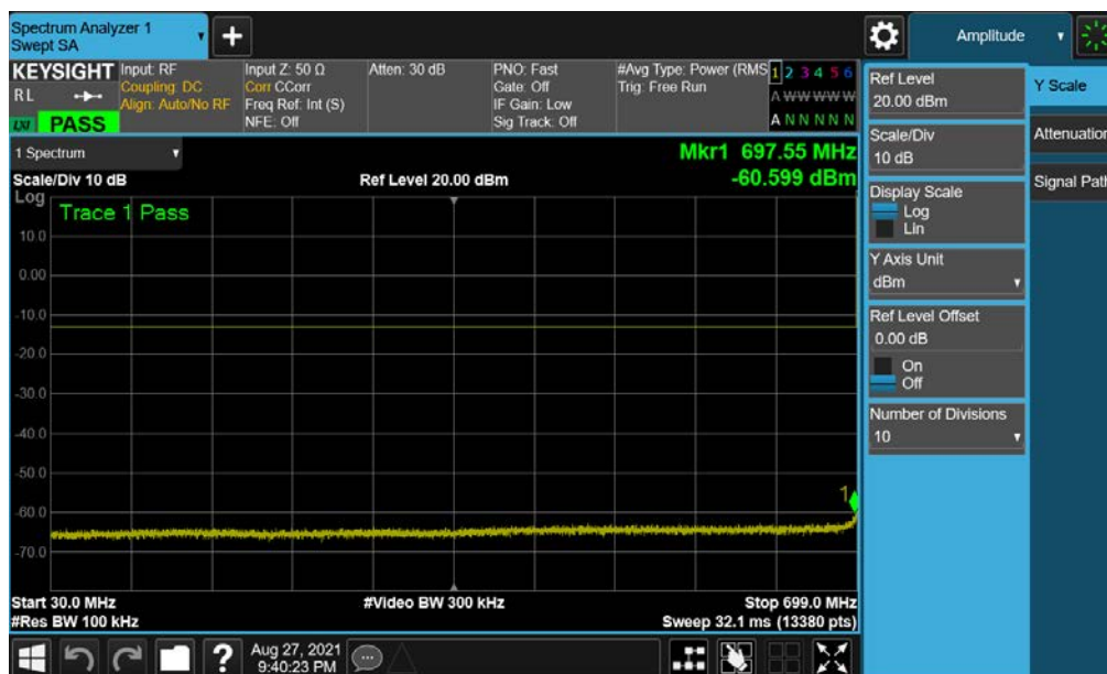
Plot 7-124. Conducted Spurious Plot (NR Band n12 - 15.0MHz - 1 RB - Mid Channel - Ant I)
