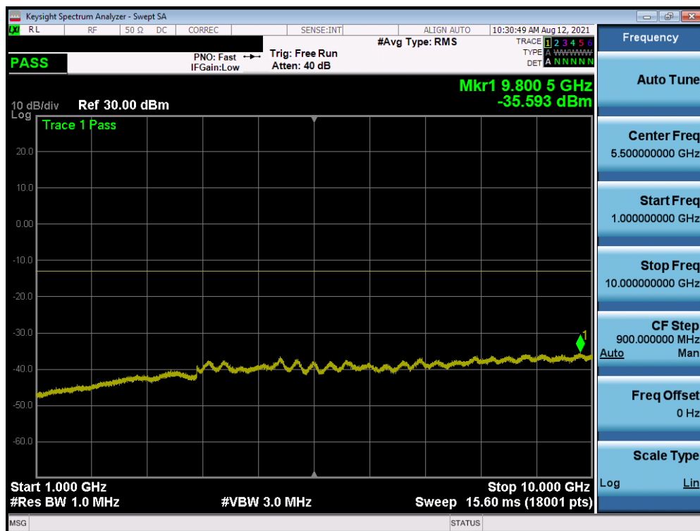
Plot 7-105. Conducted Spurious Plot (LTE Band 12 - 10MHz QPSK - 1 RB - Mid Channel - Ant I)
