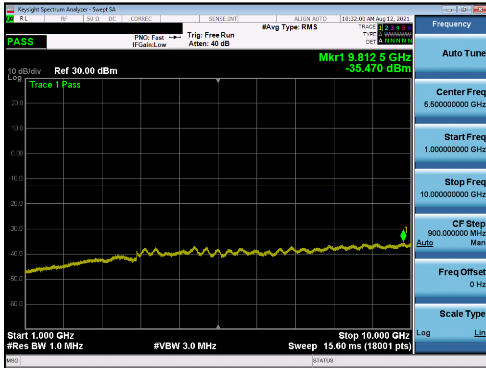
Plot 7-108. Conducted Spurious Plot (LTE Band 12 - 10MHz QPSK - 1 RB - High Channel - Ant I)
