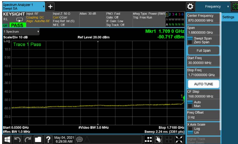
Plot 7-157. Conducted Spurious Plot (NR Band n66 -40.0MHz - 1 RB - Low Channel)
