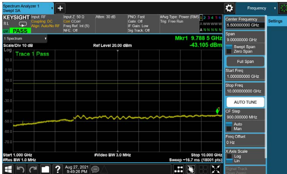
Plot 7-123. Conducted Spurious Plot (NR Band n12 - 15.0MHz - 1 RB - Low Channel - Ant I)
