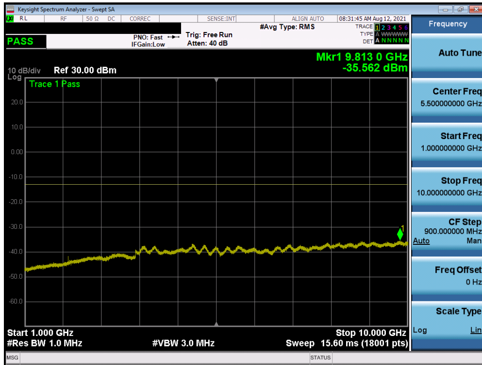
Plot 7-93. Conducted Spurious Plot (LTE Band 71 - 20.0MHz - 1 RB - Low Channel - Ant I)
