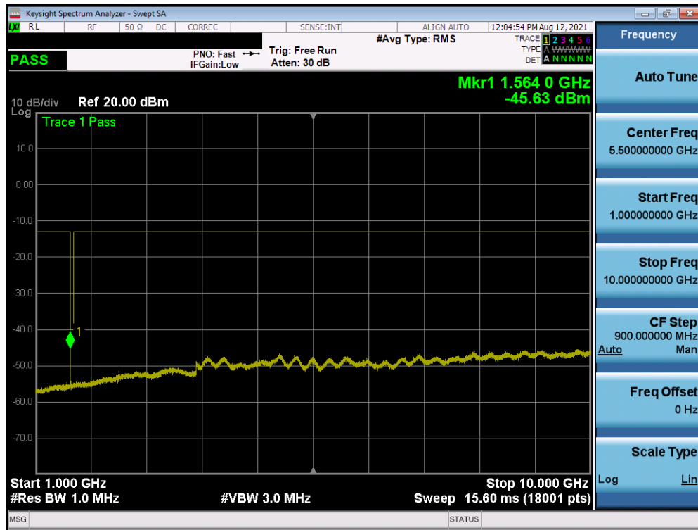
Plot 7-111. Conducted Spurious Plot (LTE Band 13 - 10MHz QPSK - 1 RB)
