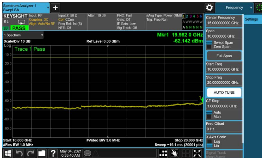
Plot 7-162. Conducted Spurious Plot (NR Band n66 - 40.0MHz - 1 RB - Mid Channel)
