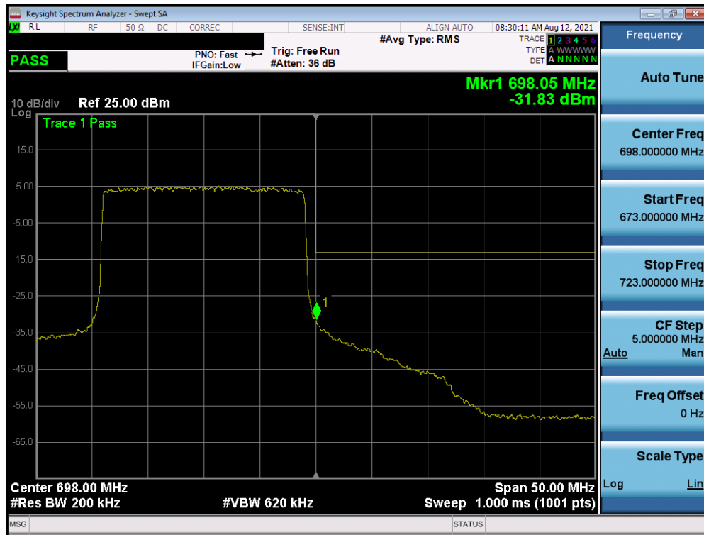
Plot 7-167. Upper Band Edge Plot (LTE Band 71 - 20MHz QPSK – Full RB - Ant I)
