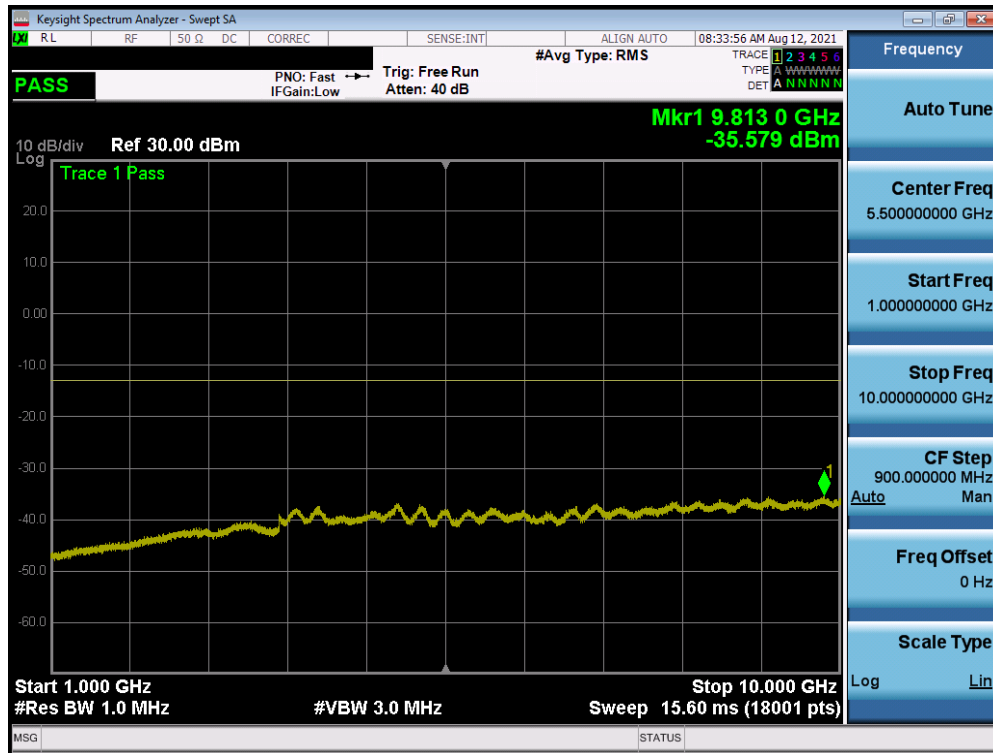
Plot 7-99. Conducted Spurious Plot (LTE Band 71 - 20.0MHz - 1 RB - High Channel - Ant I)
