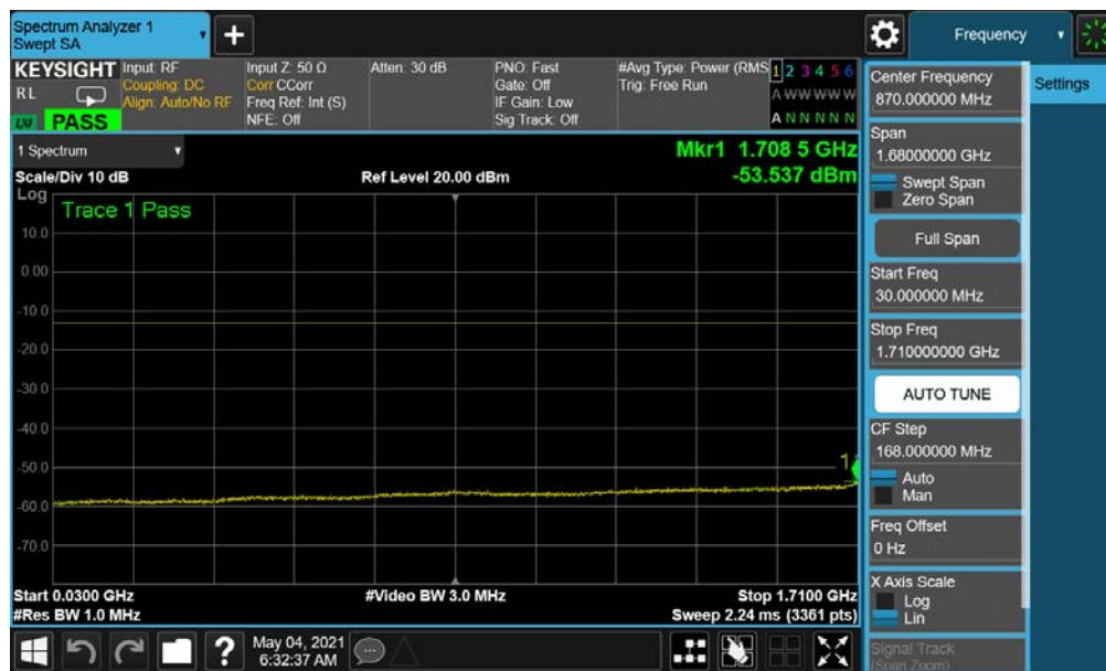
Plot 7-160. Conducted Spurious Plot (NR Band n66 - 40.0MHz - 1 RB - Mid Channel)
