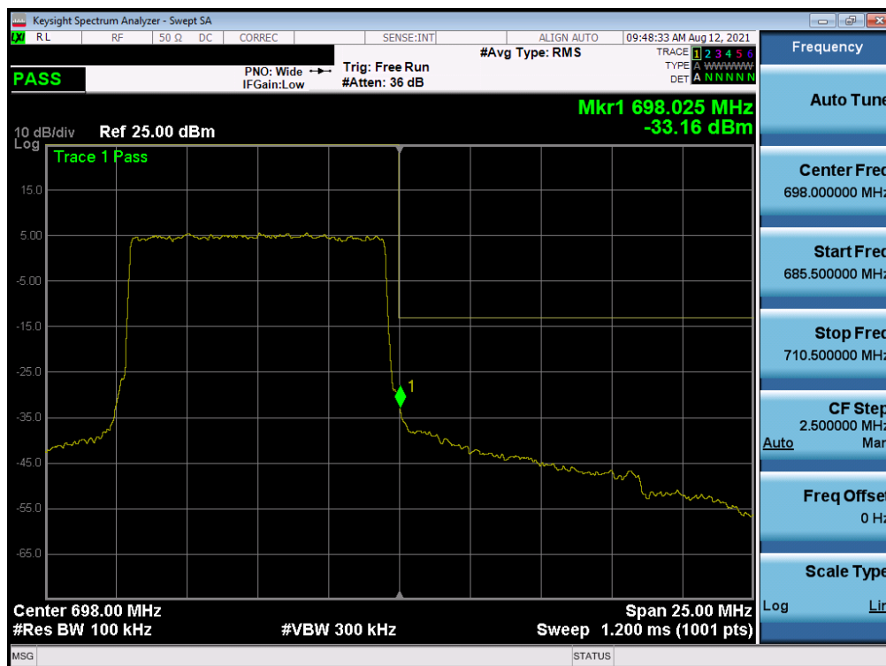
Plot 7-171. Upper Band Edge Plot (LTE Band 71 - 10MHz QPSK - Full RB - Ant I)
