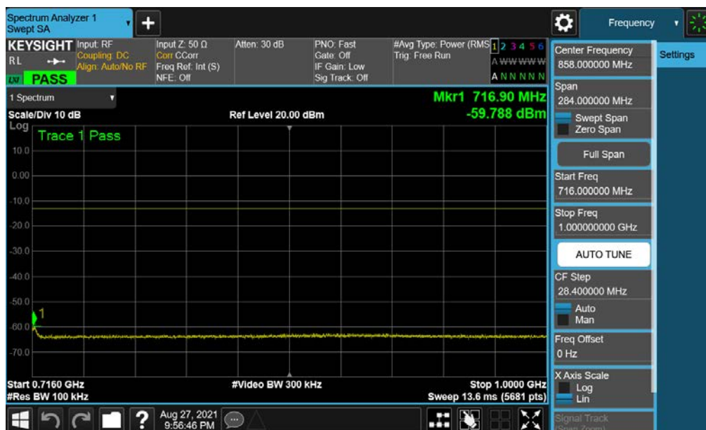
Plot 7-128. Conducted Spurious Plot (NR Band n12 - 15.0MHz - 1 RB - High Channel - Ant I)
