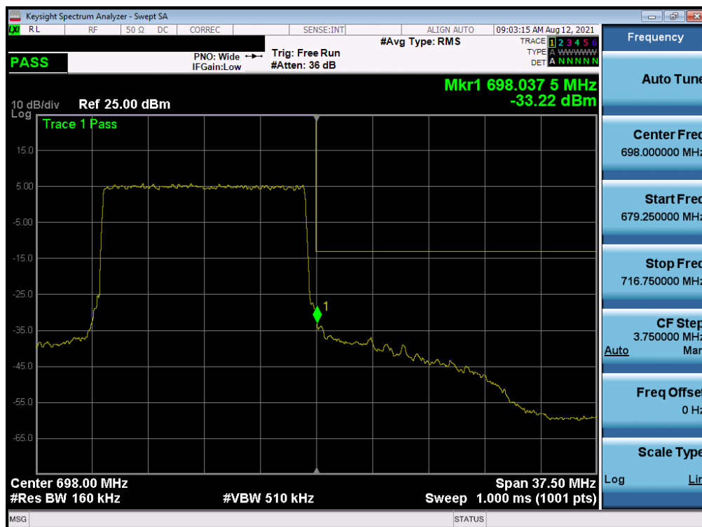
Plot 7-169. Upper Band Edge Plot (LTE Band 71 - 15MHz QPSK - Full RB - Ant I)
