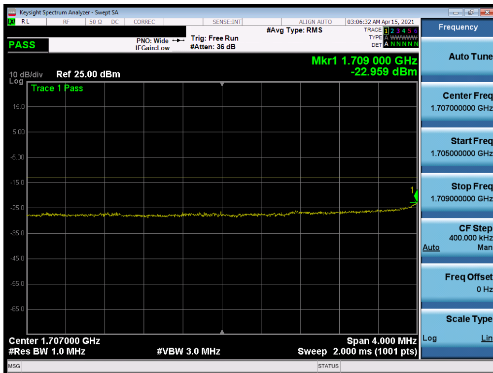
Plot 7-221. Lower Extended Band Edge Plot (LTE Band 66/4 - 10MHz QPSK – Full RB)
