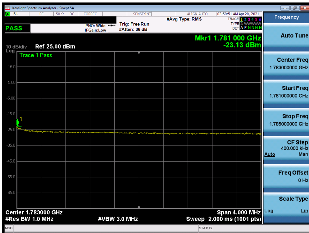
Plot 7-259. Upper Extended Band Edge Plot (NR Band n66 – 15.0MHz - Full RB)
