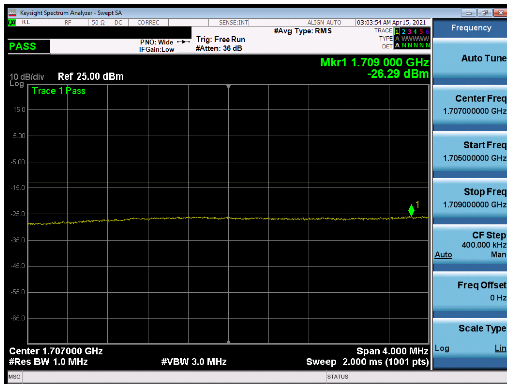
Plot 7-215. Lower Extended Band Edge Plot (LTE Band 66/4 - 15MHz QPSK – Full RB)
