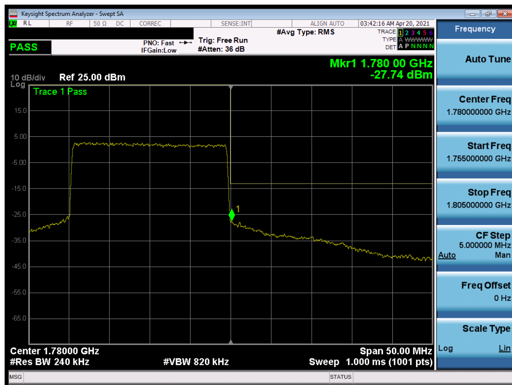
Plot 7-254. Upper Band Edge Plot (NR Band n66 – 20.0MHz - Full RB)
