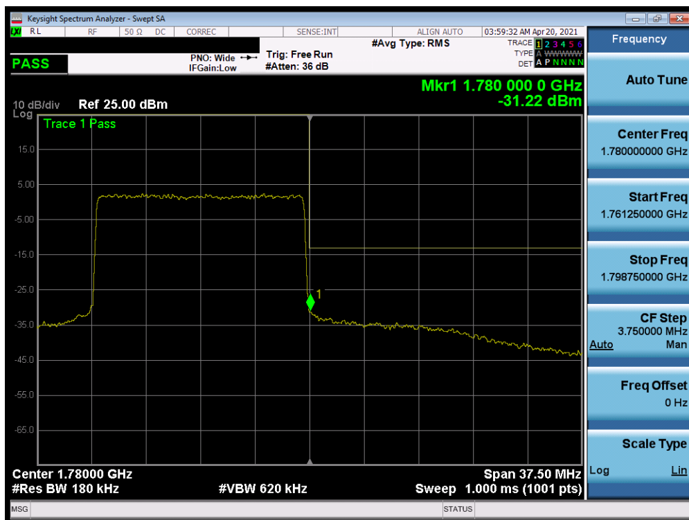
Plot 7-258. Upper Band Edge Plot (NR Band n66 – 15.0MHz - Full RB)
