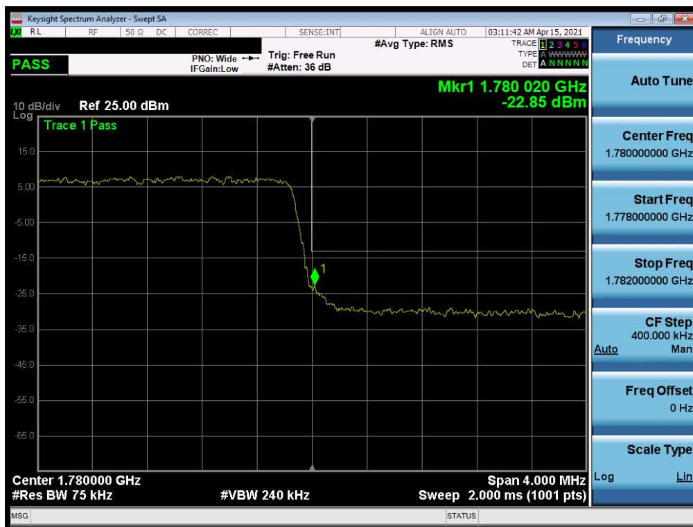
Plot 7-236. Upper Band Edge Plot (LTE Band 66 - 3MHz QPSK – Full RB)
