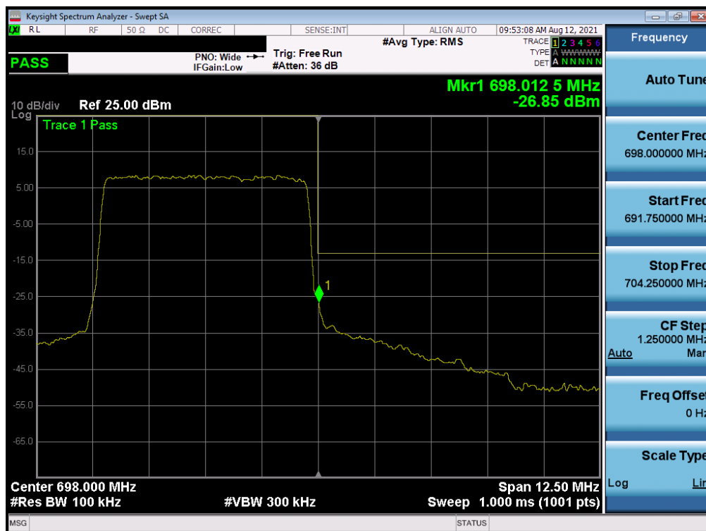
Plot 7-173. Upper Band Edge Plot (LTE Band 71 - 5MHz QPSK – Full RB - Ant I)
