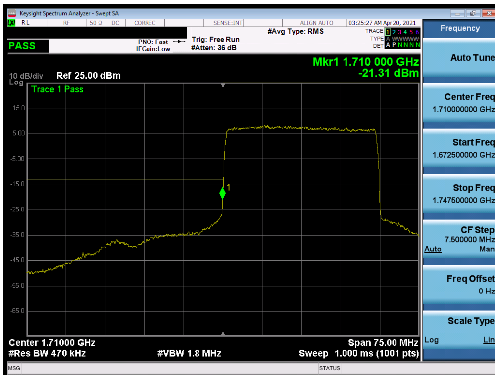
Plot 7-248. Lower Band Edge Plot (NR Band n66 – 30.0MHz - Full RB)
