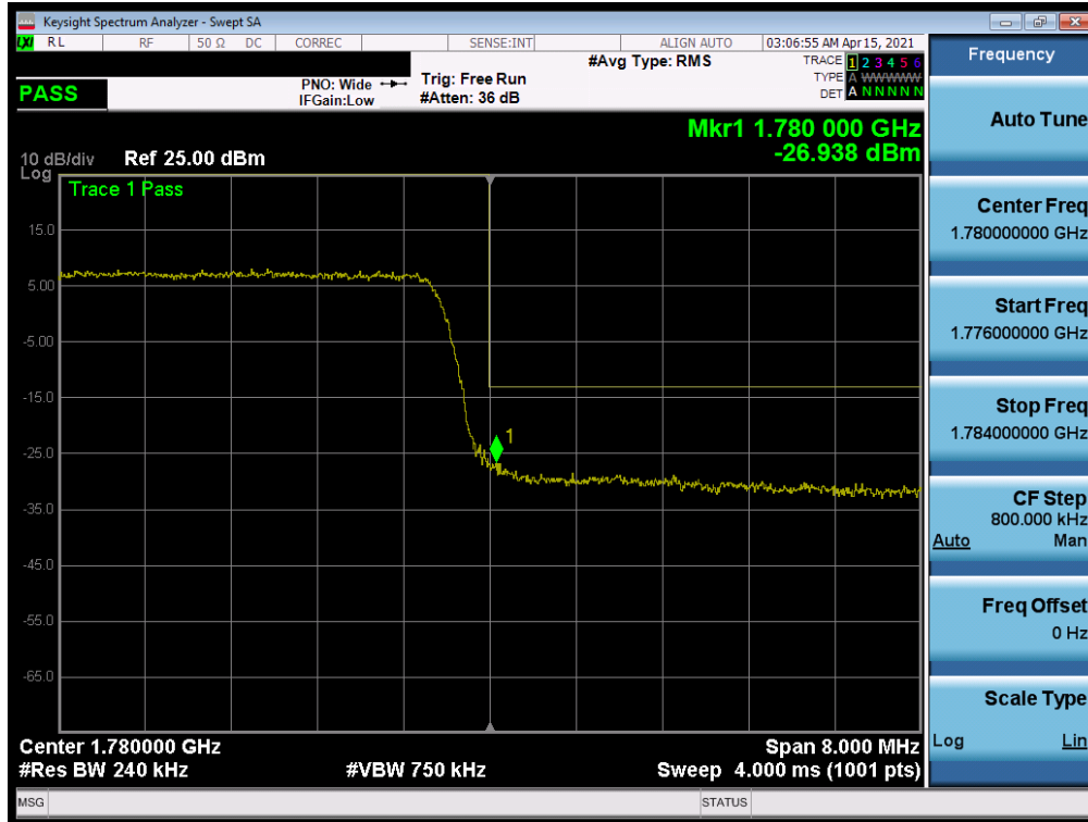
Plot 7-224. Upper Band Edge Plot (LTE Band 66 - 10MHz QPSK – Full RB)
