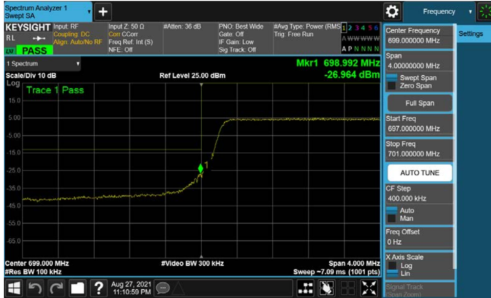
Plot 7-202. Lower Band Edge Plot (NR Band n12 – 5.0MHz - Full RB - Ant I)
