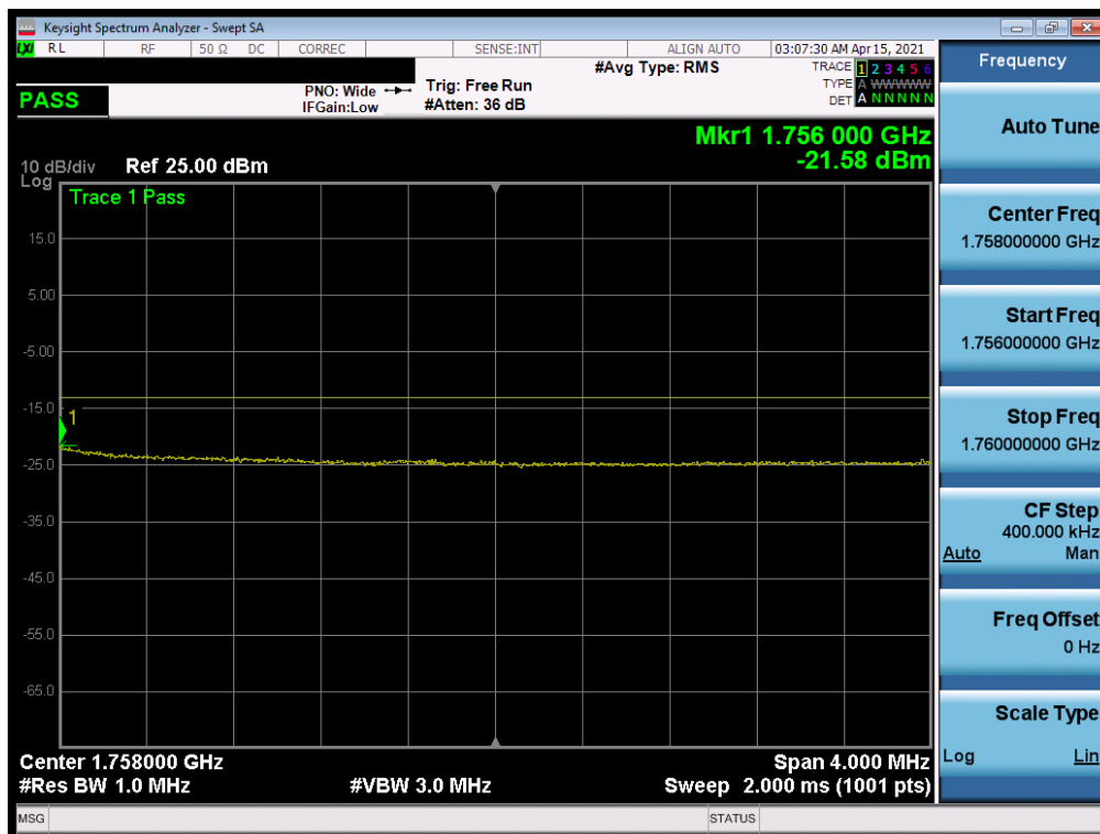
Plot 7-223. Upper Extended Band Edge Plot (LTE Band 4 - 10MHz QPSK – Full RB)
