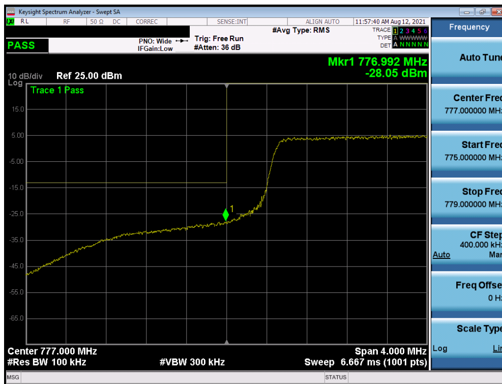
Plot 7-182. Lower Band Edge Plot (LTE Band 13 - 10MHz QPSK – Full RB - Ant I)
