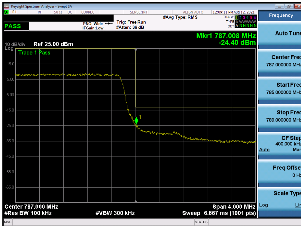
Plot 7-188. Upper Band Edge Plot (LTE Band 13 - 5MHz QPSK - Full RB - Ant I)
