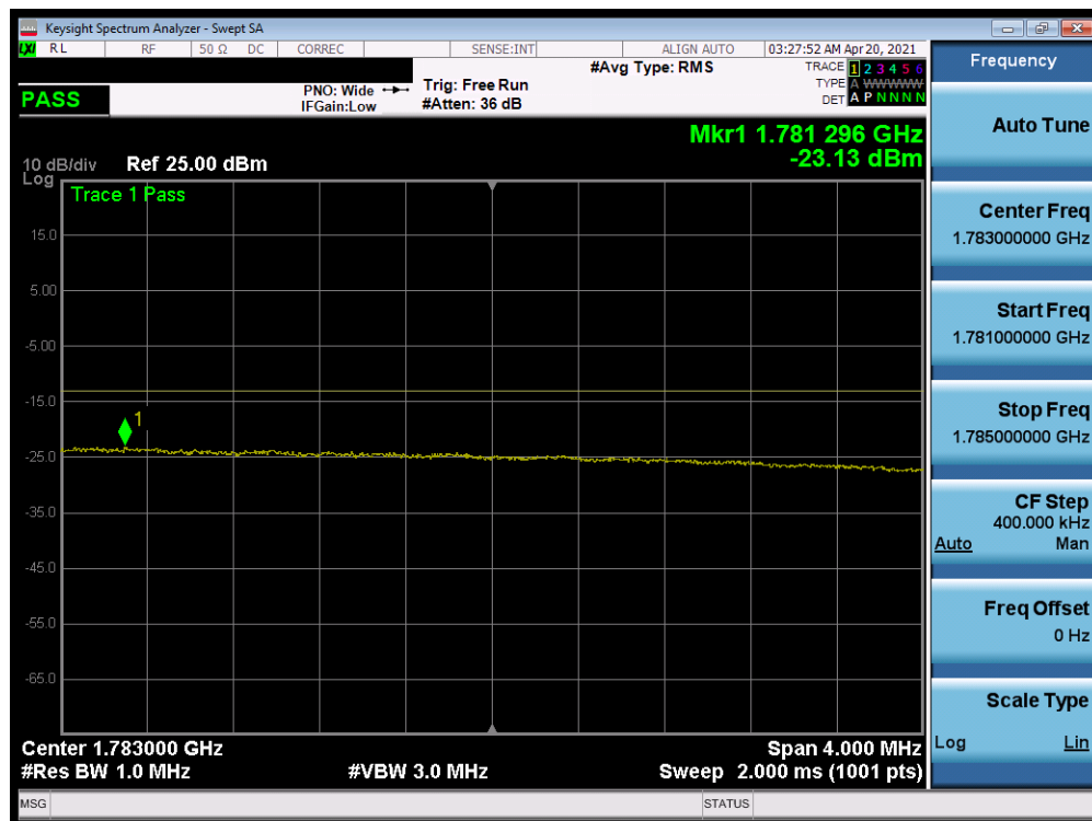
Plot 7-251. Upper Extended Band Edge Plot (NR Band n66 – 30.0MHz - Full RB)
