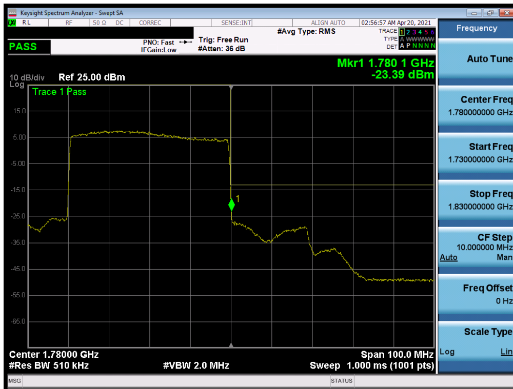
Plot 7-246. Upper Band Edge Plot (NR Band n66 – 40.0MHz - Full RB)
