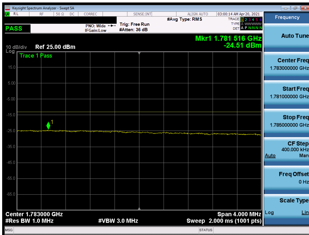
Plot 7-247. Upper Extended Band Edge Plot (NR Band n66 – 40.0MHz - Full RB)
