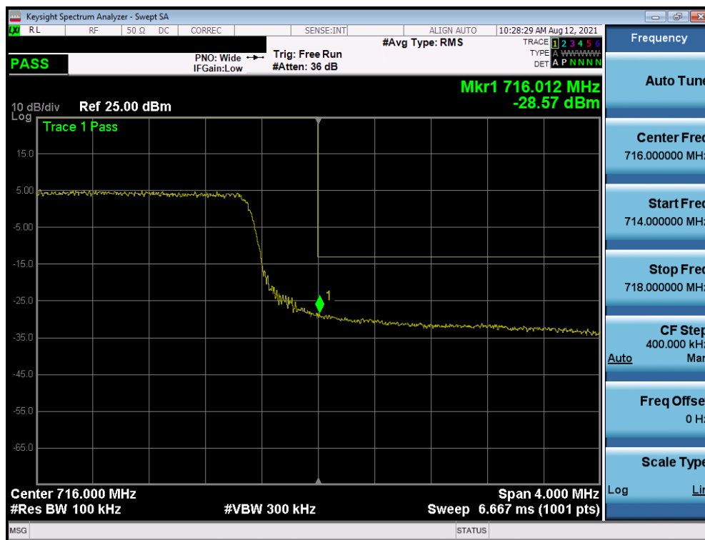
Plot 7-175. Upper Band Edge Plot (LTE Band 12 - 10MHz QPSK – Full RB - Ant I)
