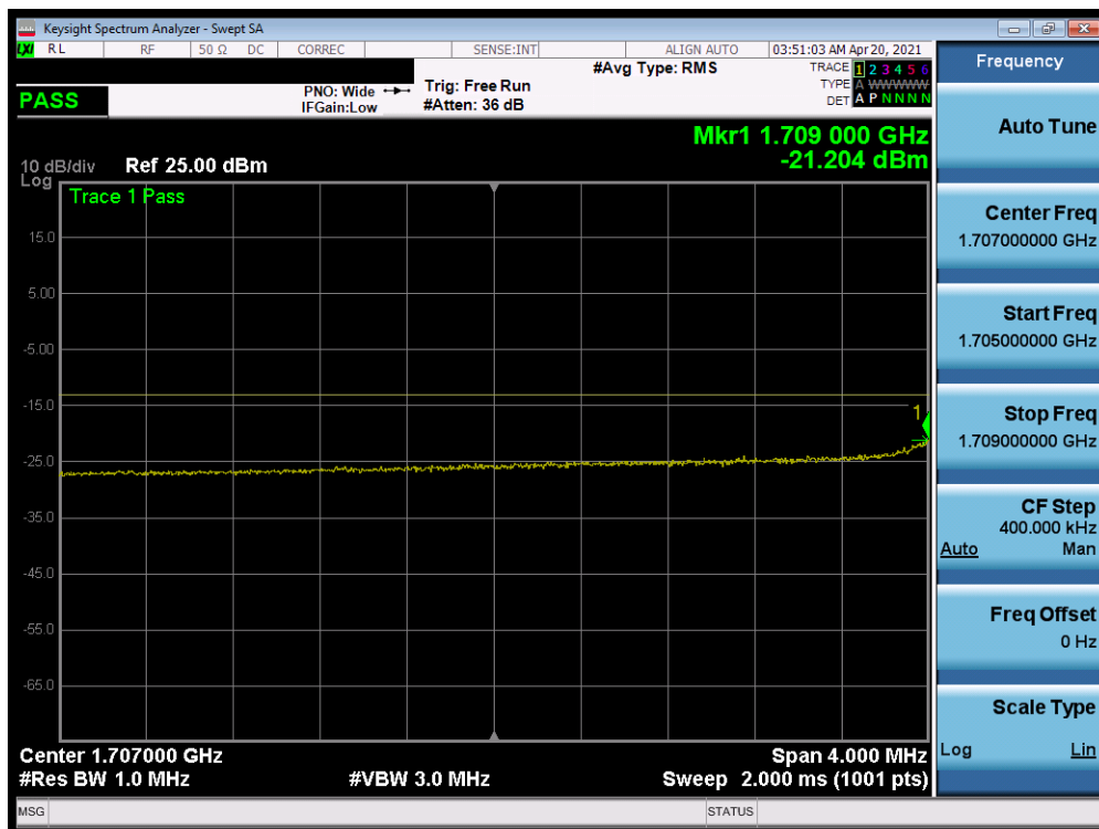
Plot 7-257. Lower Extended Band Edge Plot (NR Band n66 – 15.0MHz - Full RB)
