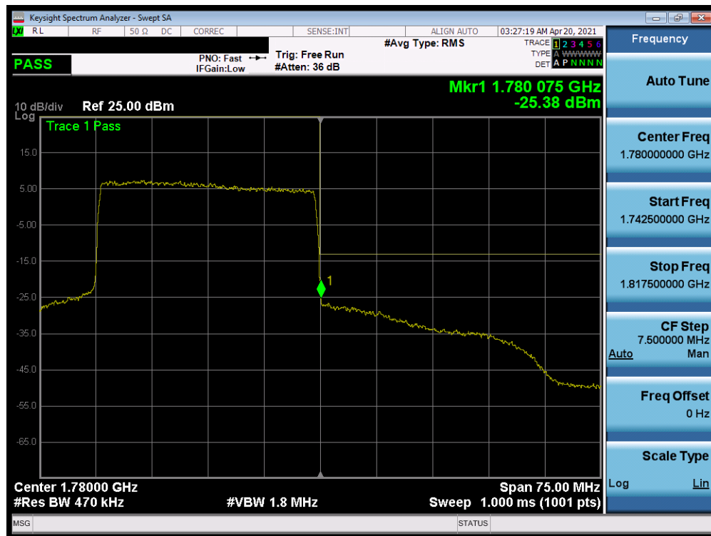
Plot 7-250. Upper Band Edge Plot (NR Band n66 – 30.0MHz - Full RB)
