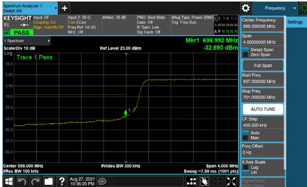
Plot 7-200. Lower Band Edge Plot (NR Band n12 - 10.0MHz - Full RB - Ant I)
