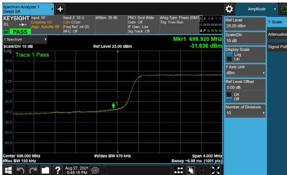
Plot 7-198. Lower Band Edge Plot (NR Band n12 – 15.0MHz - Full RB - Ant I)
