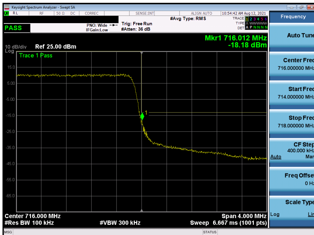
Plot 7-179. Upper Band Edge Plot (LTE Band 12 - 3MHz QPSK - Full RB - Ant I)
