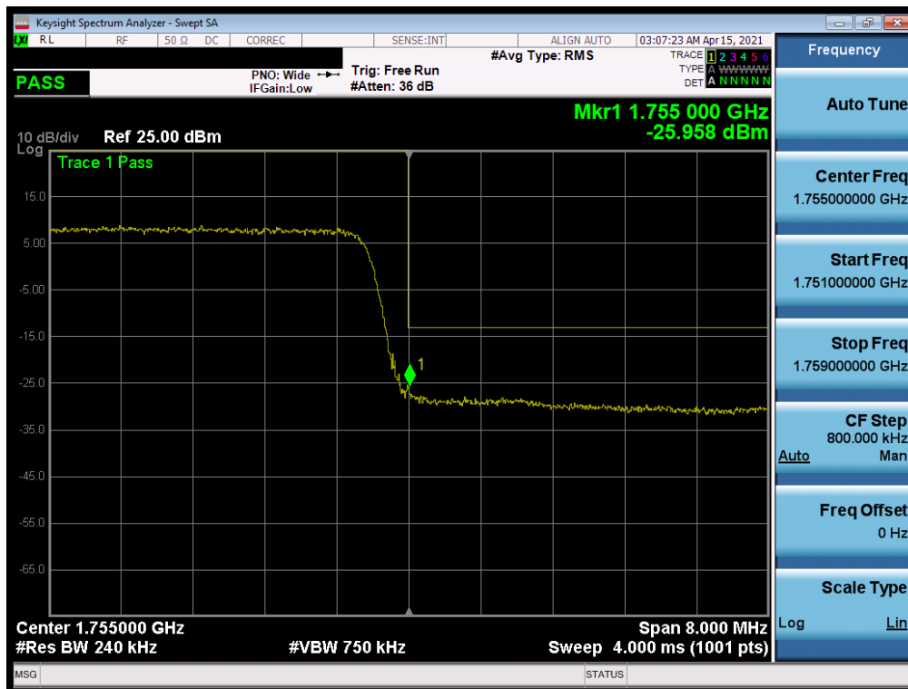
Plot 7-222. Upper Band Edge Plot (LTE Band 4 - 10MHz QPSK – Full RB)
