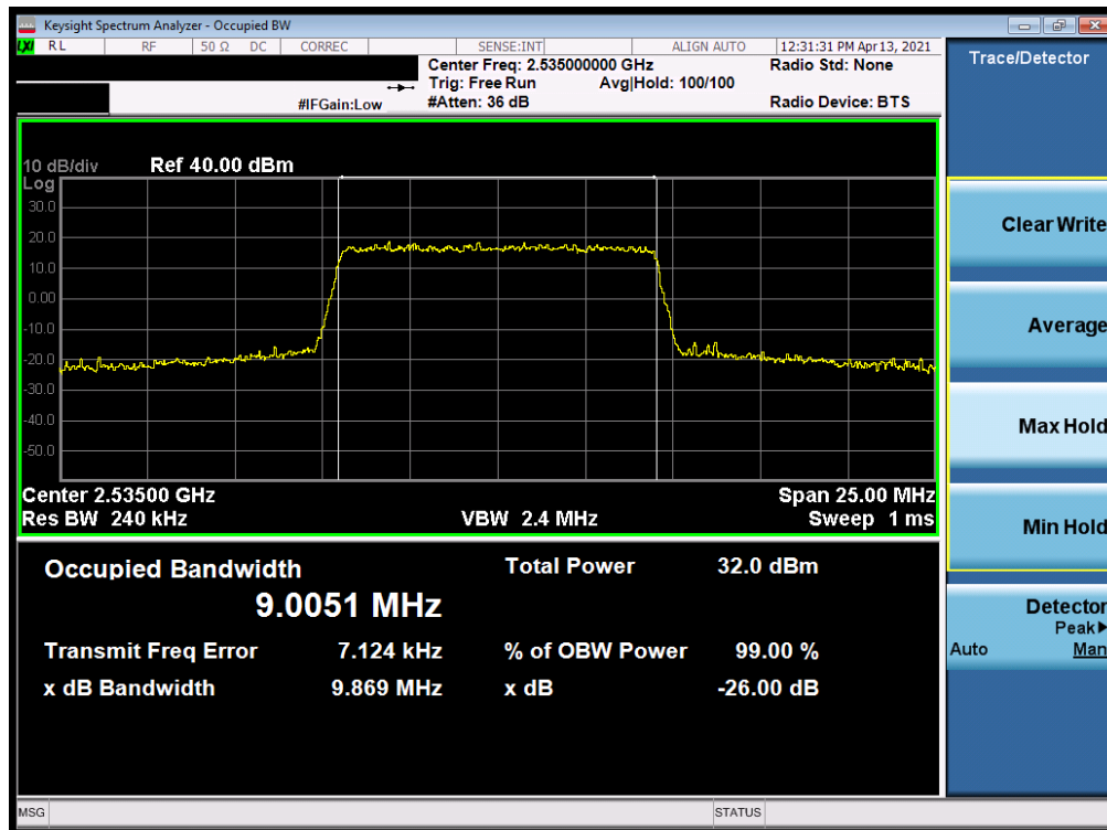
Plot 7-10. Occupied Bandwidth Plot (LTE Band 7 - 10MHz 16-QAM - Full RB)
