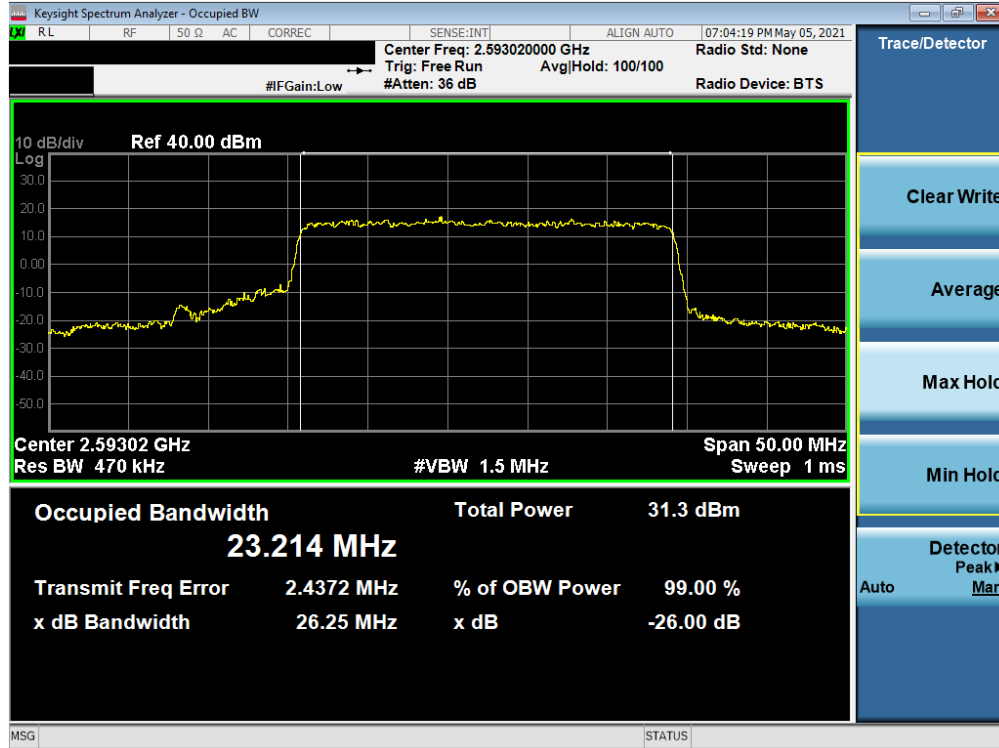
Plot 7-57. Occupied Bandwidth Plot (NR Band n41 - 20MHz QPSK - Full RB)
