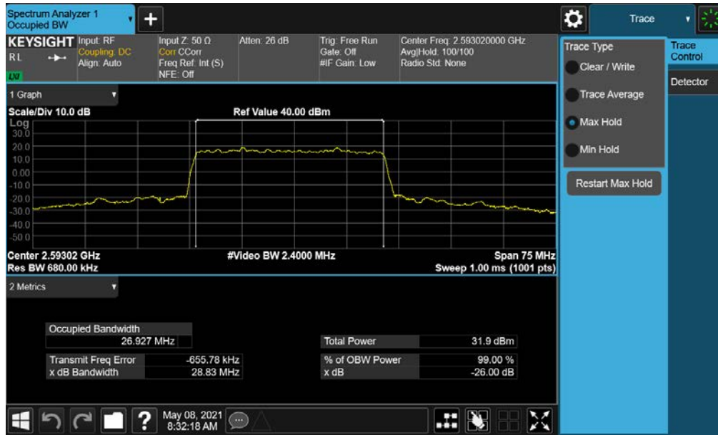
Plot 7-77. Occupied Bandwidth Plot (NR Band n41 - 30MHz \pi/2 BPSK - Full RB)
