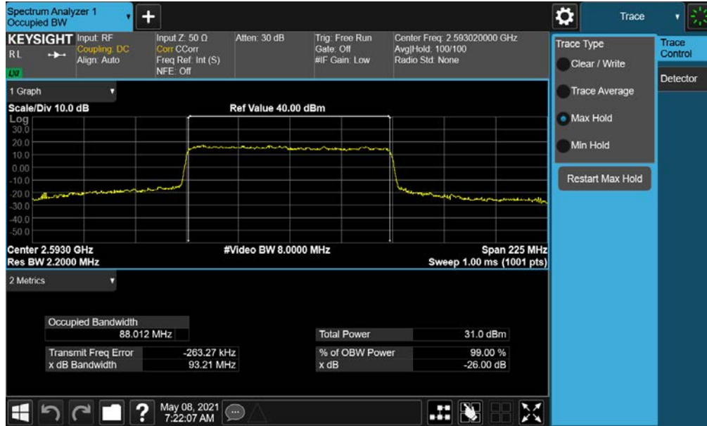
Plot 7-63. Occupied Bandwidth Plot (NR Band n41 - 90MHz QPSK - Full RB)
