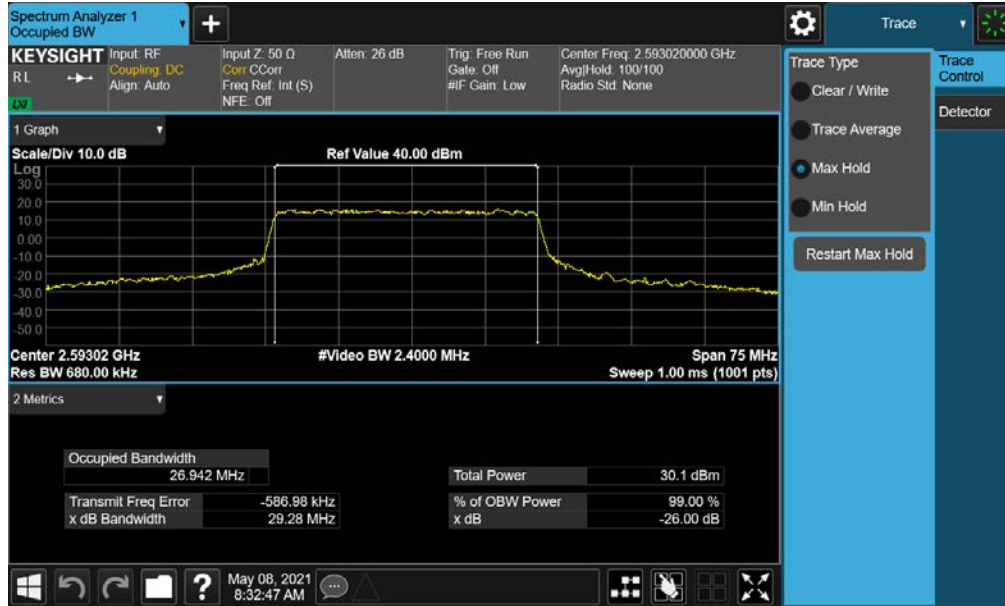
Plot 7-79. Occupied Bandwidth Plot (NR Band n41 - 30MHz 16-QAM - Full RB)
