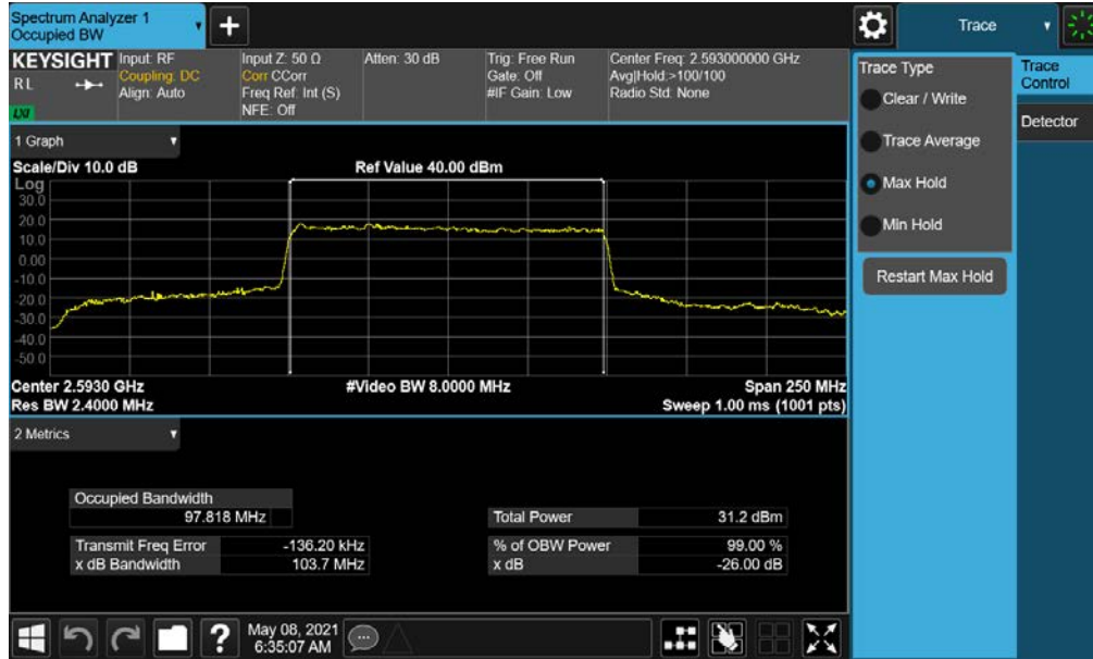
Plot 7-61. Occupied Bandwidth Plot (NR Band n41 - 100MHz 16-QAM - Full RB)
