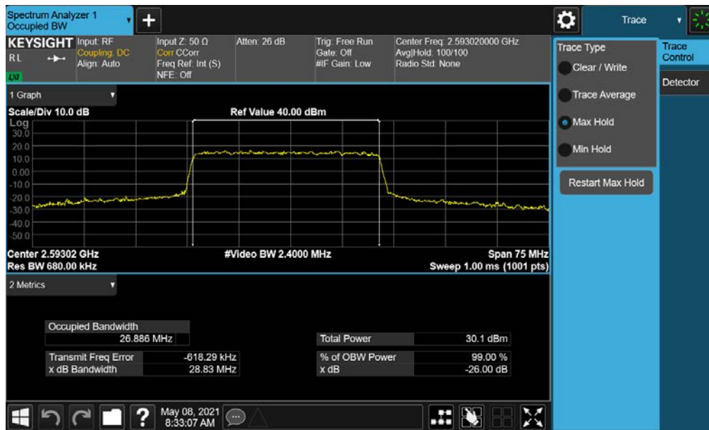
Plot 7-78. Occupied Bandwidth Plot (NR Band n41 - 30MHz QPSK - Full RB)
