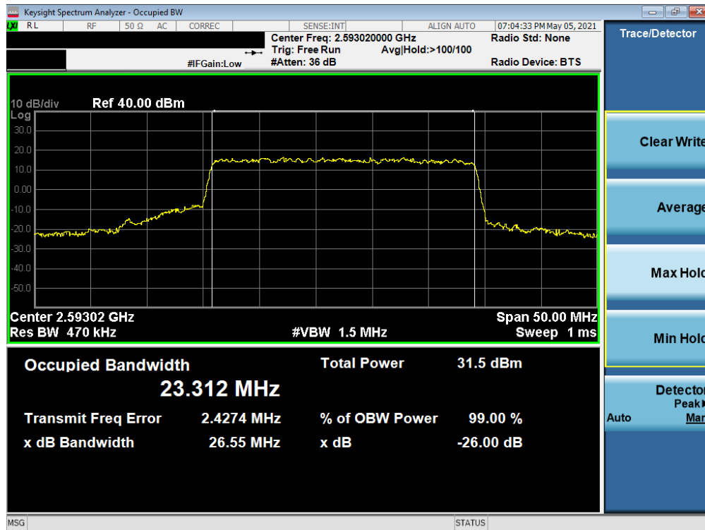
Plot 7-58. Occupied Bandwidth Plot (NR Band n41 - 20MHz 16-QAM - Full RB)
