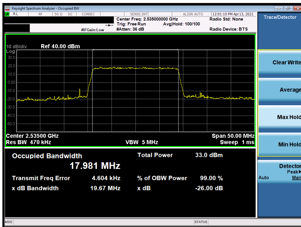
Plot 7-5. Occupied Bandwidth Plot (LTE Band 7 - 20MHz QPSK - Full RB)
