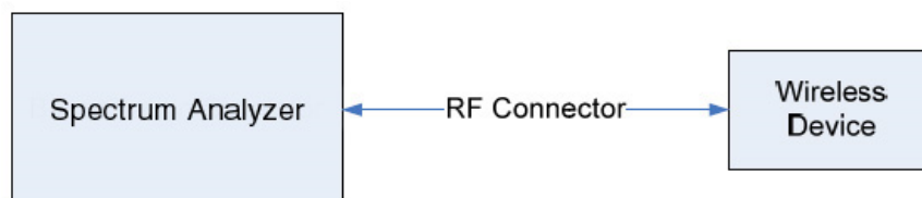
Figure 7-4. Test Instrument & Measurement Setup
