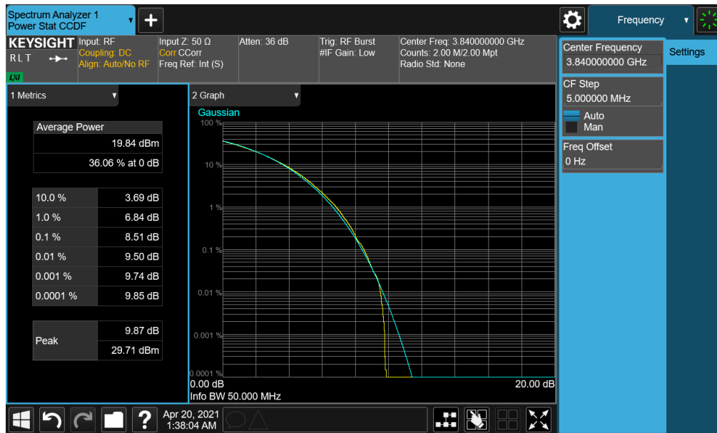
Plot 7-168. PAR Plot (NR Band n77 PC2 - 50MHz CP-OFDM 256-QAM - Full RB)
