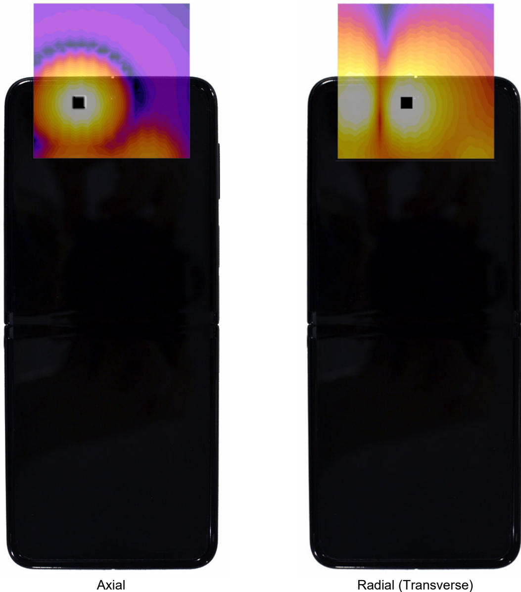
Figure 16-3 T-Coil Scan Overlay Magnetic Field Distributions
