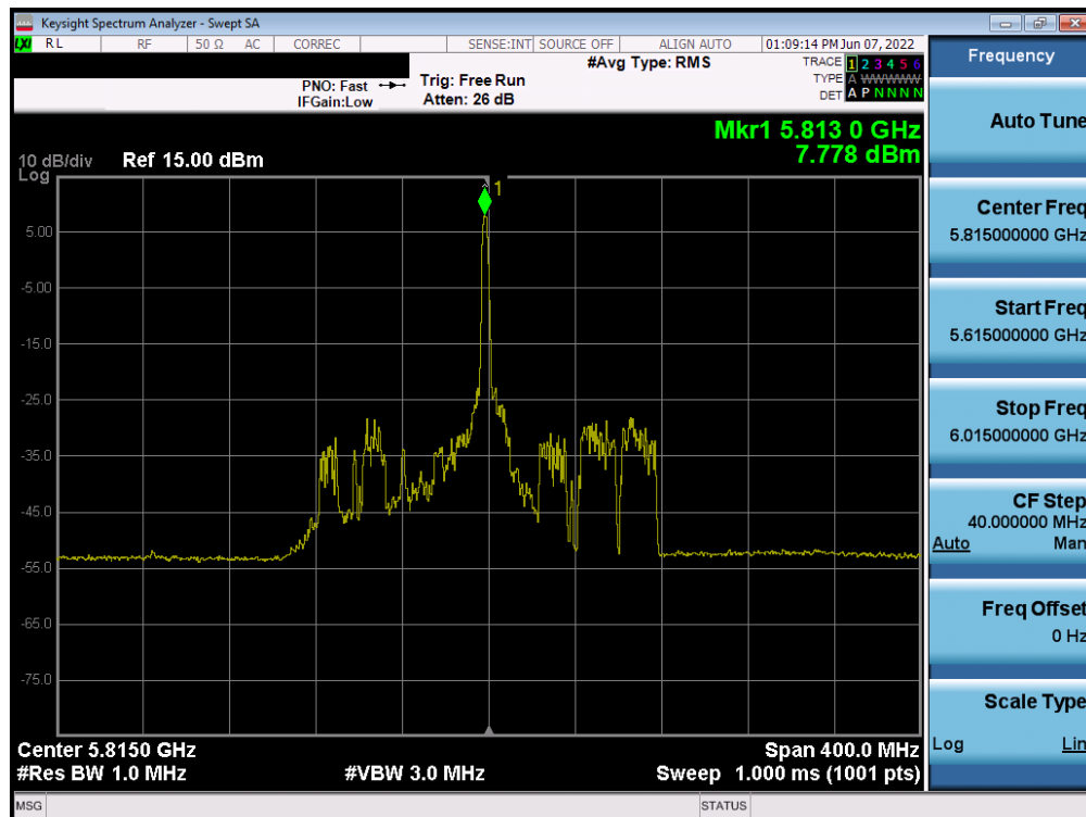
Plot 7-194. Power Spectral Density Plot SISO ANT1 (160MHz BW (L) 802.11ax – 26 Tones (UNII Band 3/4) – Ch. 163)
