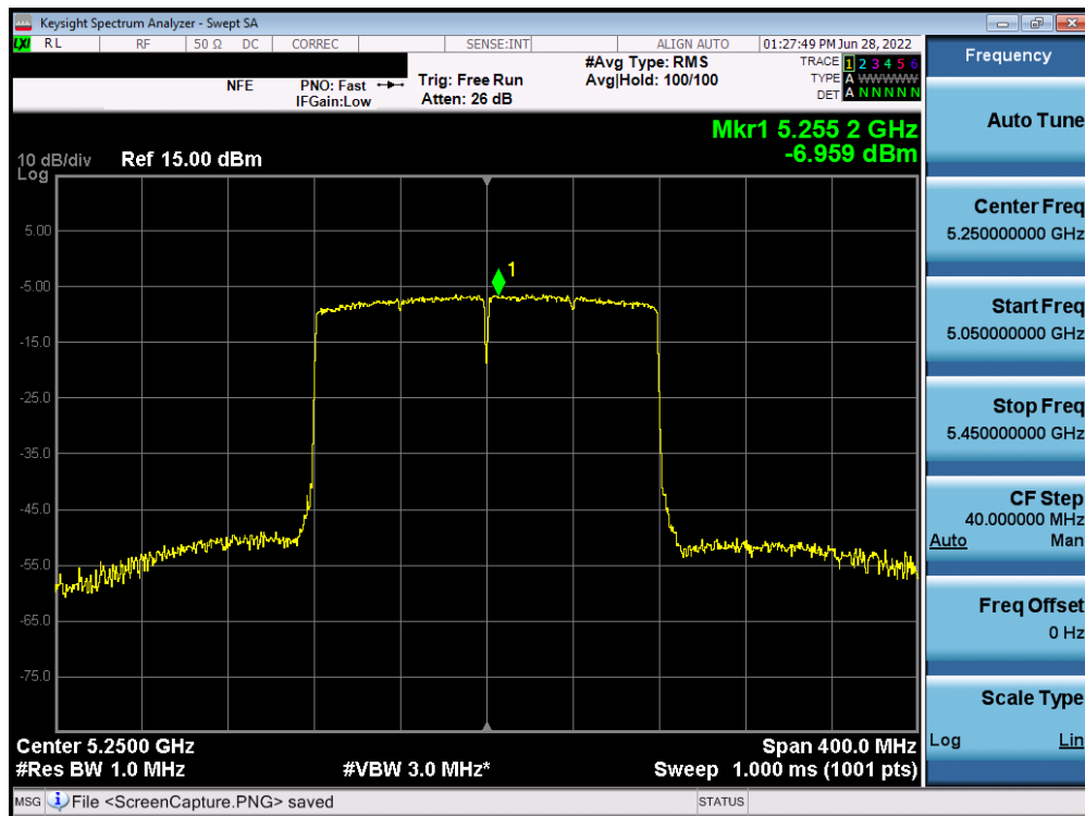
Plot 7-201. Power Spectral Density Plot SISO ANT1 (160MHz BW 802.11ax (UNII Band 1/2A) – Ch. 50)
