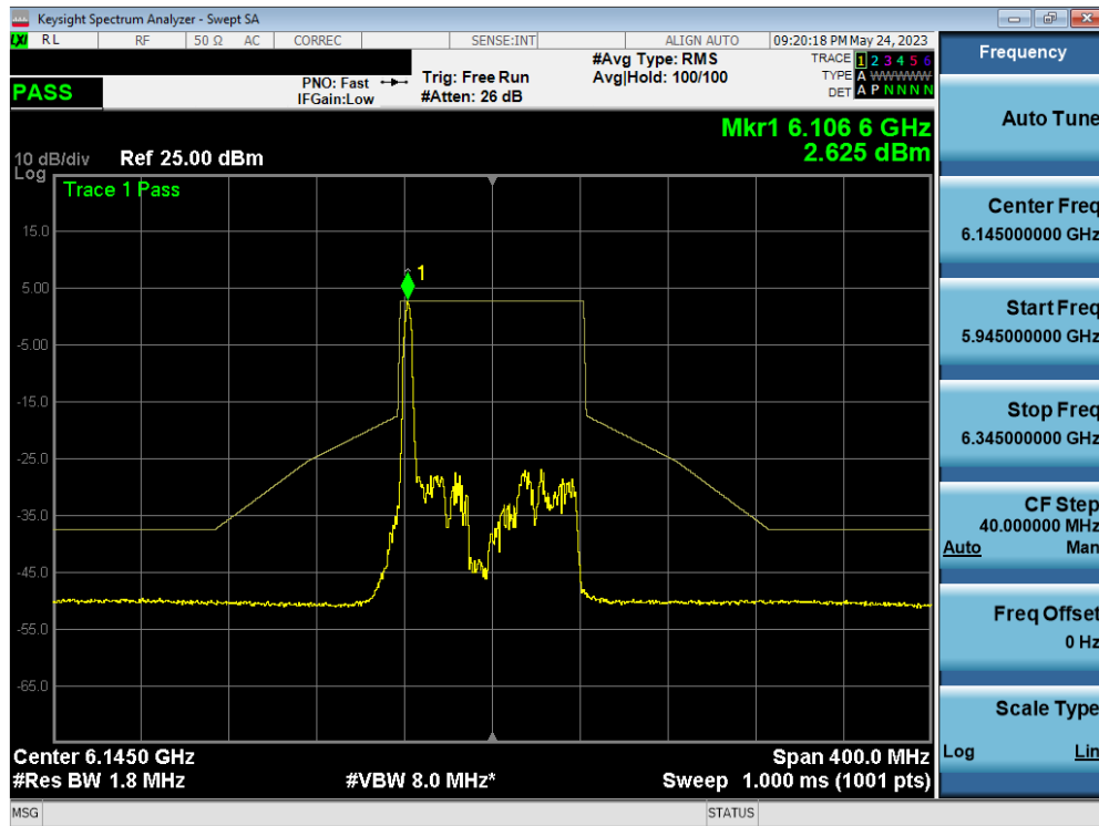
Plot 7-163. In-Band Emission Plot MIMO ANT2 (80MHz BW 802.11ax (26 Tones) (UNII Band 5) – Ch. 39)
