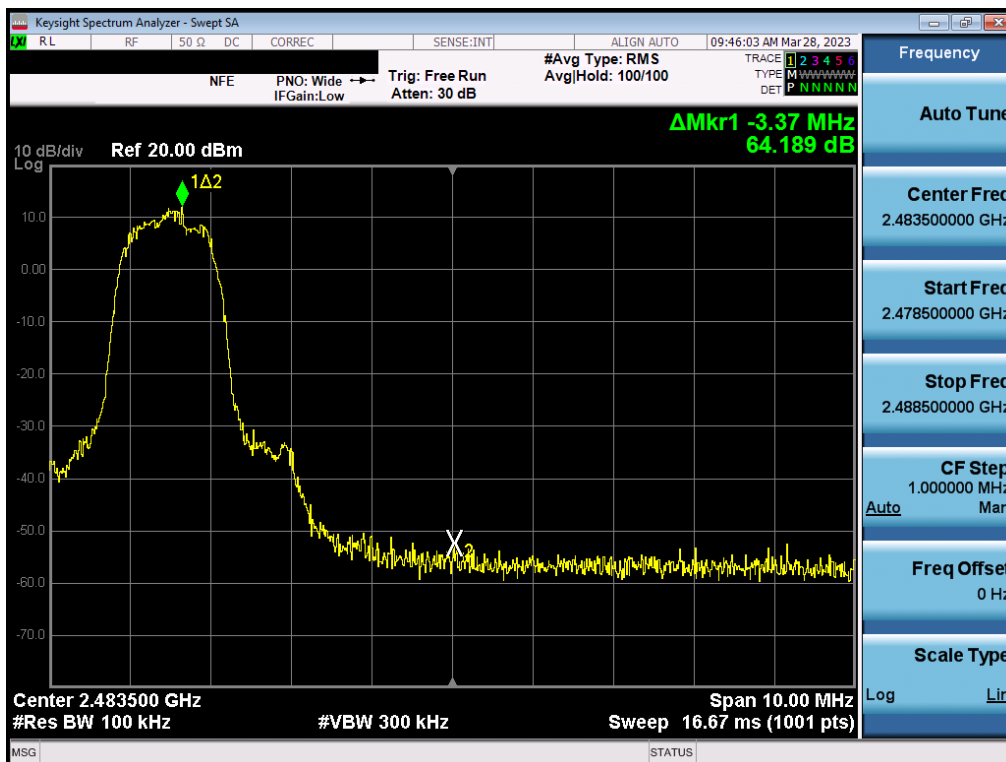
Plot 7-60. Band Edge Plot (Bluetooth with Hopping Disabled, 3 Mbps – Ch. 78) – ANT2
