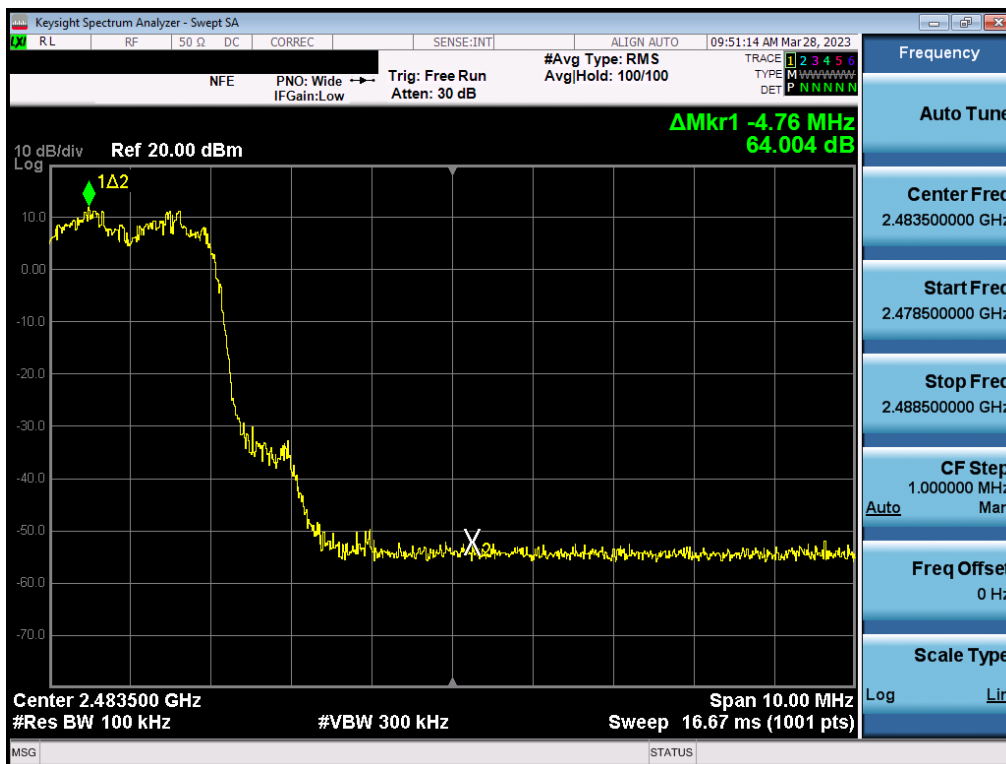
Plot 7-62. Band Edge Plot (Bluetooth with Hopping Enabled, 3 Mbps – Ch. 78) – ANT2
