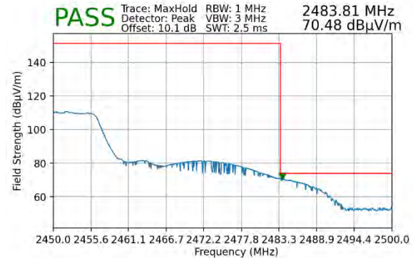
Plot 7-100. Radiated Restricted Upper Band Edge Measurement MIMO (Peak – 106 Tones)
