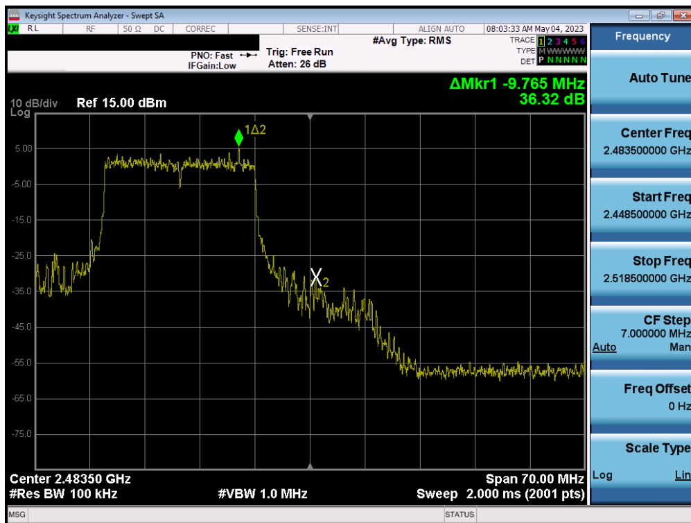
Plot 7-53. Band Edge Plot MIMO ANT2 (802.11ax OFDMA - 242 Tones - Ch. 12)
