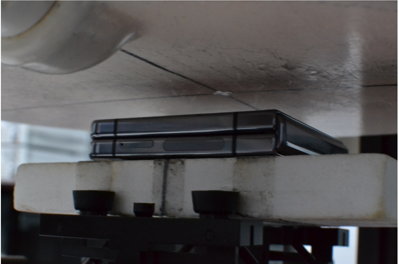
Figure F-8 SAR Test Setup Photo– Body-worn, Back Side, 15 mm, Closed
