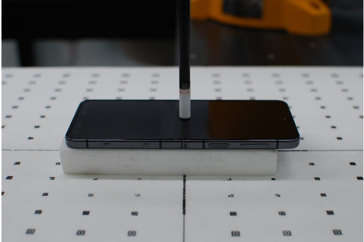
Figure F-17 Near Field Power Density Test Setup Photo – Front Side at 2 mm, Open
