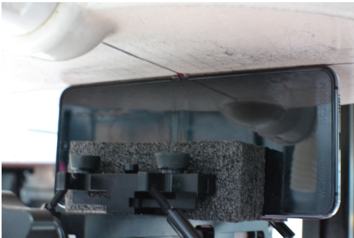
Figure F-12 SAR Test Setup Photo– Phablet, Right Edge, 0 mm, Open
