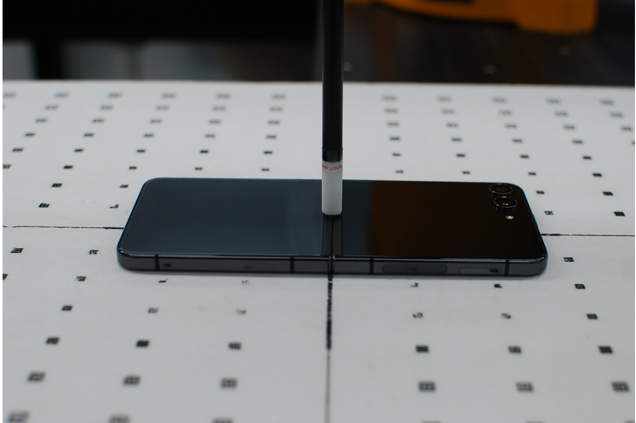
Figure F-15 Near Field Power Density Test Setup Photo – Back Side at 2 mm, Open
