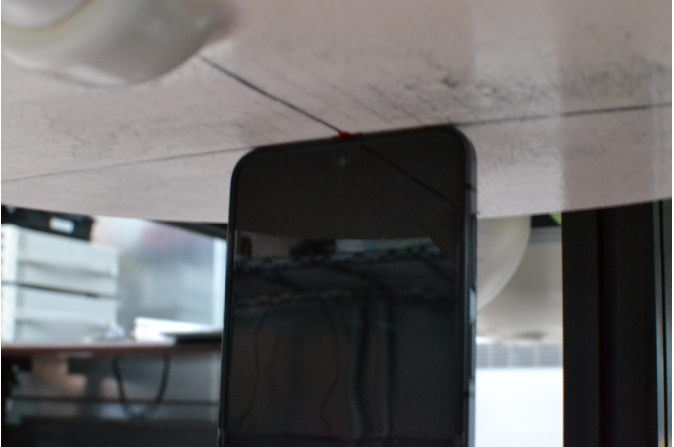
Figure F-11 SAR Test Setup Photo– Phablet, Top Edge, 0 mm, Open
