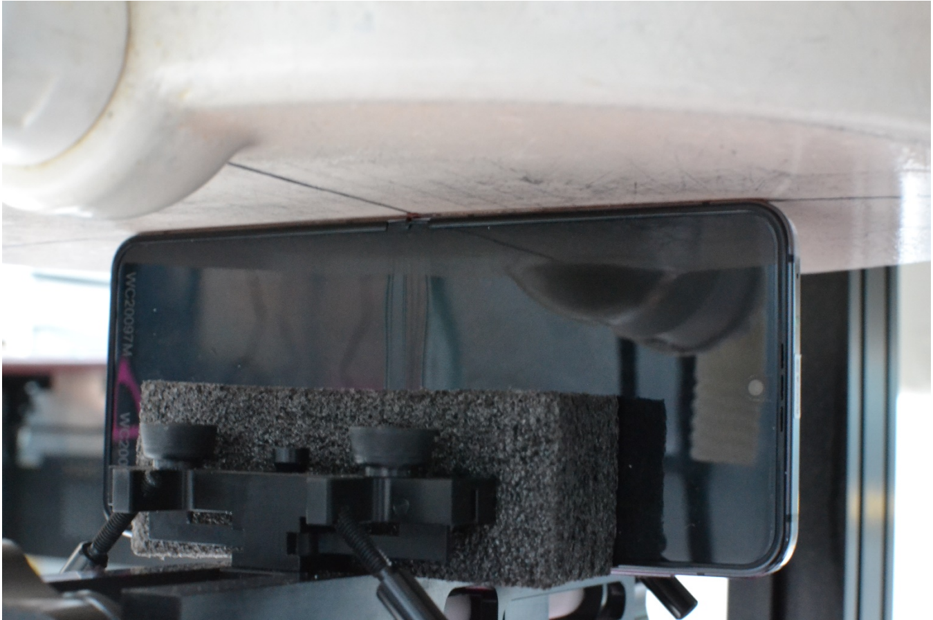
Figure F-13 SAR Test Setup Photo– Phablet, Left Edge, 0 mm, Open
