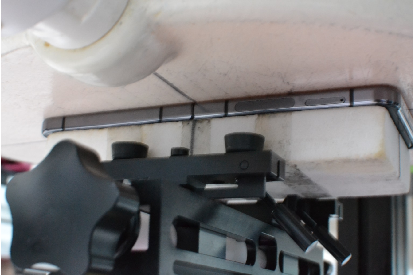
Figure F-9 SAR Test Setup Photo– Phablet, Back Side, 0 mm, Open
