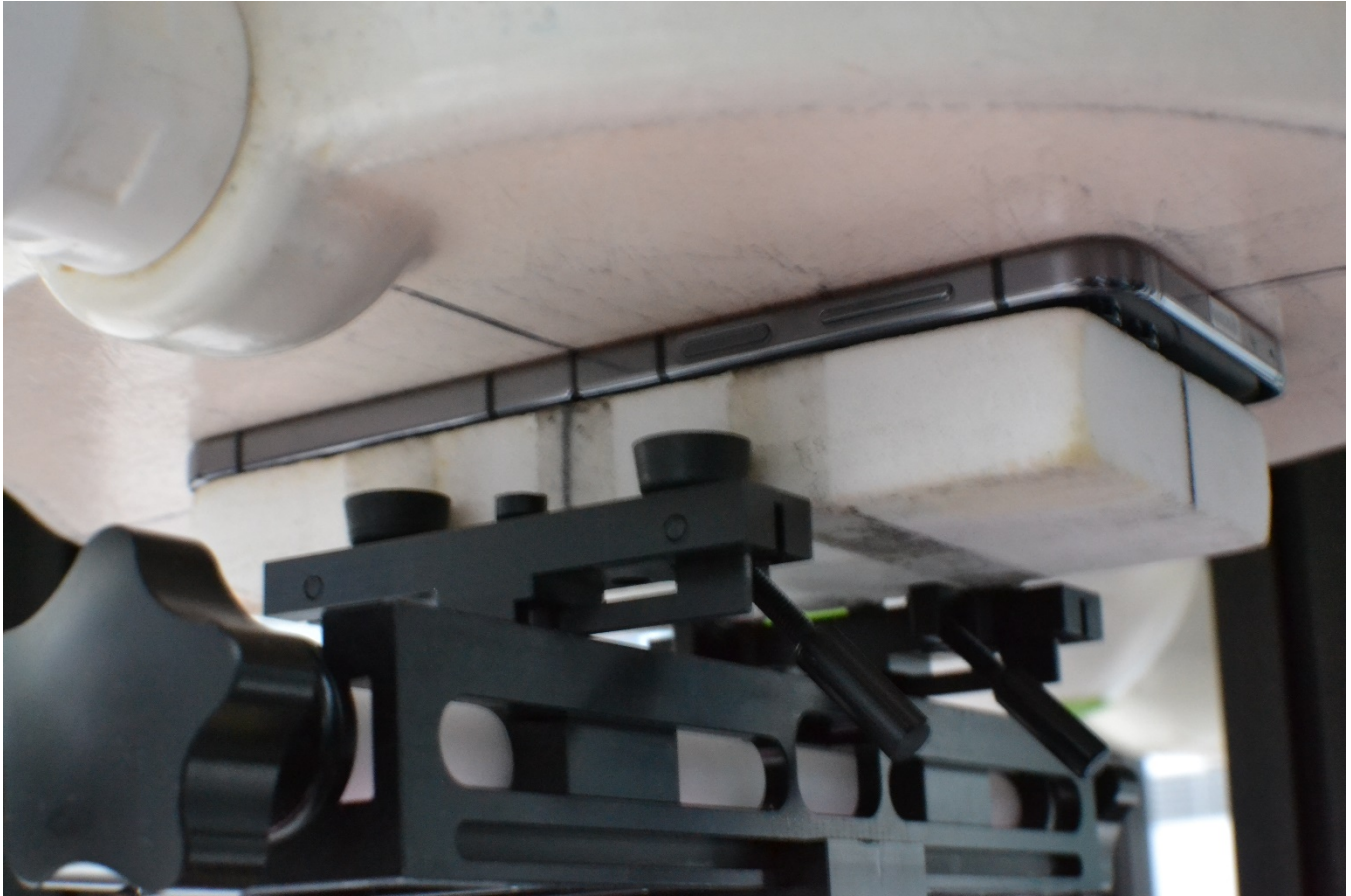
Figure F-10 SAR Test Setup Photo– Phablet, Front Side, 0 mm, Open
