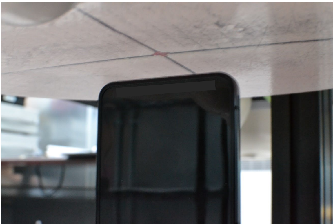
SAR Test Setup Photo 10 – Hotspot, Bottom Edge at 10 mm
