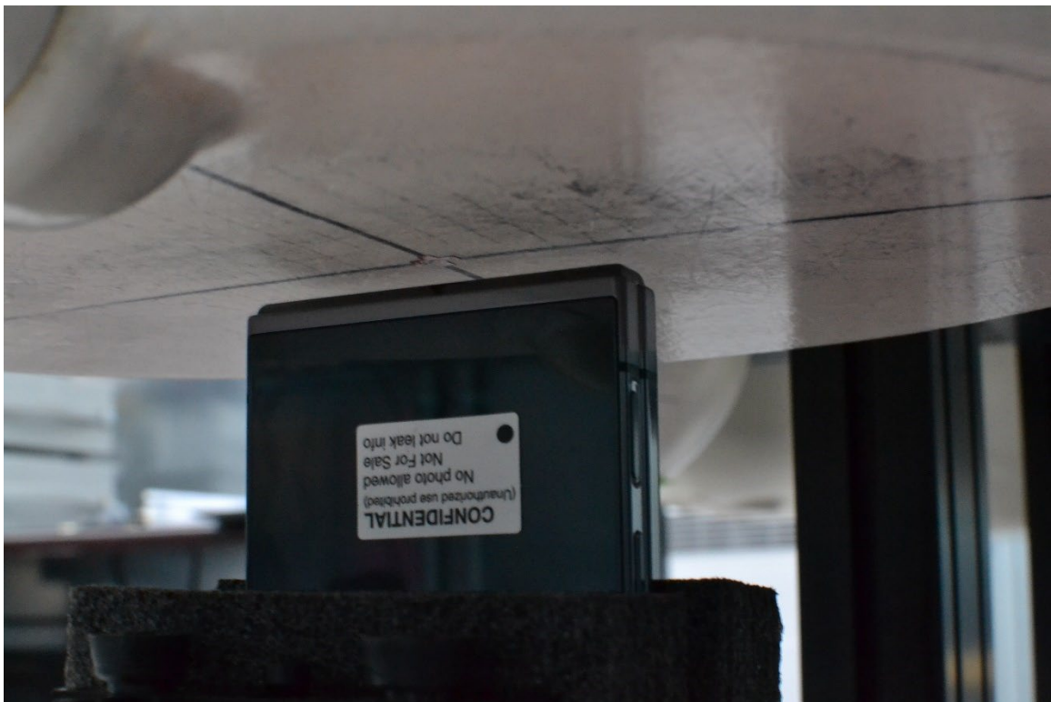
SAR Test Setup Photo 22 – Closed Hotspot, Top Edge at 5 mm
