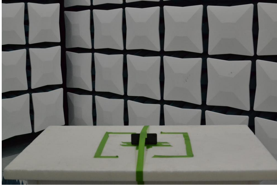
Figure 17. Test Setup – Y Position – 30MHz-1GHz – Open
