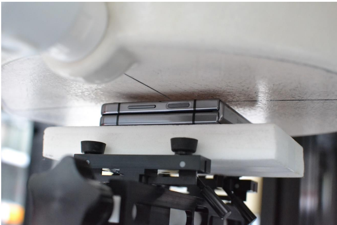
SAR Test Setup Photo 20 – Closed Hotspot, Front Side at 5 mm
