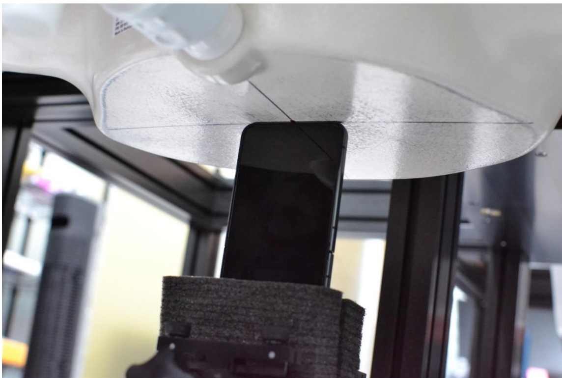
SAR Test Setup Photo 11 – Phablet, Bottom Edge at 0 mm
