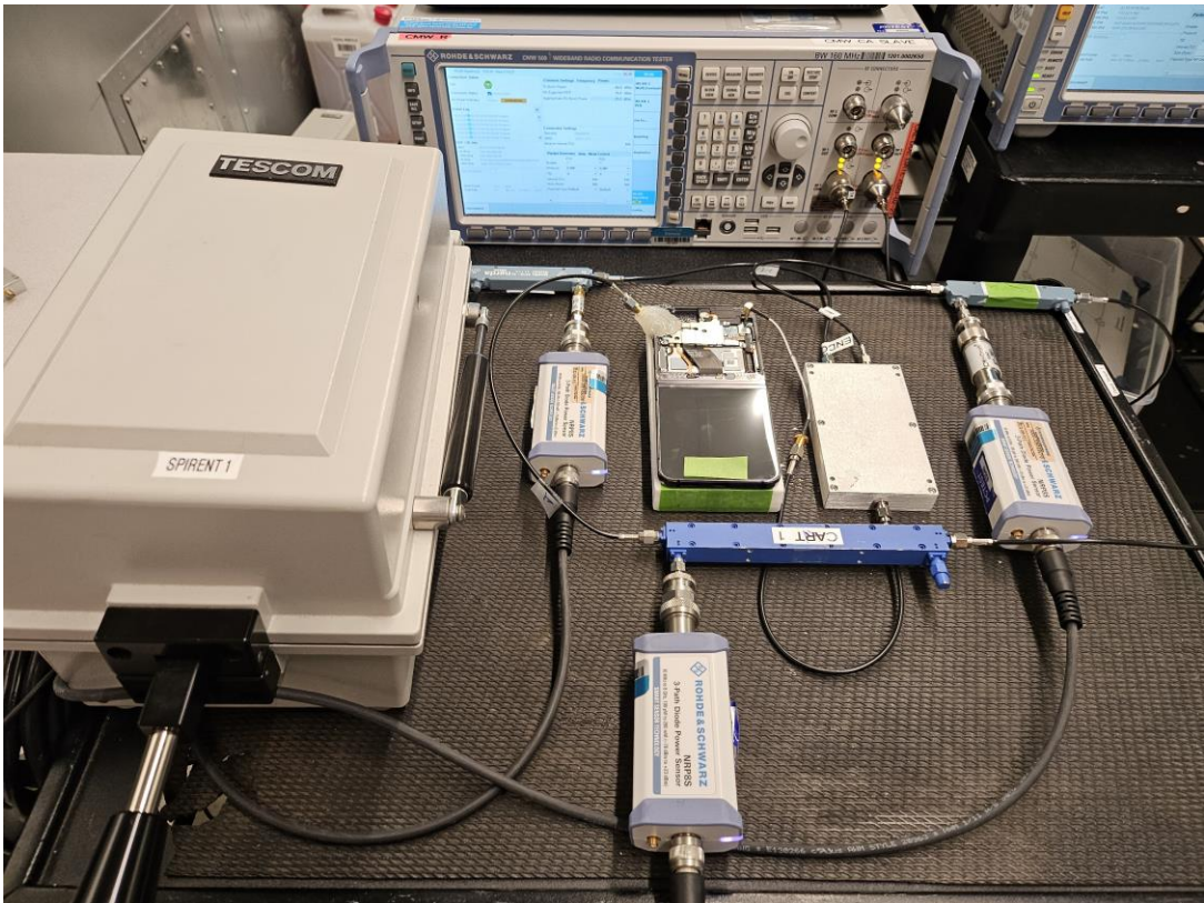
Test Setup Photo 9 – Conducted Test Setup (Figure 6-1f)
