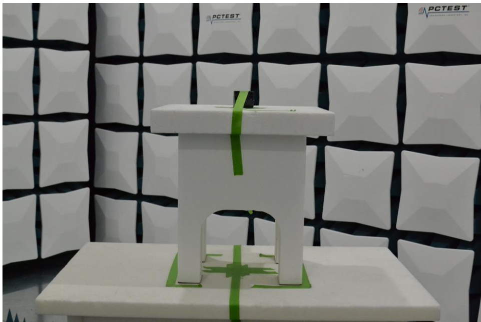
Figure 10. Test Setup – Y Position – 1GHz-18GHz – Closed
