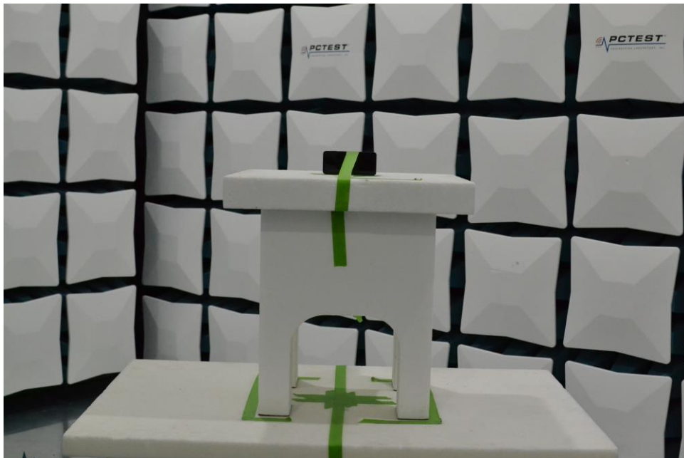
Figure 2. Test Setup – Y Position – 1GHz-18GHz – Open
