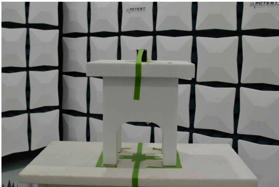
Figure 8. Test Setup – Z Position – 1GHz-18GHz – Half
