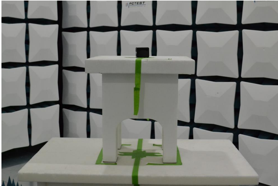
Figure 7. Test Setup – Y Position – 1GHz-18GHz – Half
