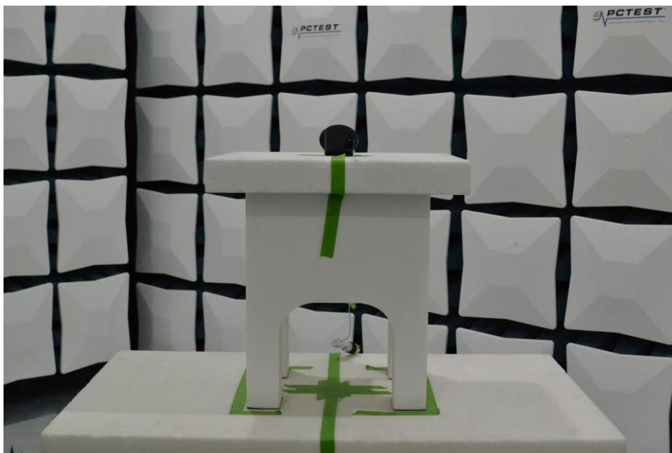
Figure 12. Test Setup – WCP Position – 1GHz-18GHz – Closed
