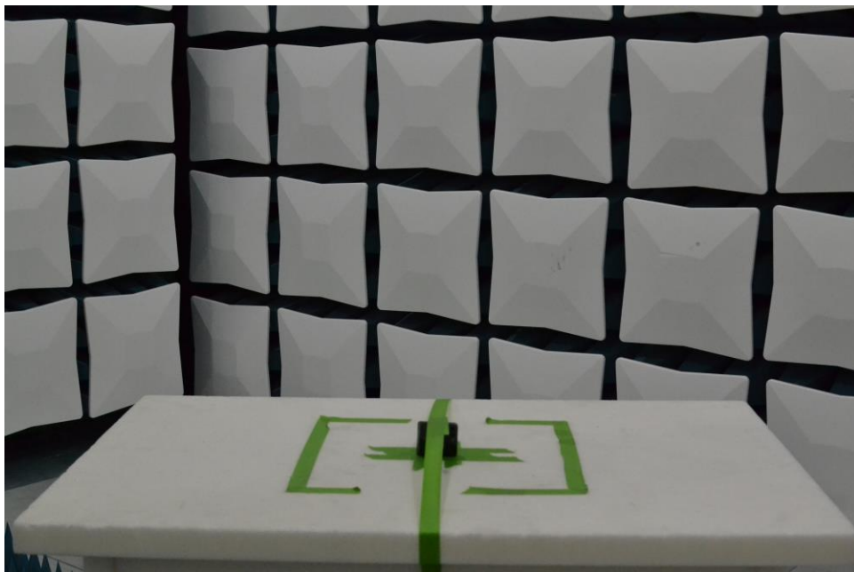
Figure 22. Test Setup – Y Position – 30MHz-1GHz – Closed
