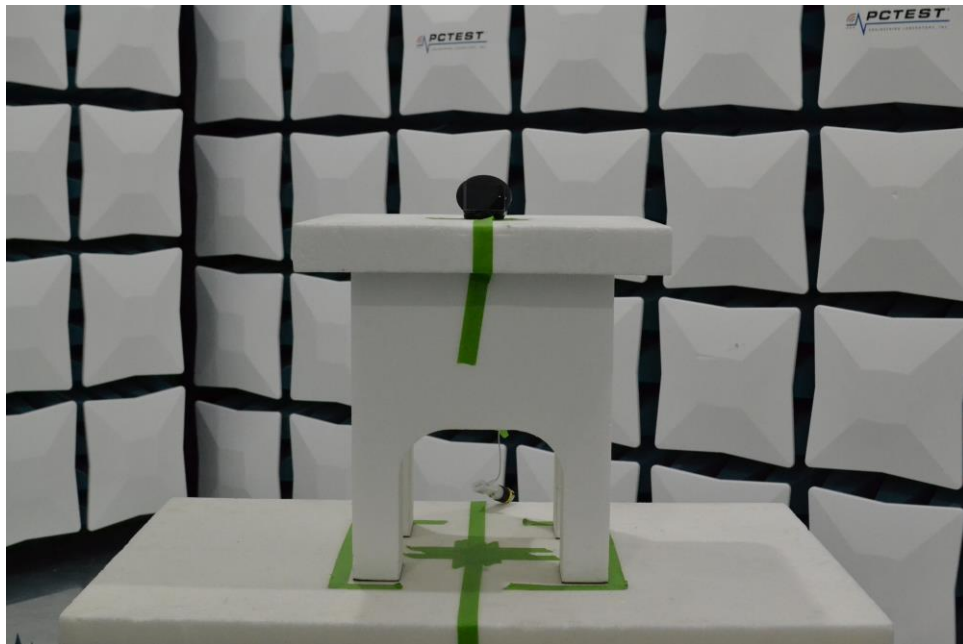
Figure 16. Test Setup – WCP Position – 1GHz-18GHz – Closed
