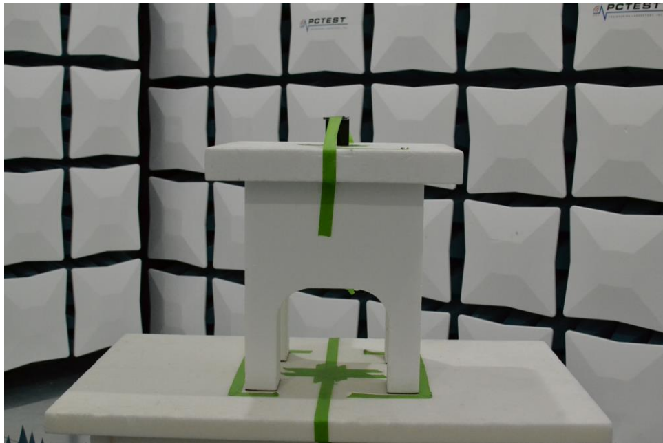
Figure 12. Test Setup – Z Position – 1GHz-18GHz – Half
