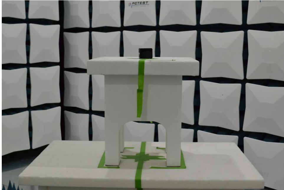
Figure 11. Test Setup – Y Position – 1GHz-18GHz – Half
