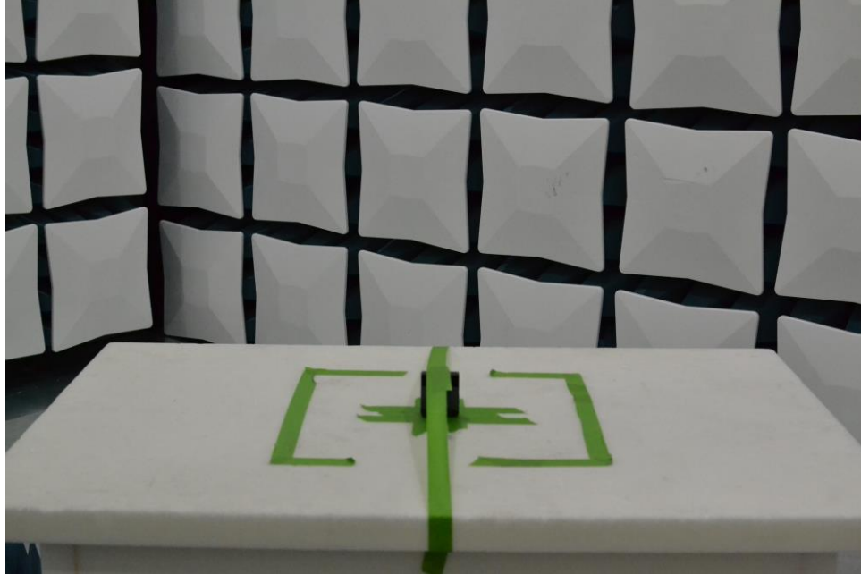
Figure 27. Test Setup – Z Position – 30MHz-1GHz – Closed
