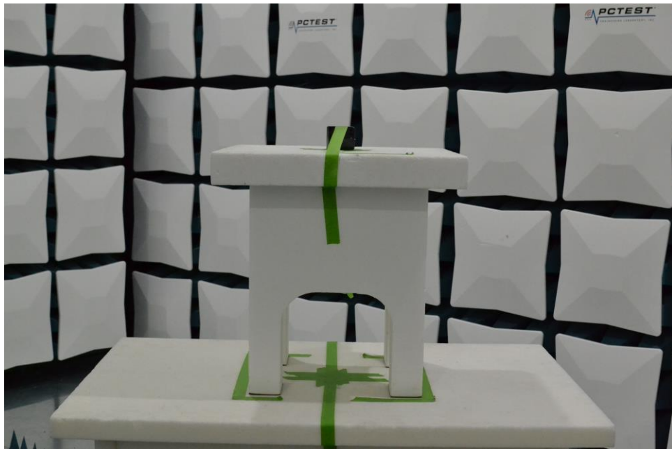
Figure 14. Test Setup – Y Position – 1GHz-18GHz – Closed
