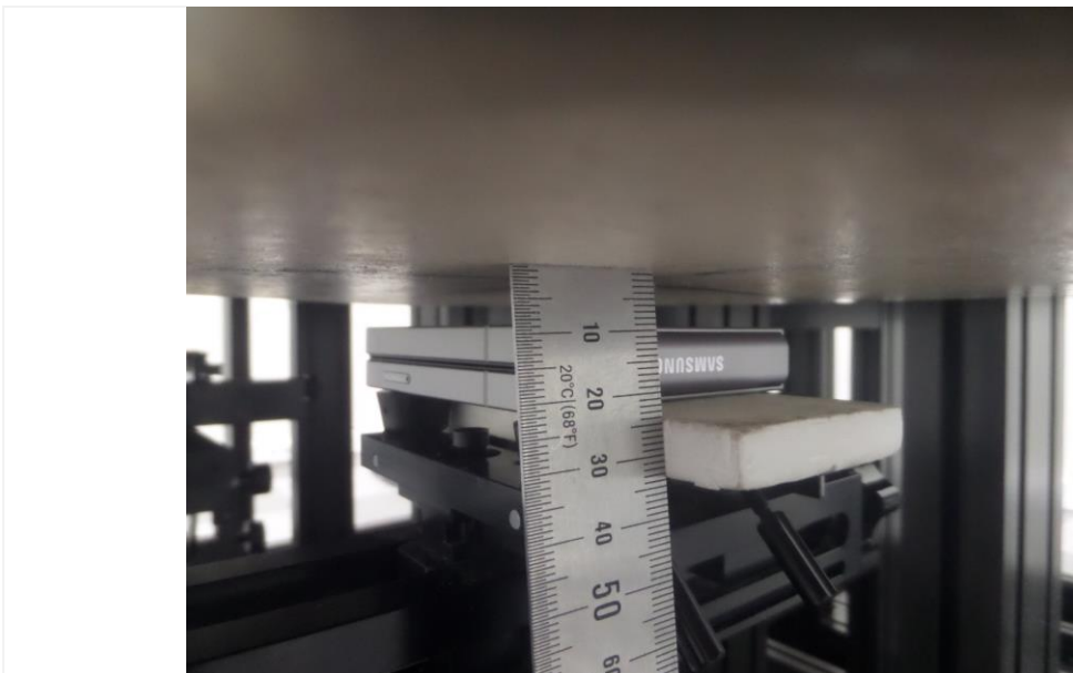
Distance of 10 mm from the EUT
