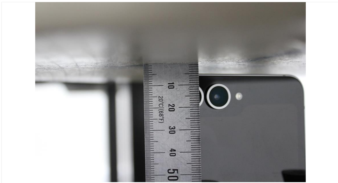
Distance of 5 mm from the EUT
