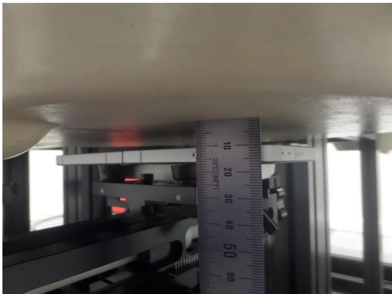
Distance of 10 mm from the EUT
