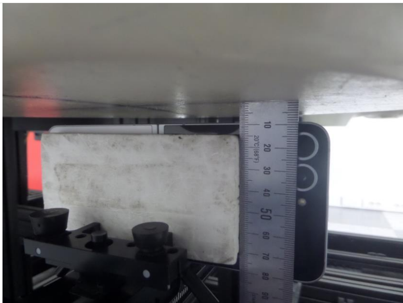
Distance of 10 mm from the EUT
