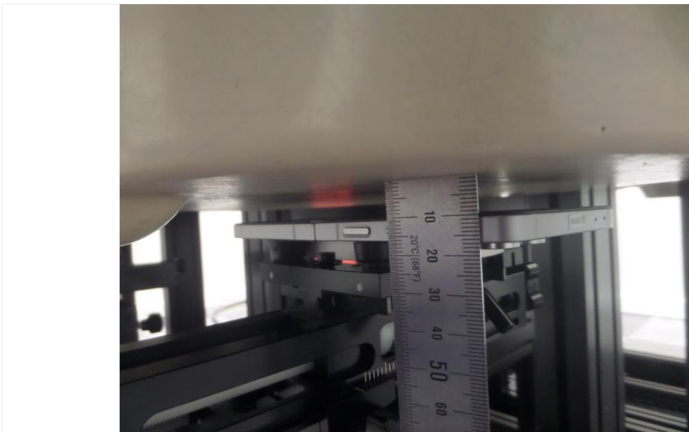
Distance of 10 mm from the EUT
