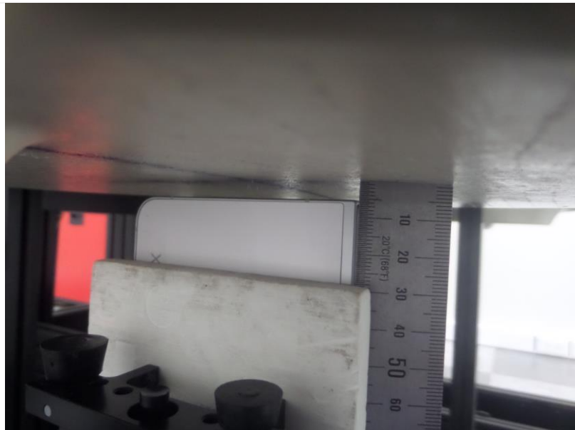
Distance of 5 mm from the EUT
