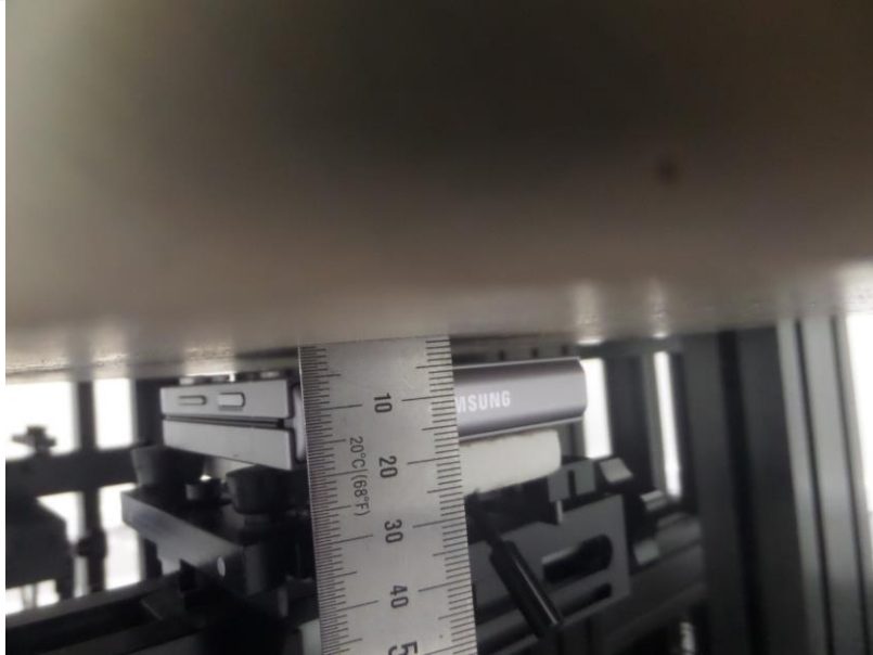
Distance of 5 mm from the EUT
