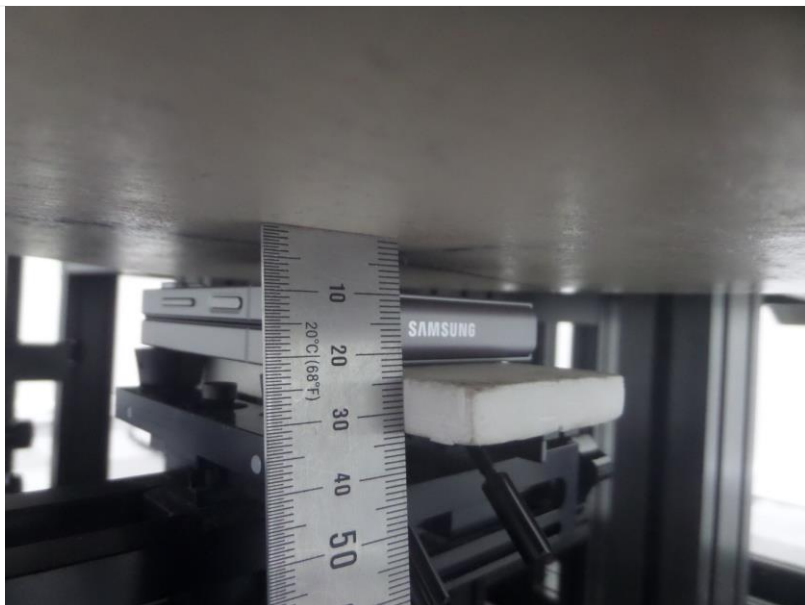
Distance of 10 mm from the EUT
