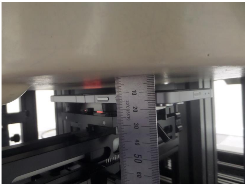
Distance of 10 mm from the EUT
