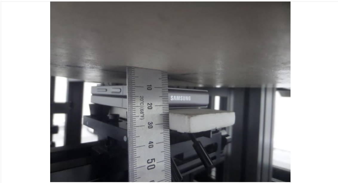
Distance of 10 mm from the EUT
