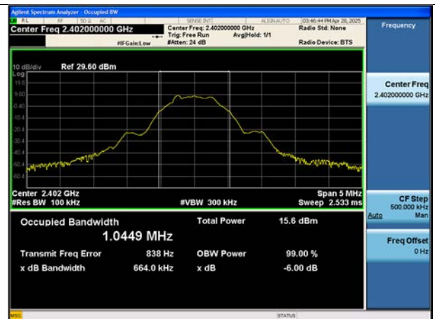
500k Bit/s 255 Byte (Low-CH 37)
