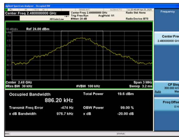
Dual ANT. 1 8DPSK 20 dB BW &amp; 99% OBW (Ch. 0)
