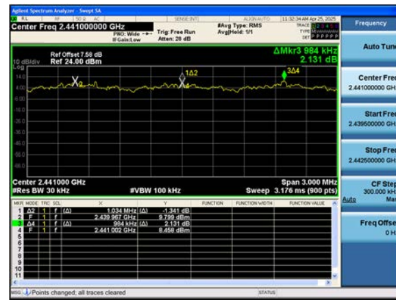
Dual ANT. 1 \pi/4 DQPSK : Channel Separation
