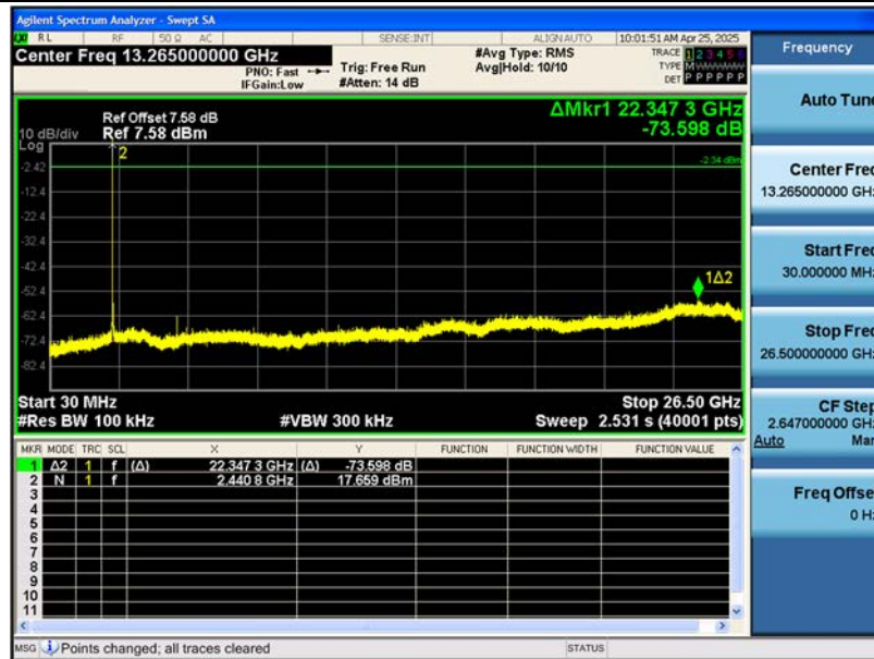
Spurious Emission (30 MHz - 26.50 GHz)Ant.2, GFSK Ch. 39
