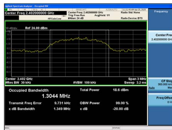
Dual ANT. 1 \pi/4 DQPSK 20 dB BW & 99% OBW (Ch. 0)
