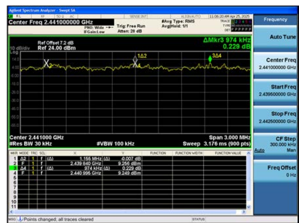
Dual ANT. 2 \pi/4 DQPSK : Channel Separation
