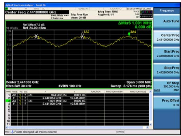
Dual ANT. 2 8DPSK : Channel Separation
