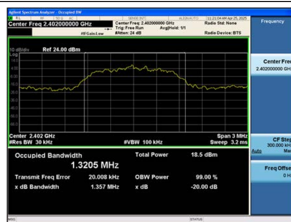
Dual ANT. 1 \pi/4 DQPSK 20 dB BW & 99% OBW (Ch. 0)
