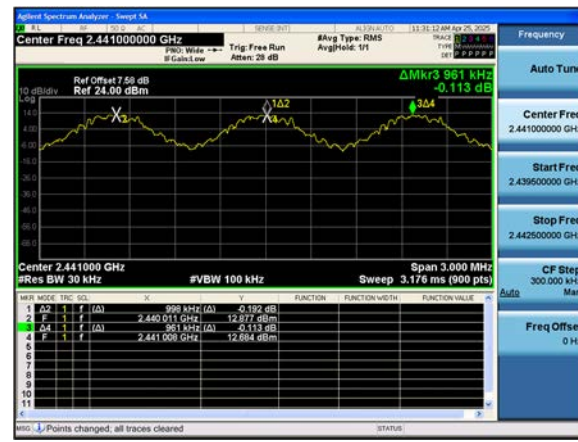
Dual ANT. 1 8DPSK : Channel Separation
