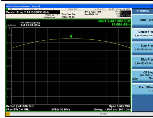
Dual ANT.1 \pi /4DQPSK : Peak Power (Ch. 39)
