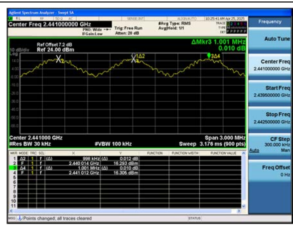
ANT. 2 8DPSK : Channel Separation
