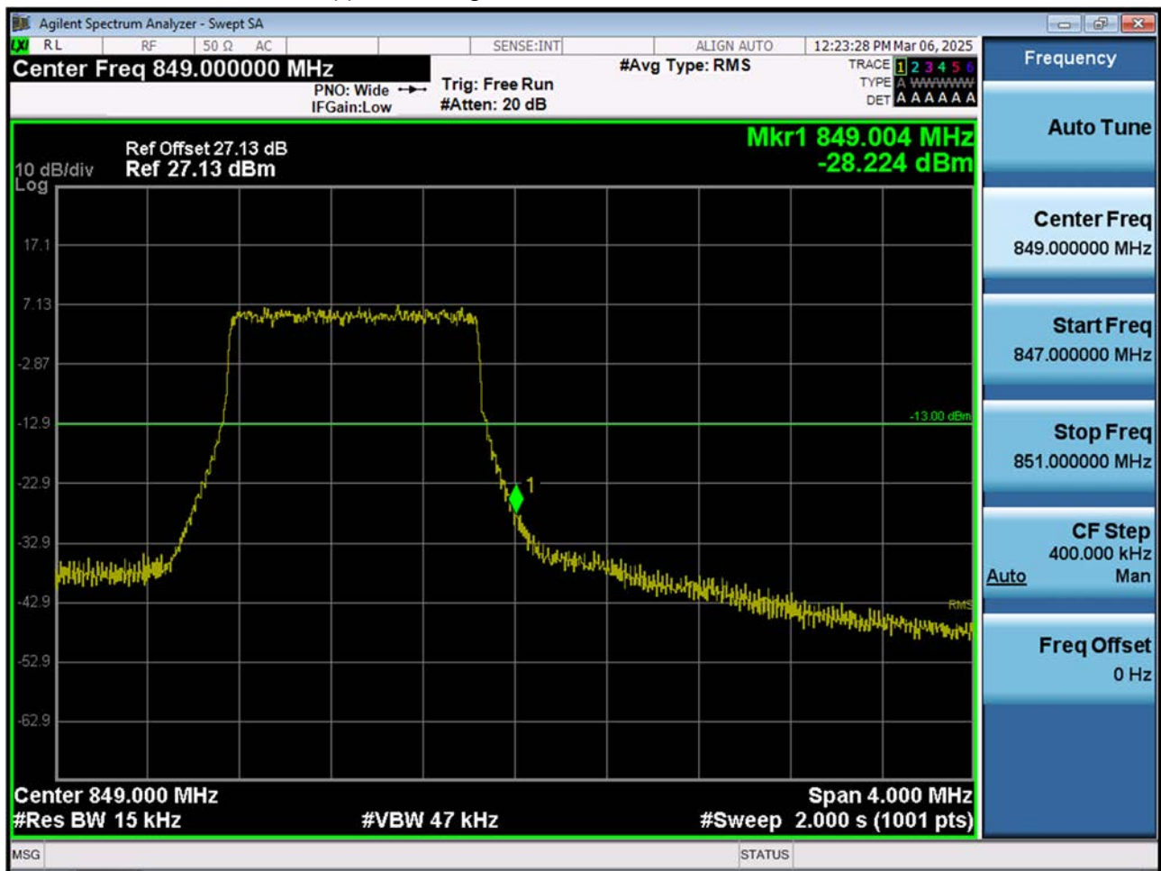
BAND 26. Upper Band Edge Plot (1.4 M BW Ch.27033 QPSK_RB6_Offset 0)
