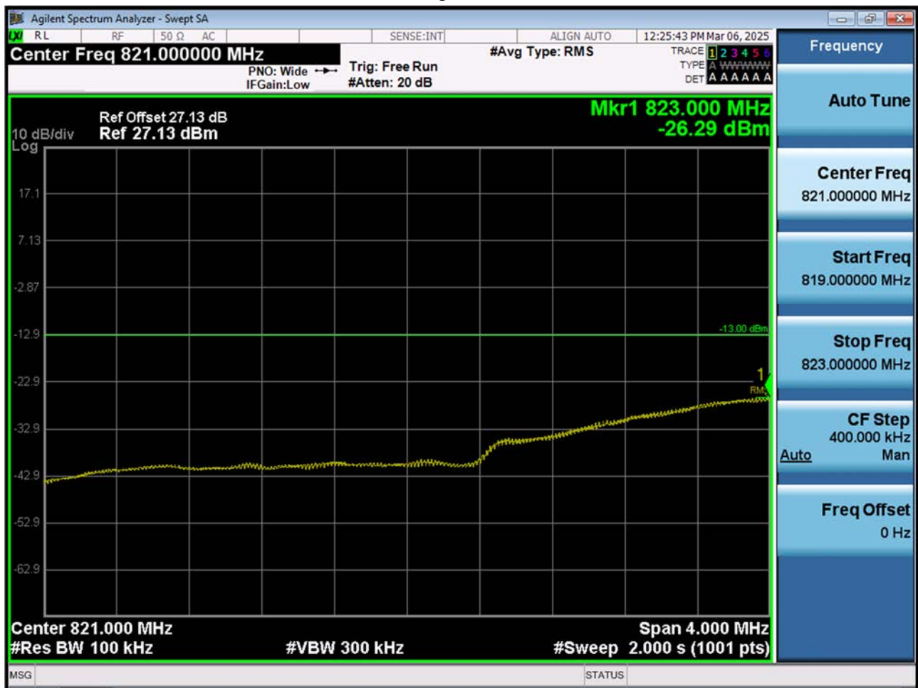
BAND 26. Lower Extended Band Edge Plot (3 M BW Ch.26805 QPSK_RB15_0)
